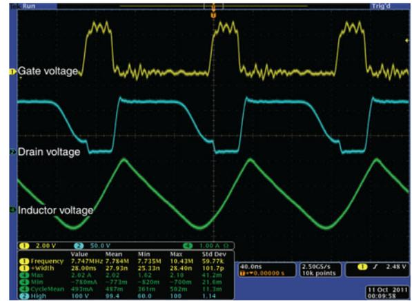
Fig. 5. Waveforms for a prototype HF magnetic stage operating at a frequency of approximately 7.8 MHz from an input voltage of 100 V. Top: gate voltage (2 V/div); middle: drain voltage (50 V/div); bottom: inductor current (1 A/div); horiz: 40 ns/div. At the top end of the input voltage range, the HF stage loses true zero-voltage turn on, but switch turn on is at a sufficiently low voltage that the efficiency remains high.
