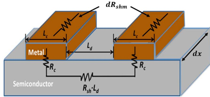
$$R_{||} = \frac{R_{TLM}}{L_{Tx}} \operatorname{csch}\left(\frac{W}{L_{Tx}}\right)$$
