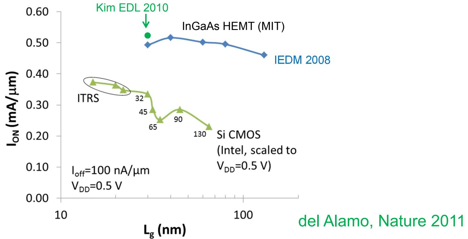
InGaAs HEMTs: higher  $I_{ON}$  for same  $I_{OFF}$  than Si
