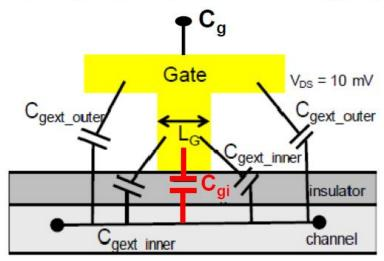
$$C_{g} = C_{gi} \times L_{g} + 2C_{gext\_inner} + 2C_{gext\_outer} \times C_{g} @ OFF$$
