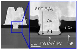
Optimized gate recess with L<sub>side</sub> < 5 nm
