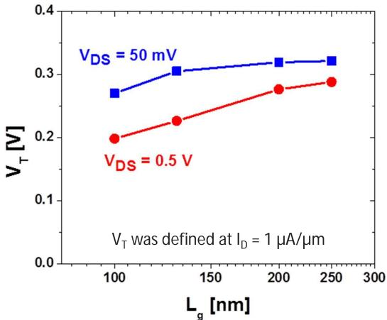
■ V<sub>T</sub> = 0.2 V at L<sub>q</sub> = 100 nm: Enhancement-mode operation
