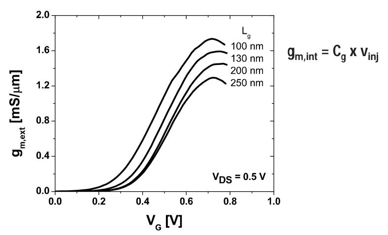
$g_m = 1.73$  mS/ $\mu$ m at  $V_{DS} = 0.5$  V (A record  $g_{m,ext}$  at  $L_g = 100$  nm)
