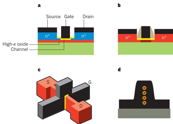
**Figure 4 | Possible future MOSFETs using a III-V compound semiconductor channel.**
