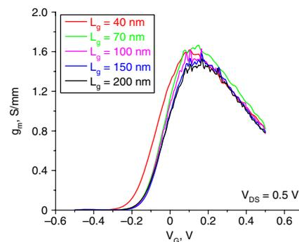
Fig. 3 Transconductance characteristics of HEMTs with various gate lengths from 40 to 200 nm at  $V_{\text{DS}} = 0.5\ \text{V}$
