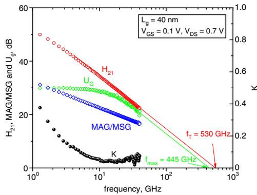
**Fig. 4** Microwave characteristics of 40 nm InGaAs HEMT at  $V_{GS} = 0.1 \text{ V}$  and  $V_{DS} = 0.7 \text{ V}$ . An  $f_T = 530 \text{ GHz}$  and  $f_{max} = 445 \text{ GHz}$  are extracted
