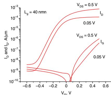
Fig. 2 Subthreshold and gate current characteristics of 40 nm InGaAs HEMT at  $V_{\text{DS}} = 50\ \text{mV}$  and  $V_{\text{DS}} = 0.5\ \text{V}$
