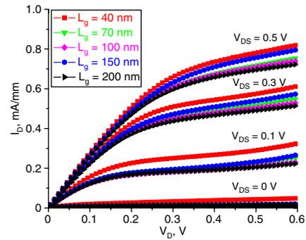
Fig. 1 Output characteristics of fabricated InGaAs HEMTs with various gate lengths
