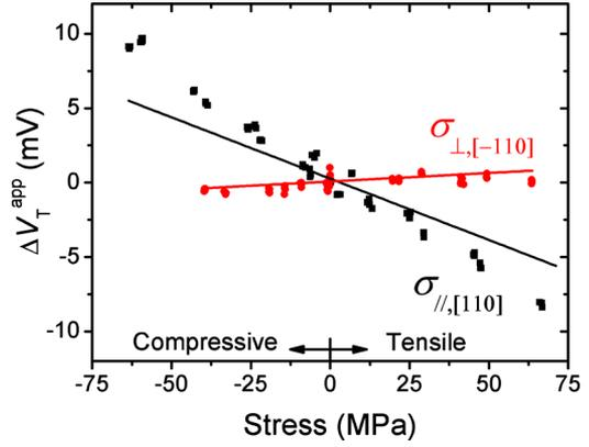
FIG. 3. (Color online) Change of measured or apparent threshold voltage as a function of  $\langle 110 \rangle$  stress. The solid lines represent  $\Delta V_T^{\text{app}}$  projected from  $\Delta \mu_h$  according to Eq. (2).
