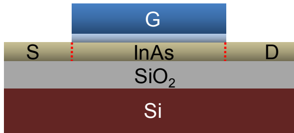
InAs Nanoribbon MOSFETs on Insulator (UC Berkeley) Ko, Nature 2010
