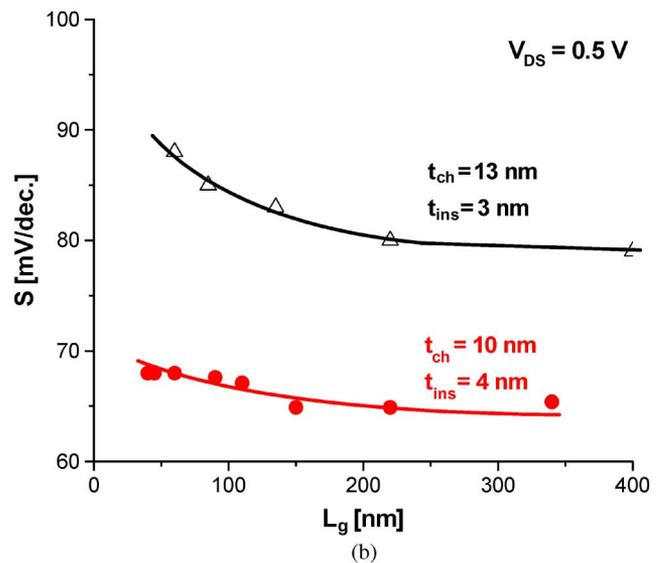
Fig. 10. (a) DIBL and (b) subthreshold swing as a function of  $L_g$ , for InAs HEMTs with  $t_{ins} = 4 \text{ nm}$  and  $t_{ch} = 4 \text{ nm}$ , and  $\text{In}_{0.7}\text{Ga}_{0.3}\text{As}$  HEMTs with  $t_{ins} = 3 \text{ nm}$  and  $t_{ch} = 13 \text{ nm}$ .
