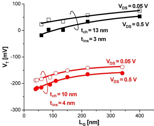
Fig. 9.  $V_T$  roll-off behavior of InAs HEMTs with  $t_{ins} = 4 \text{ nm}$  and  $\text{In}_{0.7}\text{Ga}_{0.3}\text{As}$  HEMTs with  $t_{ins} = 3 \text{ nm}$ .
