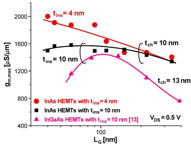
Fig. 6. Maximum transconductance ( $g_{m,\text{max}}$ ) as a function of  $L_g$  for InAs HEMTs with  $t_{\text{ins}} = 10$  nm (black) and  $t_{\text{ins}} = 4$  nm (red). Our previous results on  $\text{In}_{0.7}\text{Ga}_{0.3}\text{As}$  HEMTs with  $t_{\text{ins}} = 10$  nm and  $t_{\text{ch}} = 13$  nm are also included [13]. For all data,  $V_{DS}$  is 0.5 V.
