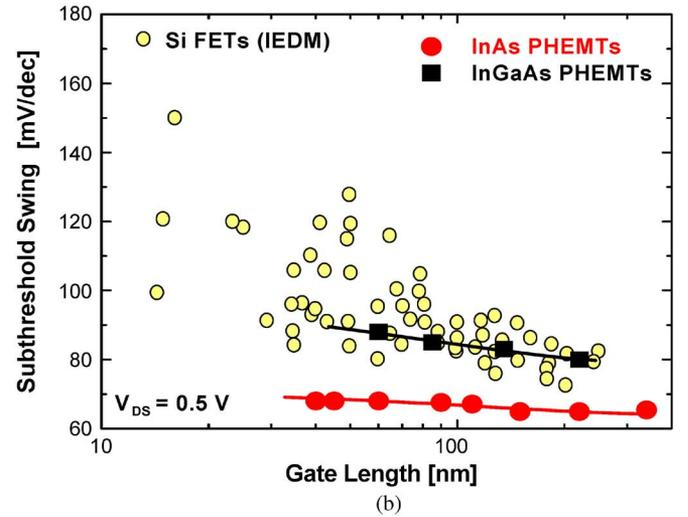
Fig. 13. (a) DIBL and (b) subthreshold swing of InAs HEMTs with  $t_{ins} = 4$  nm and  $t_{ch} = 4$  nm, and  $In_{0.7}Ga_{0.3}As$  HEMTs with  $t_{ins} = 3$  nm and  $t_{ch} = 13$  nm against  $L_g$ , together with that of advanced Si MOSFETs.
