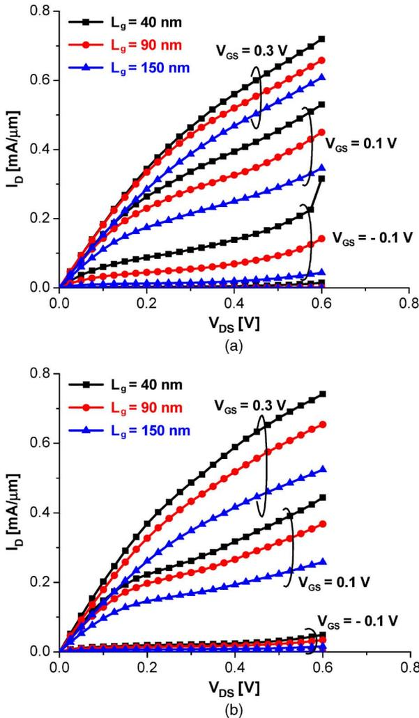
Fig. 3. Output characteristics of InAs HEMTs with (a)  $t_{ins} = 10$  nm and (b)  $t_{ins} = 4$  nm for various values of  $L_g$ .
