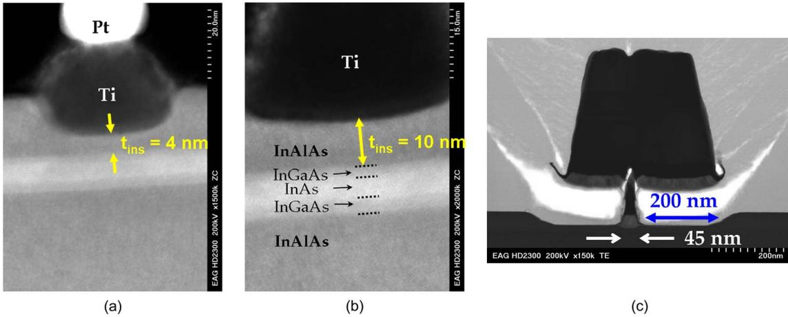
Fig. 2. STEM images of the cross section of the fabricated device. (a) Close up of gate region for an  $L_g = 40$  nm and  $t_{ins} = 4$  nm device. (b) Close up of gate region for  $t_{ins} = 10$  nm device with  $L_g = 45$  nm. (c) Gate view of an  $L_g = 45$  nm gate length device showing  $L_{side} = 200$  nm.
