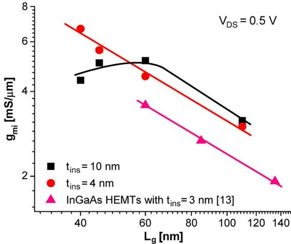
Fig. 8. Extracted intrinsic transconductance ( $g_{mi}$ ) as a function of  $L_g$  for InAs HEMTs with  $t_{ins} = 4 \text{ nm}$  and  $10 \text{ nm}$ , and  $\text{In}_{0.7}\text{Ga}_{0.3}\text{As}$  HEMTs with  $t_{ins} = 3 \text{ nm}$ , at  $V_{DS} = 0.5 \text{ V}$ .
