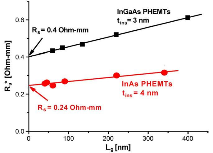
Fig. 7. Measured  $R_s^*$  as extracted by the gate current injection technique as a function of  $L_g$  for InAs HEMTs with  $t_{\text{ins}} = 4$  nm and  $\text{In}_{0.7}\text{Ga}_{0.3}\text{As}$  HEMTs with  $t_{\text{ins}} = 3$  nm. The extracted values of  $R_s$  for both devices are shown.
