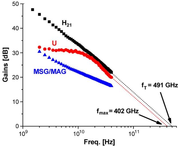
Fig. 12.  $H_{21}$ ,  $U$ , and  $MSG/MAG$  of 40-nm InAs HEMTs at  $V_{GS} = 0$  V and  $V_{DS} = 0.5$  V.
