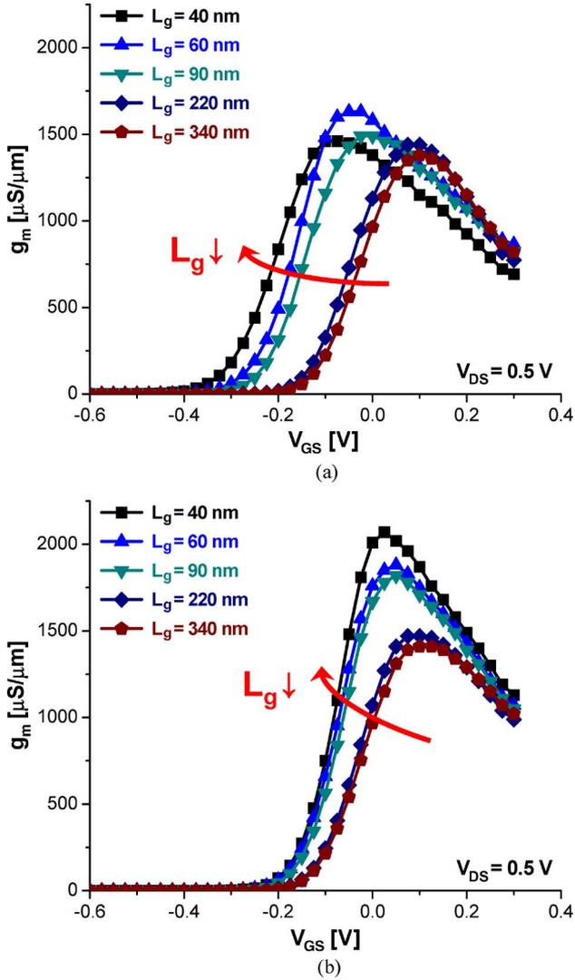
Fig. 5. Transconductance characteristics of 40-nm InAs HEMTs with (a)  $t_{\text{ins}} = 10$  nm and (b)  $t_{\text{ins}} = 4$  nm, for various values of  $L_g$ , at  $V_{DS} = 0.5$  V.
