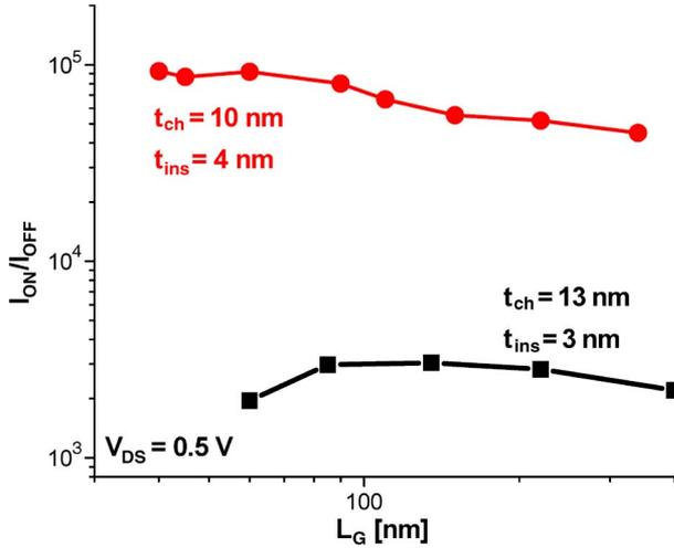
Fig. 11.  $I_{ON}/I_{OFF}$  as a function of  $L_g$ , for InAs HEMTs with  $t_{ins} = 4$  nm and  $t_{ch} = 4$  nm, and  $In_{0.7}Ga_{0.3}As$  HEMTs with  $t_{ins} = 3$  nm and  $t_{ch} = 13$  nm.
