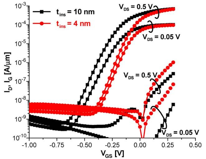
Fig. 4. Subthreshold and gate current characteristics of 40-nm InAs HEMTs with  $t_{ins} = 10$  nm (black) and  $t_{ins} = 4$  nm (red), at  $V_{DS} = 0.05$  V and 0.5 V.
