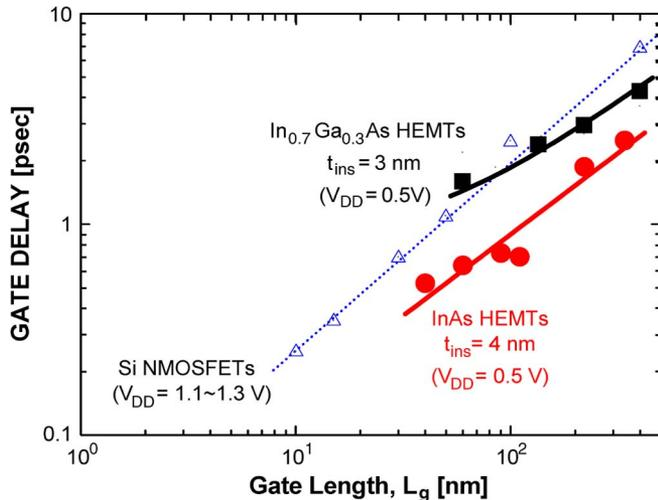
Fig. 14. Gate delay (CV/I) of InAs HEMTs with  $t_{\text{ins}} = 4$  nm and  $t_{\text{ch}} = 4$  nm, and  $\text{In}_{0.7}\text{Ga}_{0.3}\text{As}$  HEMTs with  $t_{\text{ins}} = 3$  nm and  $t_{\text{ch}} = 13$  nm at  $V_{DD} = 0.5$  V, together with that of advanced Si MOSFETs at  $V_{DD} = 1.1$  V to 1.3 V.
