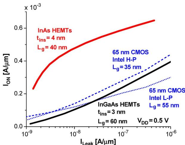
Fig. 15.  $I_{\text{ON}}$  versus  $I_{\text{Leak}}$  of 40-nm InAs HEMTs with  $t_{\text{ins}} = 4$  nm and 60-nm  $\text{In}_{0.7}\text{Ga}_{0.3}\text{As}$  HEMTs with  $t_{\text{ins}} = 3$  nm, together with both high-performance and low-power 65-nm CMOS, at  $V_{DD} = 0.5$  V.
