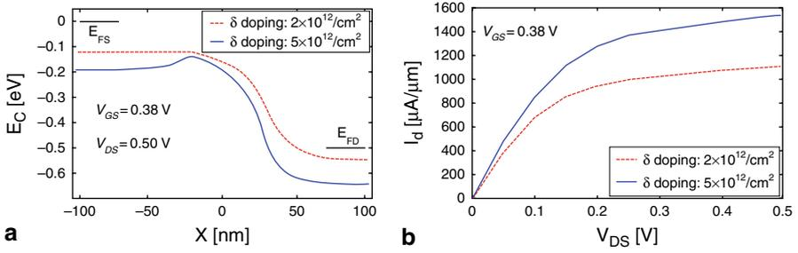
**Fig. 3.8** **a** The first subband profile of the HEMT transistor indicates that the potential barrier of the low doping HEMT vanishes at smaller gate bias than the high doping HEMT. **b** The  $I_d$ - $V_{DS}$  plot shows low delta-doping HEMT has smaller current than the one with higher delta doping at the same gate bias
