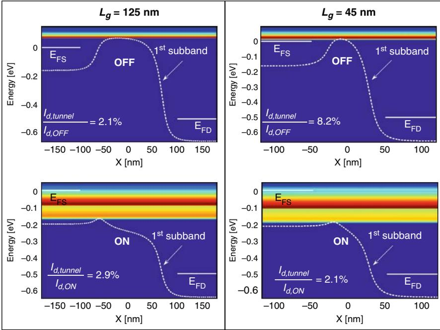
**Fig. 3.9** The S/D tunneling is illustrated by the energy-resolved current density in the short and long gate length HEMTs at off and on states. The S/D tunneling effect is larger in shorter HEMTs at off state due to short gate length and larger DIBL
