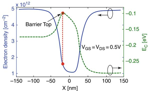
**Fig. 3.5** The sheet charge density at the virtual source is determined from the spatial sheet charge density at the top of the potential barrier
