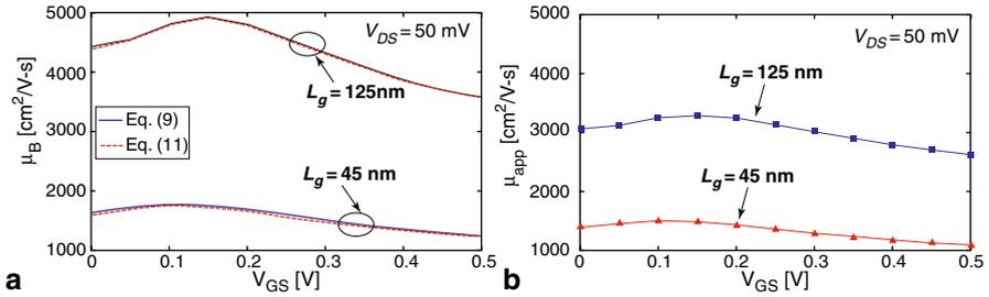
**Fig. 3.7** **a** The ballistic mobilities  $\mu_B$  determined from Eqs. (3.9) and (3.11) are almost identical for 45 nm and 125 nm HEMTs respectively. **b** The apparent channel mobility  $\mu_{app}$  is gate length dependent and significantly degraded from the bulk mobility  $\mu_0 (= 10,000\text{ cm}^2/\text{V}\cdot\text{s})$  due to the small  $\mu_B$ . The series resistance is  $R_S = R_D = 220\ \Omega\ \mu\text{m}$
