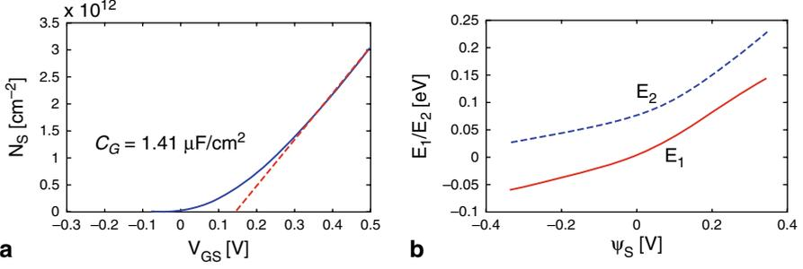
**Fig. 3.4** **a** The charge density in the quantum well gives  $C_G = 1.41 \mu\text{F}/\text{cm}^2$  at  $V_{GS} = 0.5\text{V}$ . **b** The 1st and 2nd subband energy as a function of the surface potential of the quantum well
