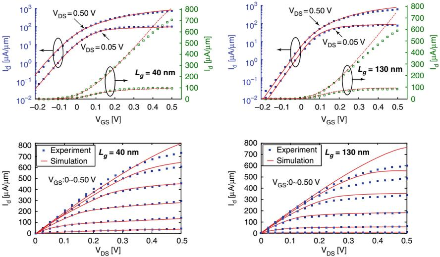
**Fig. 3.2** Comparison of the  $I$ - $V$  characteristics between experimental (*square symbols*) and simulation results (*solid and dash lines*) for 40 nm (*left*) and 130 nm (*right*) HEMTs shows quantitative good agreement by adjusting the gate length and insulator thickness in a reasonable range
