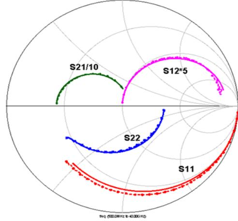
Fig. 3: Measured and Modeled s-parameters at  $V_{DD}=1$  V,  $I_D=100$  mA/mm. Measured data is in symbols and the model is the solid line.  $W=2 \times 48$   $\mu\text{m}$ .
