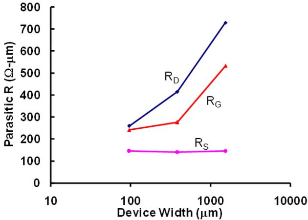
Fig. 6: Normalized parasitic resistances vs. device width. Parasitic resistances are extracted from s-parameters measured at  $V_{DD}=1$  V,  $I_D=100$  mA/mm.
