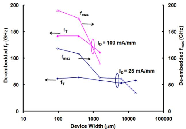
Fig. 1: De-embedded  $f_T$  and  $f_{max}$ , measured at  $I_D=25$  mA/mm and at  $I_D=100$  mA/mm, as a function of total device width
