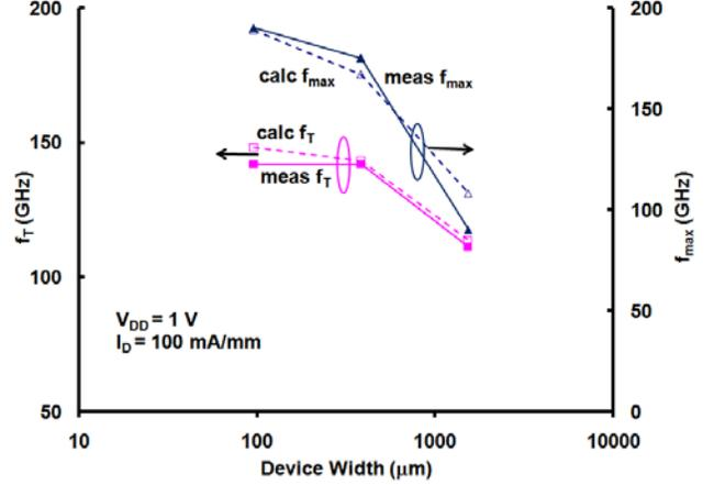
Fig. 7: Measured and calculated  $f_T$  and  $f_{\max}$  as a function of device width. Measured data in solid symbols and lines and calculated data in open symbols and dashed lines.
