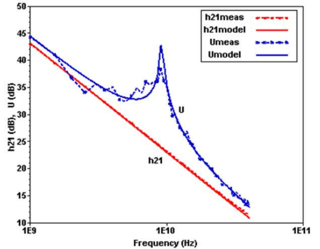
Fig. 4: Short circuit current gain and unilateral power gain as a function of frequency.  $W=2 \times 48$   $\mu\text{m}$ ,  $V_{DD}=1$  V,  $I_D=100$  mA/mm
