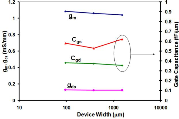
Fig. 5: Normalized intrinsic parameters ( $g_m$ ,  $g_{ds}$ ,  $C_{gs}$ ,  $C_{gd}$ ) as a function of device width.  $V_{DD}=1$  V,  $I_D=100$  mA/mm.
