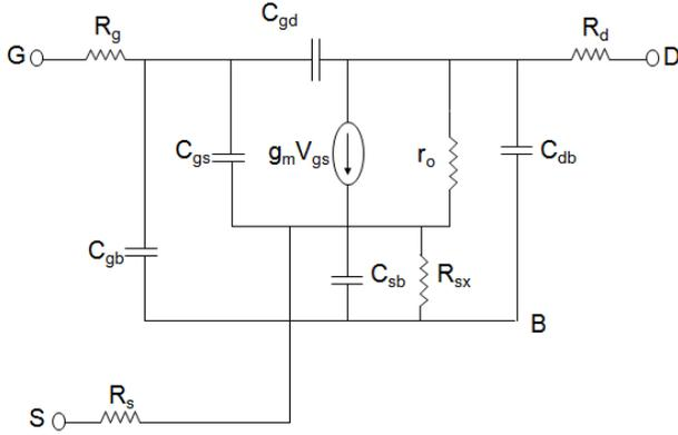
Fig. 2: Small-signal equivalent circuit of a MOSFET including parasitic resistances and the substrate network.
