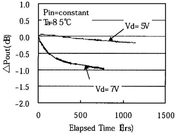
Figure 2. Pout degradation under RF life test for  $V_d$  of 5 V and 7 V. Samples are in hermetic packaging.
