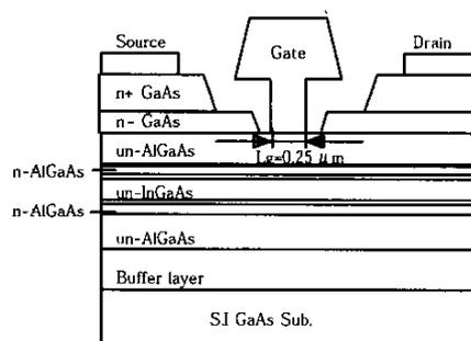
Figure 1. Cross section of AlGaAs/InGaAs PHEMT.
