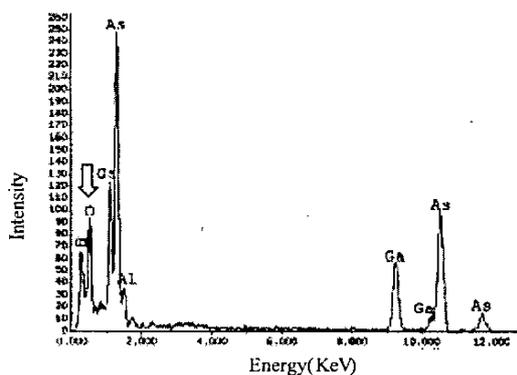
Figure 7. EDX spectra of degraded region.
