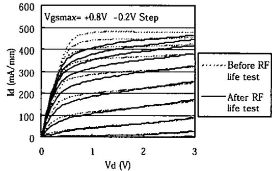
Figure 5. DC characteristics change after RF life test ( $T_{ch}=150^\circ\text{C}$ ,  $V_d=5\text{ V}$ , 2000 hrs).
