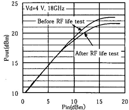
Figure 4. Power characteristics change after RF life test ( $T_{ch}=150^\circ\text{C}$ ,  $V_d=5\text{ V}$ , 2000hrs).
