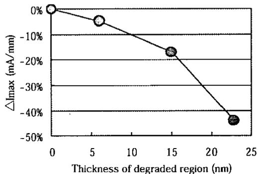
Figure 8.  $I_{max}$  change during RF life test as a function of thickness of degraded region.
