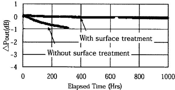
Figure 11. Pout change during RF life test (T<sub>ch</sub>=175°C, V<sub>d</sub>=5 V) of samples with and without surface treatment.
