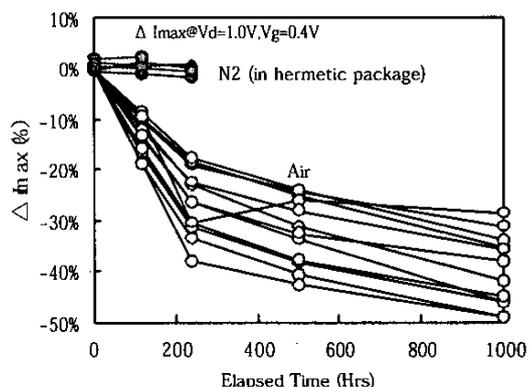
Figure 9.  $I_{max}$  change during DC life test in hermetic package and in air ( $T_{ch}=150^{\circ}\text{C}$ ,  $V_d=4\text{V}$ ,  $I_d=150\text{mA/mm}$ ).
