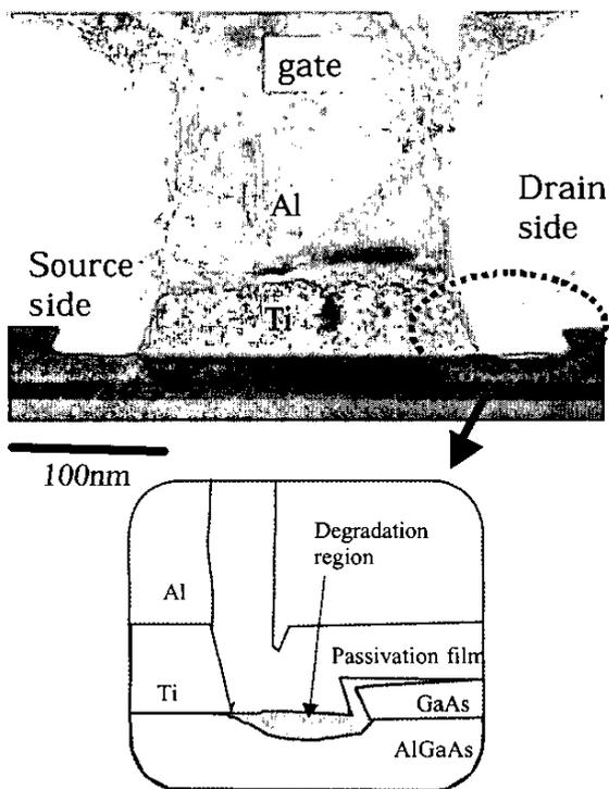
Figure 6. TEM photograph of a degraded device under RF life test.
