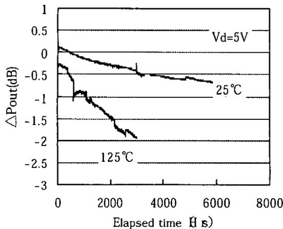
Figure 3. Pout degradation under RF life test at ambient temperature of 25°C and 125°C. Samples are in hermetic packaging.
