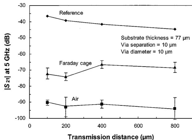
Fig. 4. Average  $|S_{21}|$  at 5 GHz versus the transmitter–receiver distance for Faraday cage and reference structures. The error bars indicate one standard deviation away from the mean. The effectiveness of the Faraday cage is relatively constant with increasing transmission distance. The air measurements are well below the Faraday cage, indicating that the measurements are not limited by air crosstalk.
