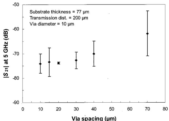
Fig. 5. Average  $|S_{21}|$  versus via spacing of the Faraday cage at 5 GHz. No crosstalk dependence is apparent up to a  $30\text{-}\mu\text{m}$  separation. There is slight degradation for larger via spacings.
