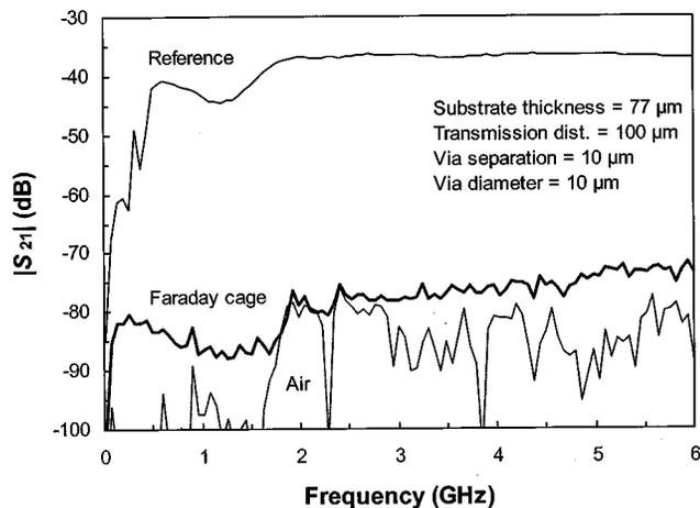
Fig. 3.  $|S_{21}|$  versus frequency for a Faraday cage and reference structure at a transmission distance of  $100 \mu\text{m}$ . This Faraday cage provides 38 dB of isolation at 5 GHz and 43 dB at 1 GHz. Also plotted is  $|S_{21}|$  of the probes in the air.
