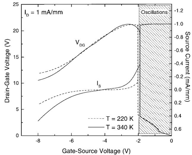
Fig. 6. Drain current injection results at high and low temperature for  $I_D = 1$  mA/mm. The drop in  $BV_{DG}$  appears virtually independent of temperature.
