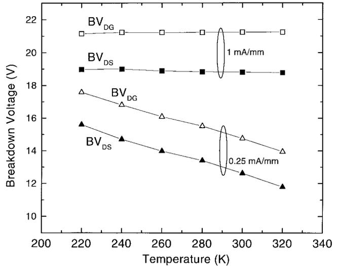
Fig. 4. Temperature dependence of breakdown at  $I_D = 0.25$  mA/mm and  $I_D = 1$  mA/mm. Note that  $BV_{DG}$  and  $BV_{DS}$  track each other, and that the temperature dependence of breakdown is negative at low current criteria, and approximately zero at higher current criteria.
