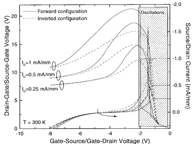
Fig. 7. Drain current injection results for pHEMT in normal and inverted configuration. The device's asymmetry is reflected by the fact that the source-gate voltage drops less than the drain-gate voltage for the same current criteria. Note that at sufficiently negative gate voltages, the asymmetry disappears.
