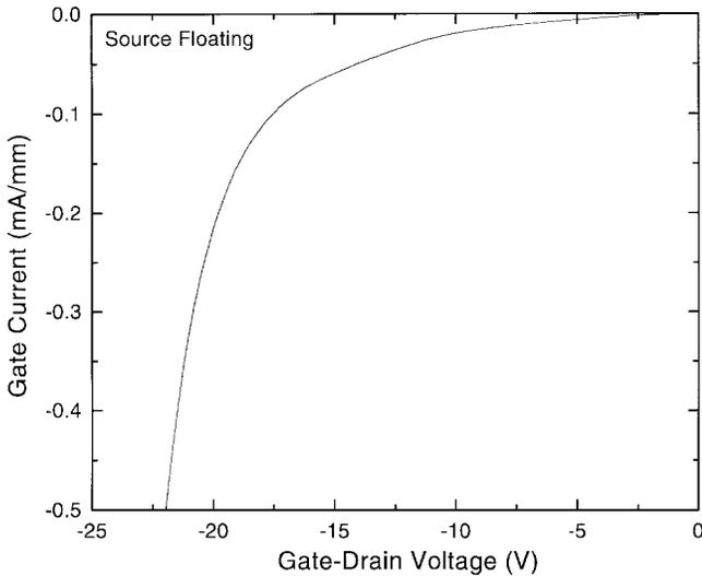
Fig. 2. Reverse gate-drain current-voltage characteristics measured with the source floating at room temperature.
