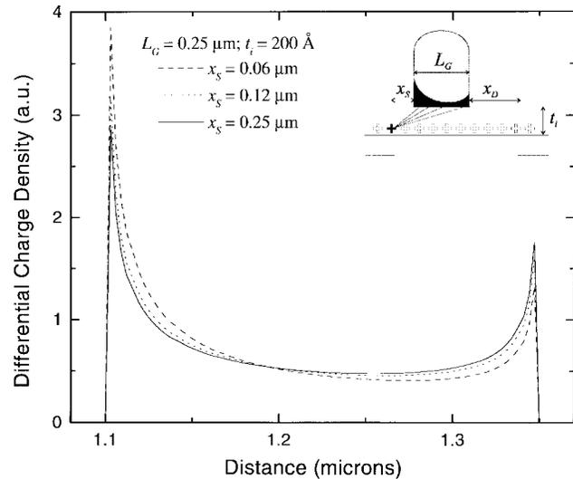
Fig. 8. Magnitude of calculated surface charge density on a finite gate due to a single line charge for three different charge positions, as indicated in the inset. Note that although the line charges are located in the gate-source gap, the conformal transform predicts that the corresponding image charges spread across the entire gate length, and are strongly peaked at *both* ends of the gate.
