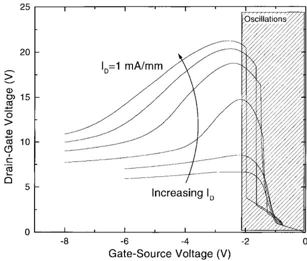
Fig. 5. Drain current injection results at room temperature for several current criteria ( $I_D = 0.02, 0.05, 0.25, 0.5, 0.75,$  and  $1.0$  mA/mm) for power pHEMT. The pHEMT exhibits classical drain-gate breakdown behavior at low current criteria ( $I_D < 0.1$  mA/mm), but for higher current criteria,  $BV_{DG}$  drops significantly as  $V_{GS}$  is reduced.
