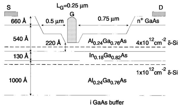
Fig. 1. Schematic cross section of AlGaAs/InGaAs double-heterostructure pHEMT used in this work.
