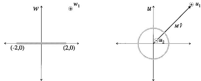
Fig. 13. Finite gate conformal transformation. The image charge necessary to create the equipotential surface is shown in the transformed coordinate system.
