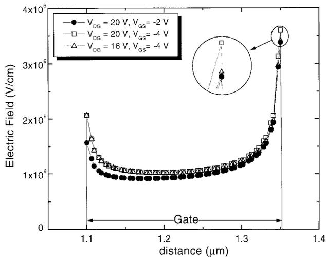
Fig. 11. MEDICI simulations of electric field beneath the gate for three bias conditions. Breakdown is associated with the peak field at the drain end of the gate; as  $V_{GS}$  is made more negative,  $V_{DG}$  must be reduced in order to keep the peak drain field constant.
