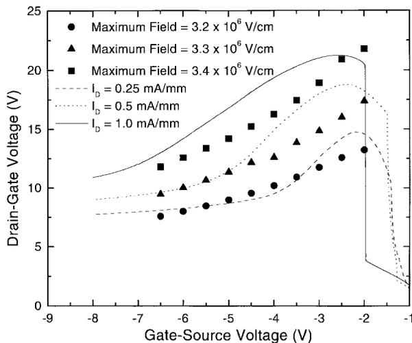
Fig. 12. Comparison of constant current criteria measurements with constant field criteria MEDICI simulations. The simulations effectively capture the qualitative behavior of  $BV_{DG}$ .
