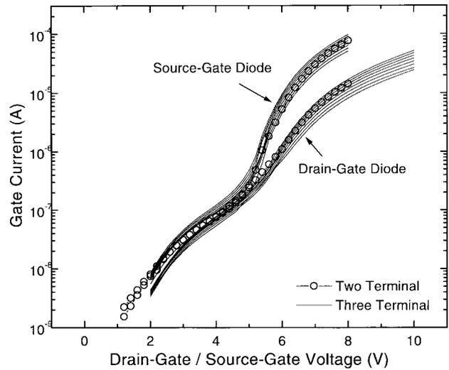
Fig. 3. Comparison of two- and three-terminal measurements of the drain-gate and source-gate diodes. The multiple three-terminal measurements were performed with the gate biased at different voltages slightly below threshold. The asymmetry of the device is apparent.
