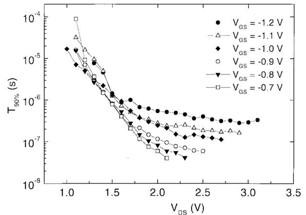
Fig. 3.  $T_{90\%}$ , the time it takes for the kink to reach 90% of its final DC value, as a function of  $V_{DS}$  for different values of  $V_{GS}$ .
