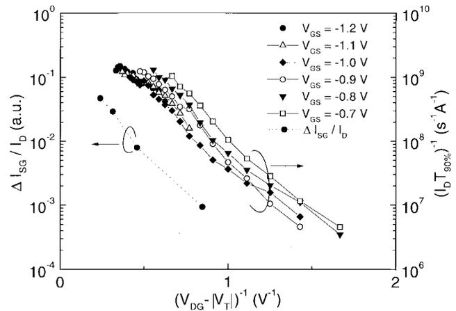
Fig. 4.  $1/(I_D \times T_{90\%})$  and  $\Delta I_{SG}/I_D$  as a function of  $(V_{DG} - |V_T|)^{-1}$ .  $1/T_{90\%}$ , just as the sidegate current, follows a classical impact ionization behavior.
