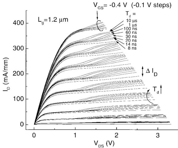
Fig. 1. Pulsed  $I$ - $V$  curves for varying delay times,  $T_d$ . No kink is seen below  $T_d = 10$  ns. For a given  $V_{GS}$ , the larger  $V_{DS}$ , the earlier the kink turns on and the faster it saturates.
