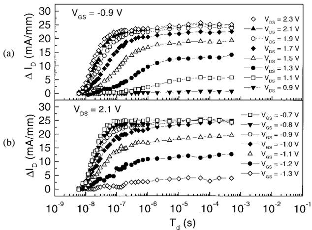
Fig. 2.  $\Delta I_D$  as a function of  $T_d$  in a semilog scale. (a) Constant  $V_{GS}$  ( $V_{GS} = -0.9$  V) and varying  $V_{DS}$ . (b) Constant  $V_{DS}$  ( $V_{DS} = 2.1$  V) and varying  $V_{GS}$ .
