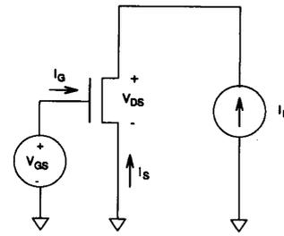
Fig. 1. Schematic circuit diagram for *Drain-current Injection* technique.
