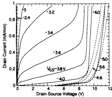
Fig. 3. The output  $I$ - $V$  characteristics on the NE-9000 GaAs MESFET till  $I_D = 1$  mA/mm for  $V_{GS}$  from  $-2.4$  to  $-6$  V. In the drain-gate breakdown regime, the characteristics have been drawn with dashed lines.
