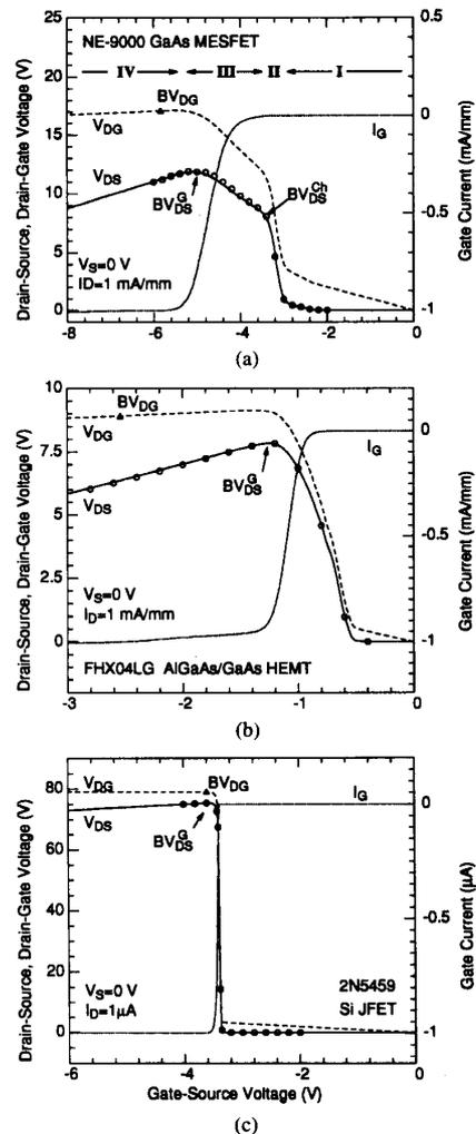
Fig. 2. Illustration of *Drain-current Injection* technique on (a) GaAs MESFET, (b) AlGaAs/GaAs HEMT, and (c) Si JFET. For comparison,  $BV_{DG}$  (triangle) was measured between gate and drain (source floating) at  $I_D = 1 \text{ mA/mm}$ . The circles ( $V_{DS}$ ) were measured from the output  $I$ - $V$  characteristics at  $I_D = 1 \text{ mA/mm}$ . For a discussion of the four regimes marked in Fig. 2(a), see text.
