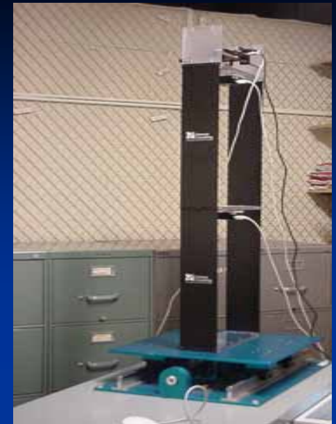
Shake table (Civil Eng., deployed 2004)
