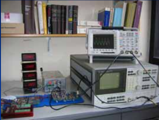
Dynamic signal analyzer (EECS, deployed 2004)
