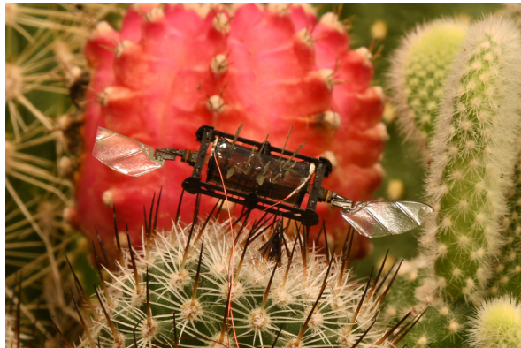
◀ Figure 1: A photograph illustrating a damaged biomimetic robot module that landed on a cactus.
