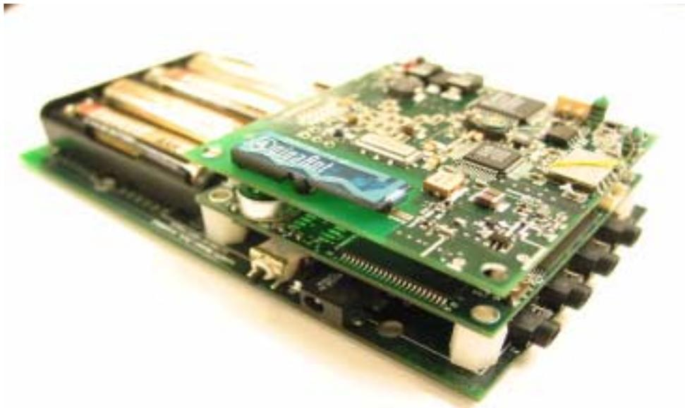
**Figure 1.3:** The current version of the stackable  $\mu$ AMPS node (Courtesy Fred S. Lee)
