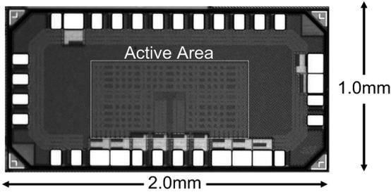
Fig. 12. Die photograph (1.0  $\times$  0.5 mm active area).
