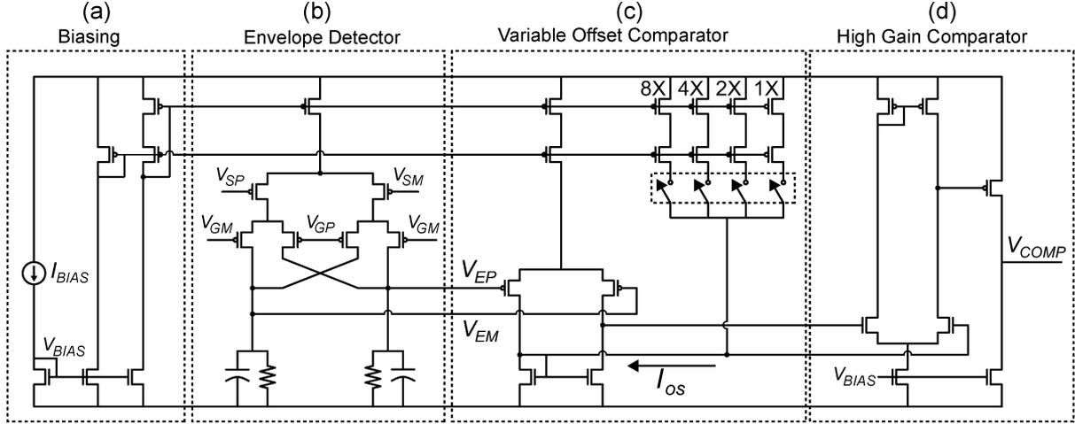
Fig. 10. Schematic for differential envelope detector and comparator with programmable input offset voltage. (a) Biasing; (b) envelope detector; (c) variable offset comparator; (d) high gain comparator.
