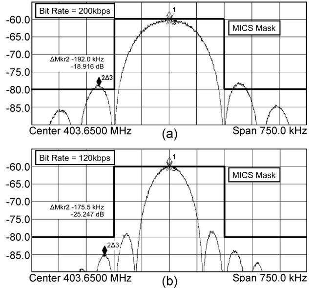
Fig. 14. Measured spectral mask of transmitter with a data rate of (a) 200 kb/s and (b) 120 kb/s. The signal is taken through an antenna 10 cm from the transmitter.
