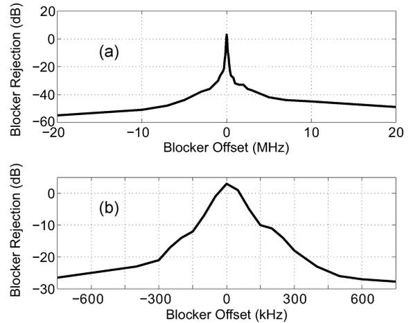
Fig. 17. (a) Far off and (b) close in CW blocker rejection. Input signal level set to sensitivity +6 dB =  $-93 \text{ dBm}$  with a carrier frequency of 403.35 MHz and a bit rate of 40 kb/s.
