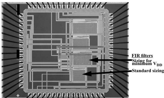
Fig. 16. Annotated die photograph of 0.18- $\mu\text{m}$  subthreshold FIR test chip.
