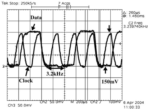
Fig. 11. Oscilloscope plot from the test chip showing  $V_{DD} = 150$  mV filtering operation with ring oscillator clock at 3.2 kHz.
