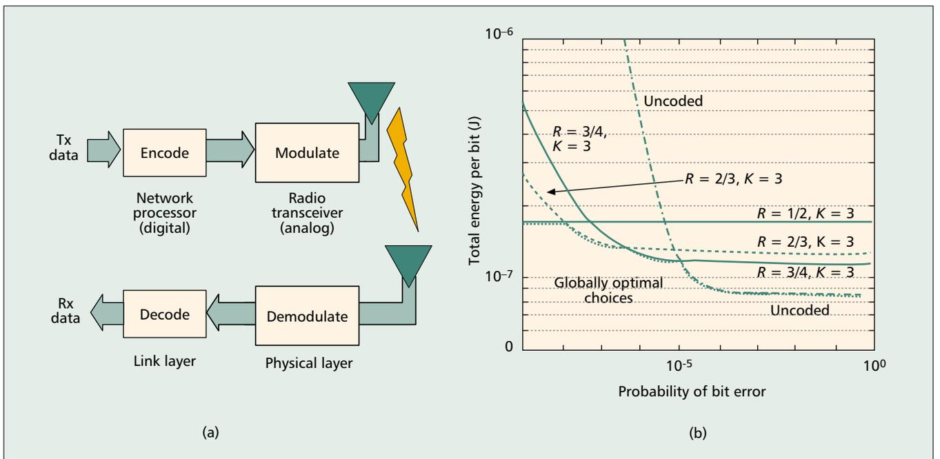
■ Figure 9. a) Energy for communication is dissipated at the network processor, which encodes and decodes the packets, and the analog radio transceiver; b) energy required to transmit 10 kb of data at 1 Mb/s over a 70 dB path loss, with various coding schemes. The globally optimal coding scheme, which is highlighted above, dynamically selects stronger codes as the tolerable bit error decreases.
