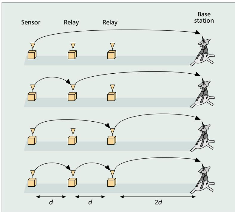
■ Figure 10. In a collinear three-node network, we consider four potential multihop routes from the most distant sensor node to the base station. The minimum energy routing strategy over the lifetime of the network is a temporal rotation among these roles, in a ratio determined by the nodes' energy consumption characteristics.
