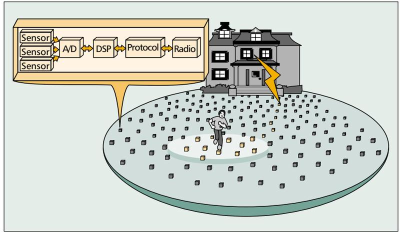
**Figure 1.** The  $\mu$ AMPS microsensor network consists of hundreds to thousands of nodes that collaboratively gather environmental observations (footsteps of the jogger) and forward them to a remote base station (within the house). Individual nodes consist of an array of environmental sensors, A/D conversion, digital signal and network protocol processors, and a radio transceiver for two-way communication.
