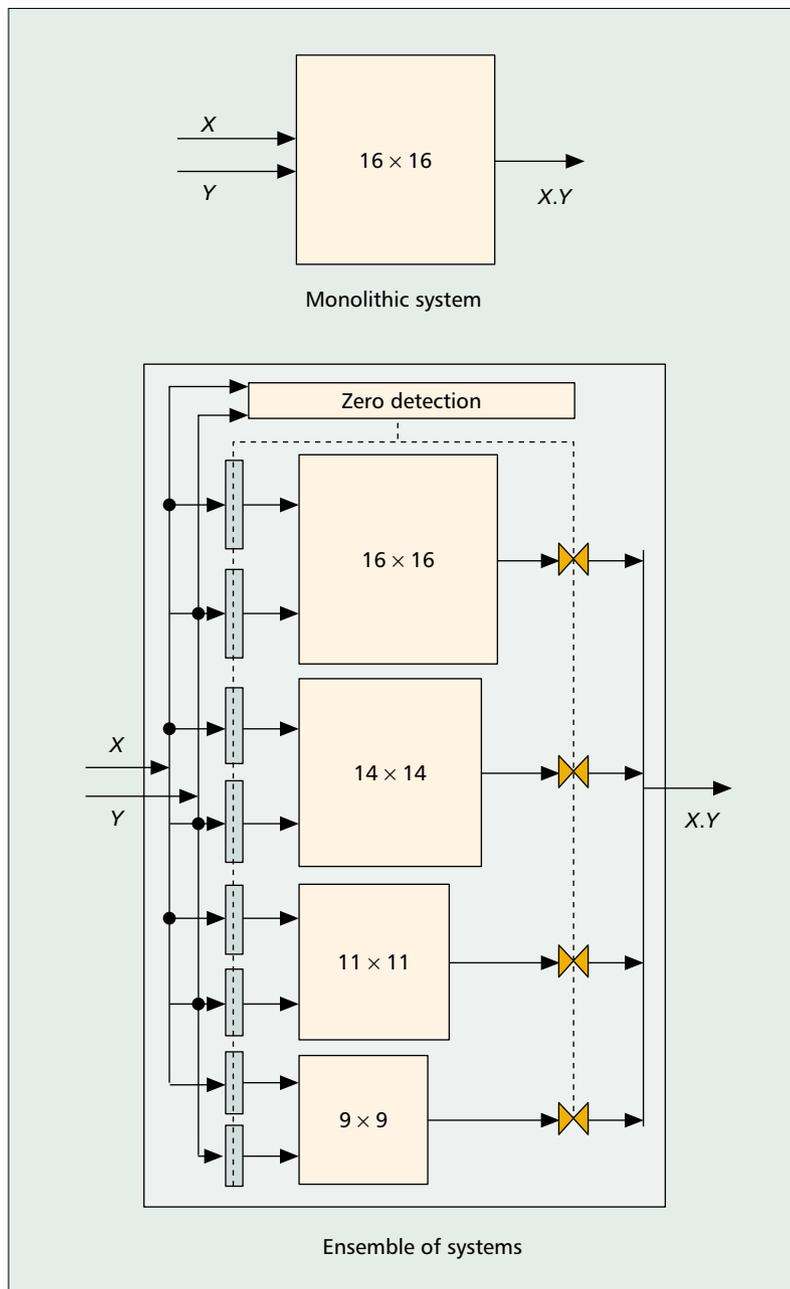
■ Figure 7. A monolithic multiplier (top) is less power-aware than an ensemble of multipliers (below). The ensemble routes each pair of incoming operands to the smallest multiplier that can compute the result to take advantage of the lower energy consumption of the smaller circuit. On a series of operands typical of speech processing applications, the ensemble consumes 57 percent less power than the monolithic multiplier [10].
