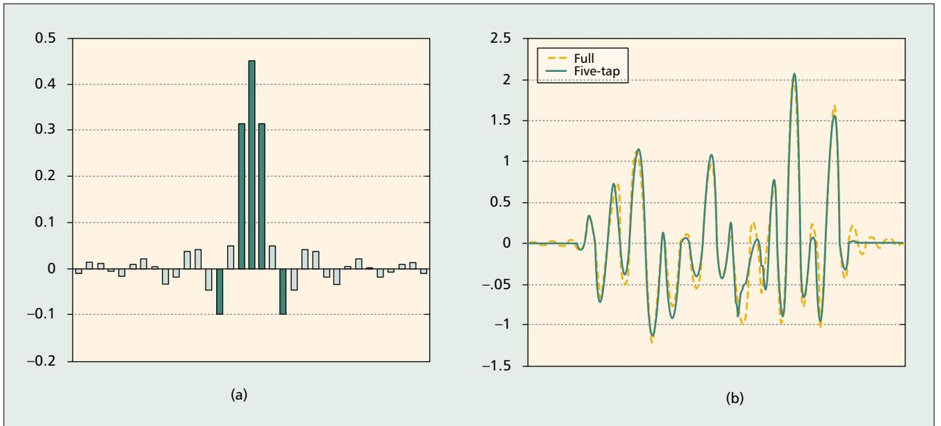
■ Figure 8. a) Finite-impulse response with the five most significant taps highlighted; b) a signal is filtered through both the full FIR filter and an abbreviated filter consisting of the five previously highlighted taps. Even a few of the most significant taps provide a close approximation to the full result.
