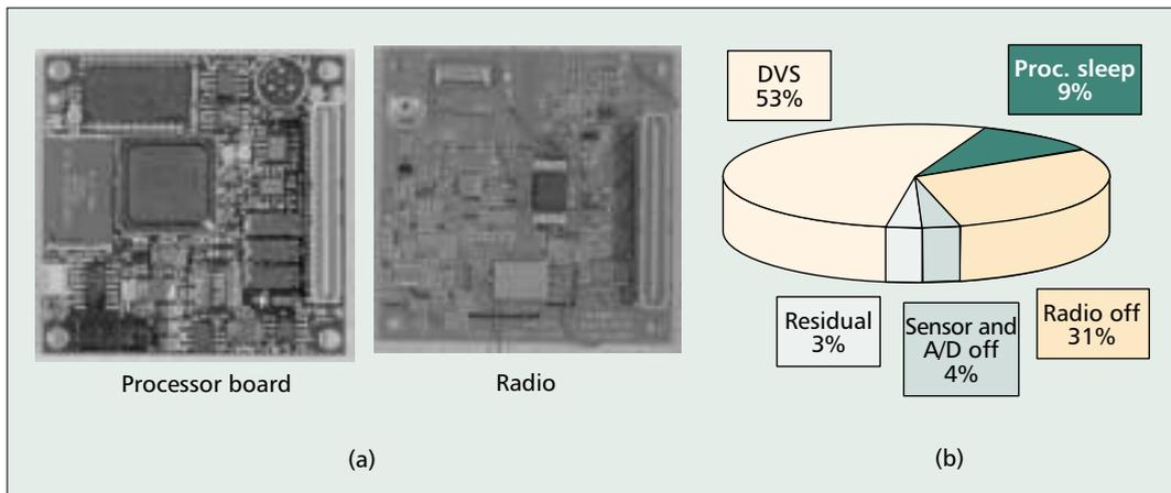
**Figure 2.** a) The  $\mu$ AMPS-1 sensor node is implemented in stackable boards; each board is 55 mm on a side; b) energy-conserving hooks present in  $\mu$ AMPS-1 reduce the peak power of the node by the proportions shown here; power dissipation scales from a minimum of 27 mW to a peak of 976 mW.
