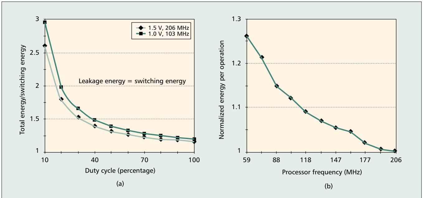
■ Figure 3. a) For low duty cycles, an SA-1100 processor consumes more energy through leakage than active switching; b) running the SA-1100 at lower clock frequencies to compensate for a low duty cycle actually increases the total energy per operation since more leakage energy is dissipated over a longer clock period.
