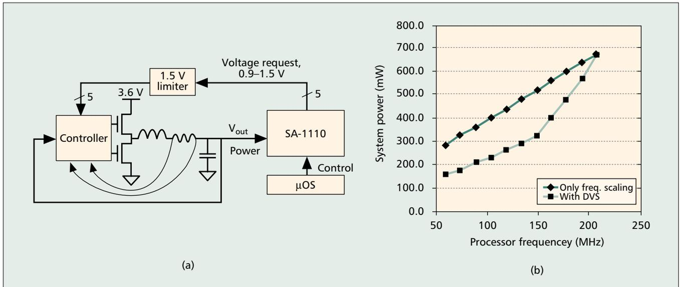
■ Figure 6. a) Dynamic voltage scaling (DVS) support aboard  $\mu$ AMPS-1 — the node operating system running on the SA-1110 monitors workload and latency requirements, and controls the voltage driven by the buck regulator that powers the SA-1110 core; b) DVS on the  $\mu$ AMPS processor alone reduces total node energy by nearly 50 percent. DVS enables a factor-of-four energy scalability on the node.
