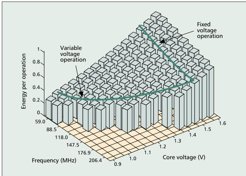
■ Figure 5. Measured energy consumption per operation for the SA-1100 processor, as clock frequency and voltage are varied. A lower frequency at the same voltage incurs a higher per-operation cost due to additional leakage energy.
