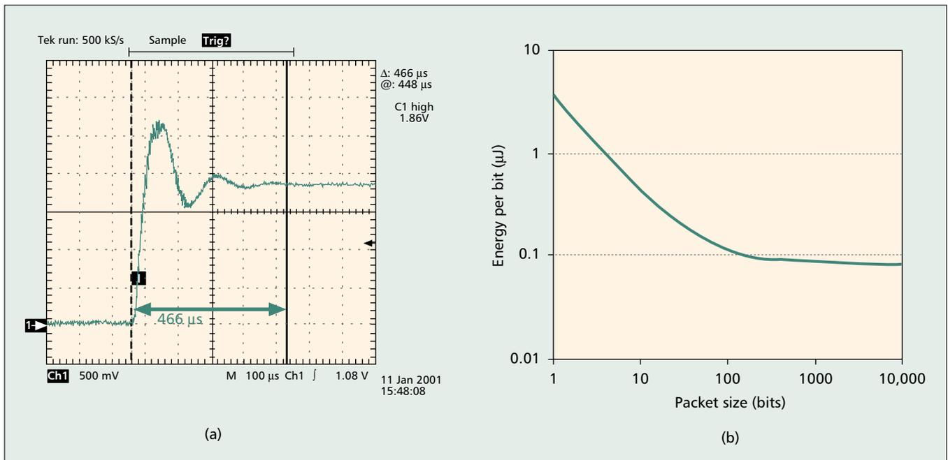
■ Figure 4. a) 466  $\mu\text{s}$  startup transient from the  $\mu\text{AMPS-1}$  2.4 GHz radio, measured at the input to the radio's voltage controlled oscillator; b) the effects of startup energy revealed — the total radio energy per bit required to transmit packets of various sizes. In our model, the data rate is 1 Mb/s, the radio electronics consume 81 mW, and the radiated output power is 1 mW (0 dBm).
