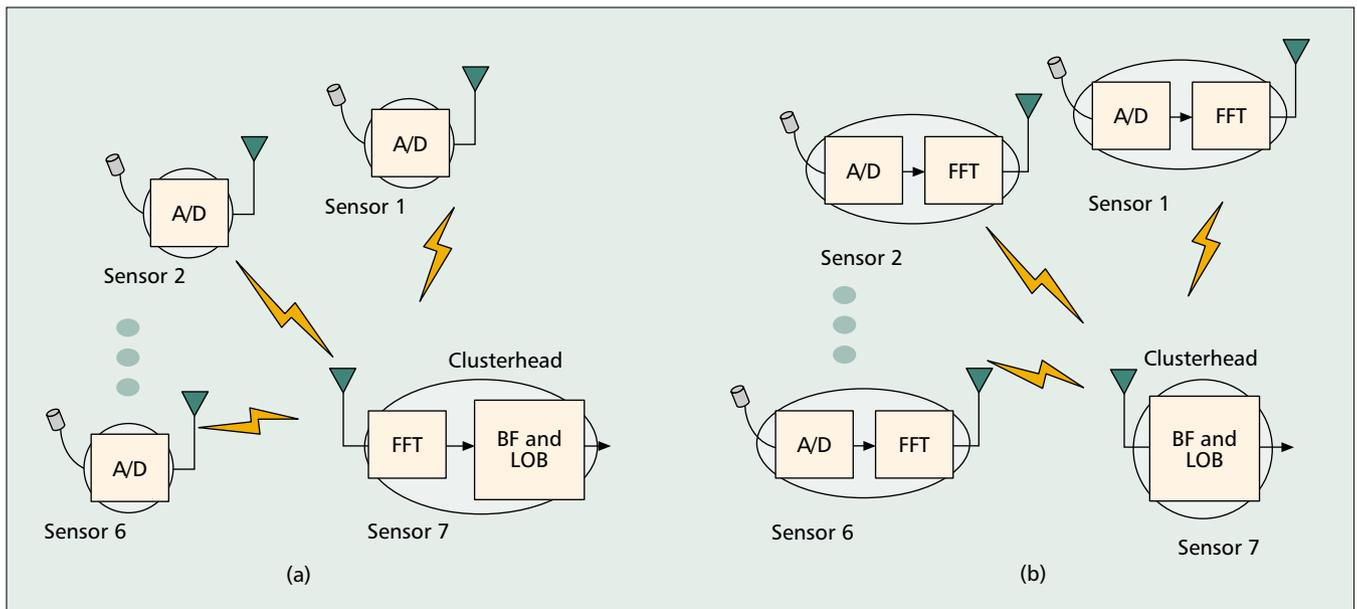
■ Figure 11. Two ways to partition a computation over a cluster of nodes: a) all digital computation (FFT, beamforming, and line-of-bearing detection) is performed at the clusterhead; b) computation is distributed between the clusterhead and observer nodes. The second system partition utilizes the network's inherent parallelism to relax global latency deadlines.
