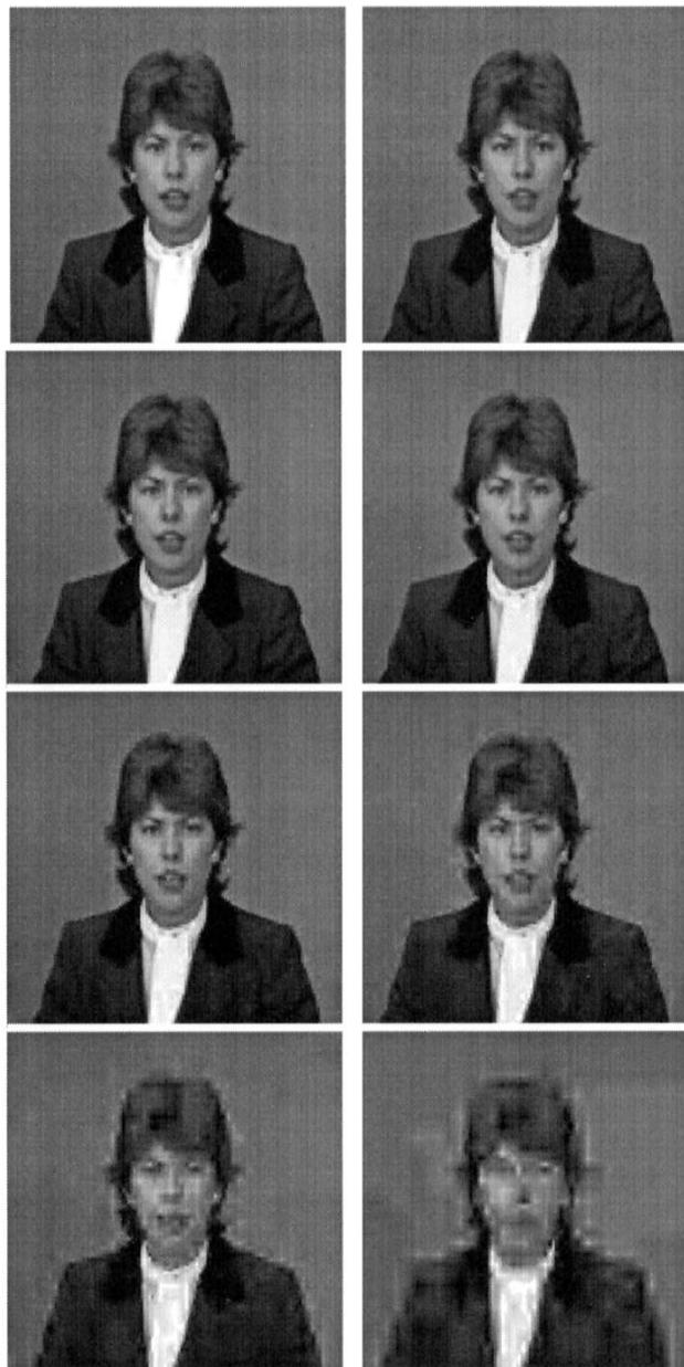
Fig. 2. Compressed frames of head and shoulders sequence. From left to right and top to bottom: original, compress  $\times 7$  (PSNR 44.63),  $\times 12.8$  (PSNR 43.59),  $\times 23.8$  (PSNR 41.36),  $\times 49$  (PSNR 37.89),  $\times 115$  (PSNR 33.77),  $\times 300$  (PSNR 29.85),  $\times 967$  (PSNR 26.17). Compression factors are averages over many frames. PSNR's are for this particular frame, but are indicative for all frames.
