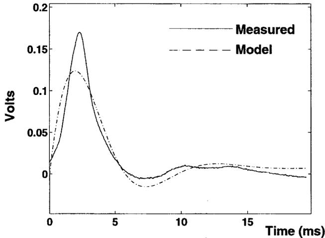
Fig. 5. Measured versus simulated generator response. Mass  $m = 0.5$  g and spring constant  $k = 174$  N/m. The rms error between the simulated and measured response is 15 mV.
