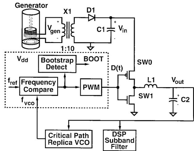
Fig. 9. Detailed block diagram of self-powered DSP system.
