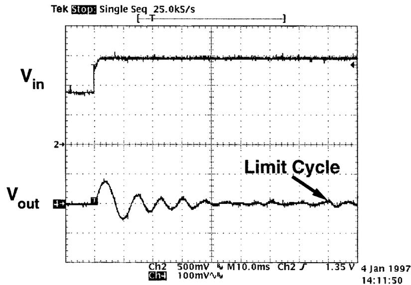
Fig. 15. Step response. Note steady-state limit cycle due to low resolution digital control.
