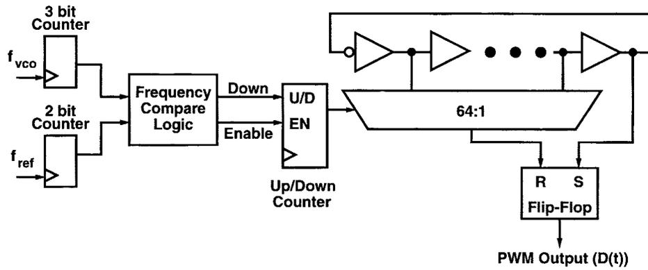
Fig. 11. Low power digital PWM controller architecture.
