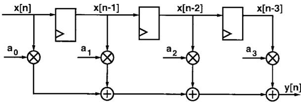
Fig. 10. Subband FIR filter block diagram.
