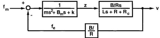
Fig. 4. Block diagram of traditional low-frequency moving-coil transducer model.
