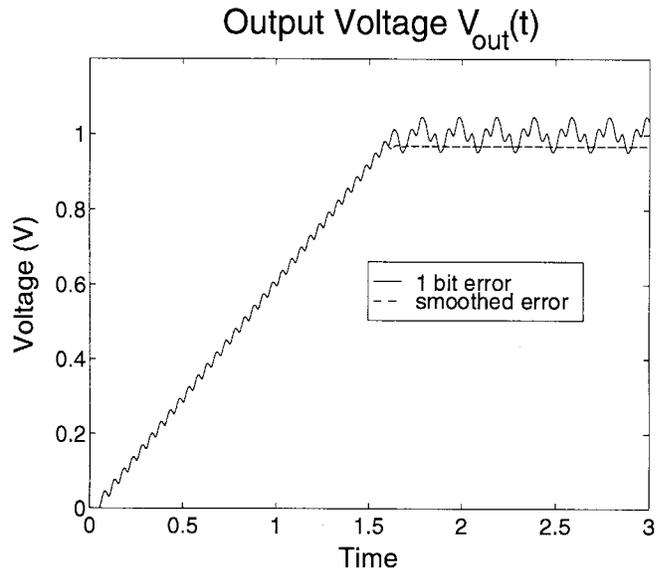
Fig. 13. Limit cycle behavior of low resolution digital control loop. The smoothed error response eliminates the limit cycle, at the cost of steady-state error. The digital duty cycle has 6-bit resolution, for a maximum value of 63.
