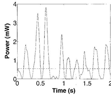
Fig. 8. Stochastic output power simulation: best-case estimate of ambient power generation from vibration due to human walking. Mean output power  $\approx 400 \mu\text{W}$ .
