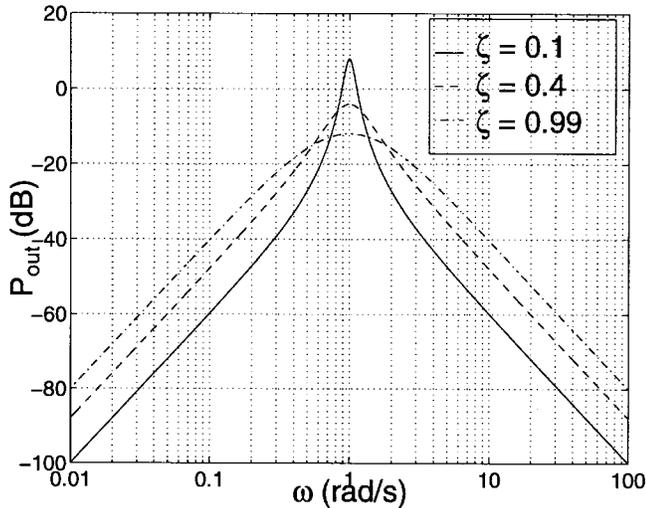
Fig. 7. Frequency domain plot of dc power  $P_{out}$  for three different damping coefficients.
