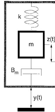
Fig. 6. Simplified generator mechanical dynamics.
