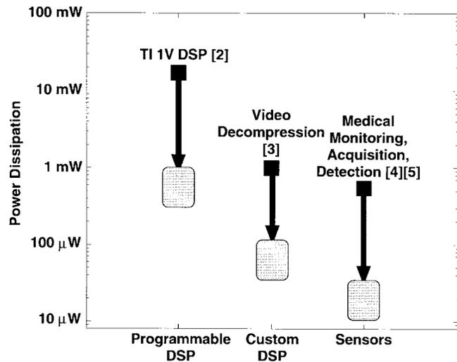
Fig. 1. Trends in power consumption for low to medium throughput DSP.
