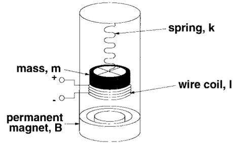
Fig. 3. Generator mechanical schematic.
