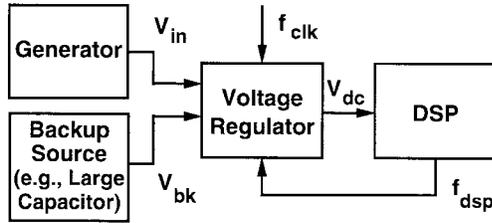
Fig. 2. System block diagram.
