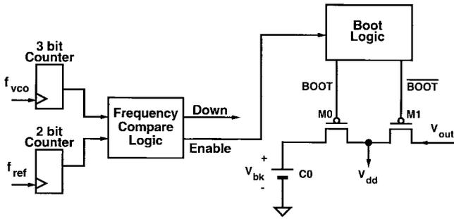
Fig. 14. Bootstrap circuit schematic.
