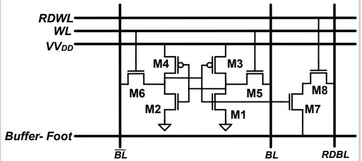
Figure 18.4.2: 8T cell enabling low-voltage read/write and sensing.
