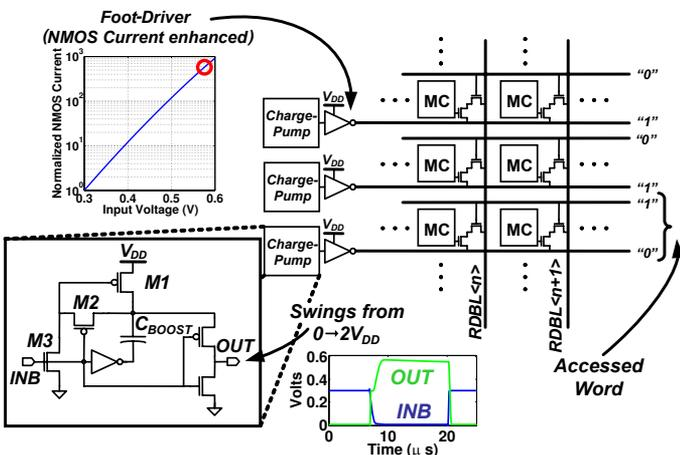
Figure 18.4.3: Circuitry to eliminate sub- $V_{DD}$  leakage from unaccessed read-buffers. Peripheral charge-pumps ensure buffer-foot drivers do not limit  $I_{READ}$ .
