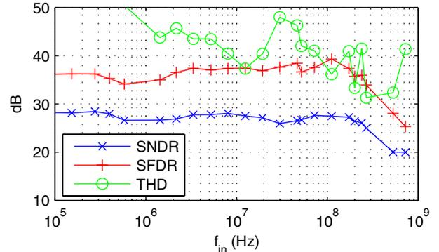
Fig. 4. SNDR and SFDR versus input frequency.
