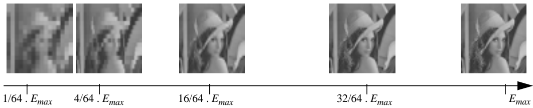
Fig. 8. Illustrating the incremental refinement property with respect to computational energy of the FM-IDCT algorithm
