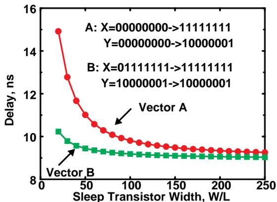
Figure 10. MTCMOS delay dependence on activity
