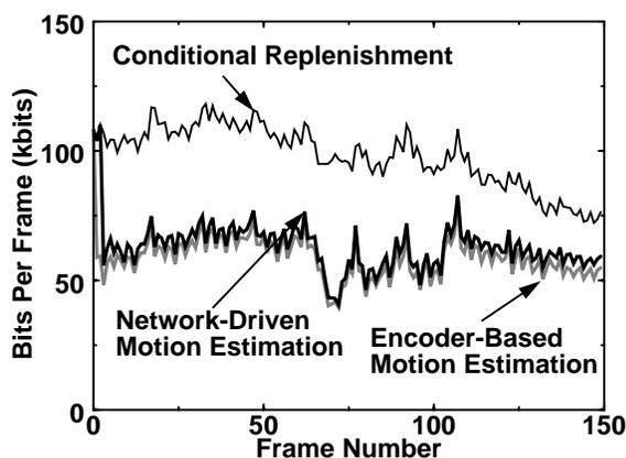
Figure 3. Bit rates for different video algorithms
