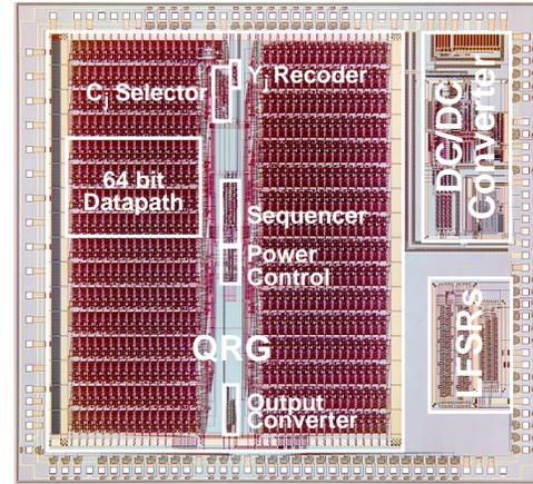
Figure 7. Encryption processor with embedded supply
