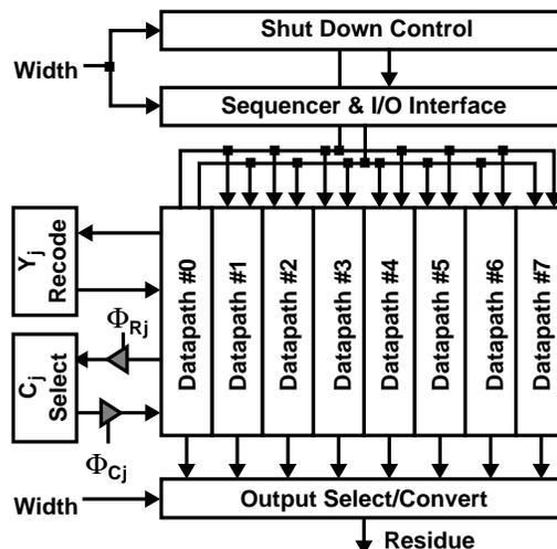
Figure 4. Energy scalable encryption processor
