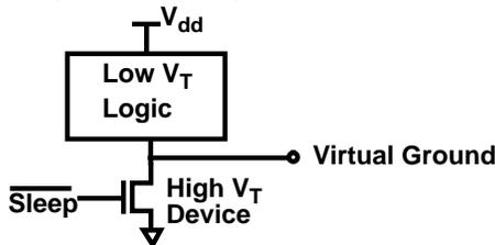
Figure 9. MTCMOS circuit structure
