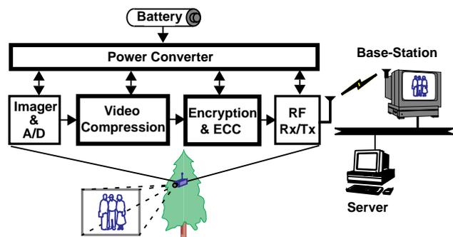
Figure 1. Portable video camera in a networked environment
