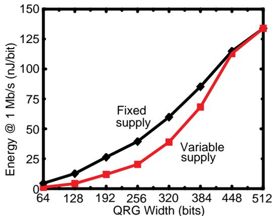
Figure 5. Power dissipation for fixed and variable supply
