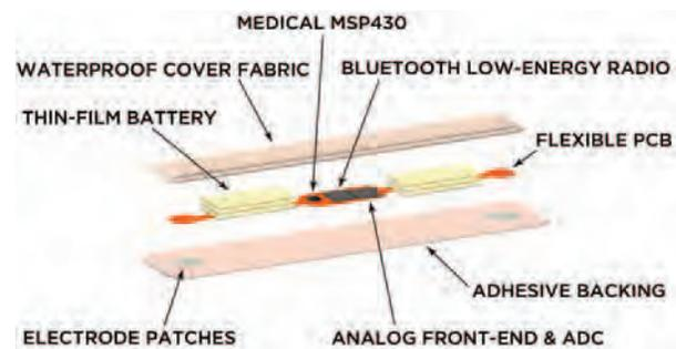
**FIGURE 1:** Wearable ECG system with flexible Band-Aid-like form factor.
