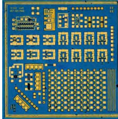
LEFT A test chip used to evaluate the performance of indium gallium arsenide in logic circuits. Image courtesy of the del Alamo group
