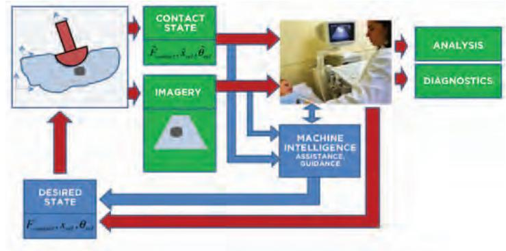
**FIGURE 4:** Ultrasound-imaging system-flow diagram. Our research occurs in the areas shown in blue.
