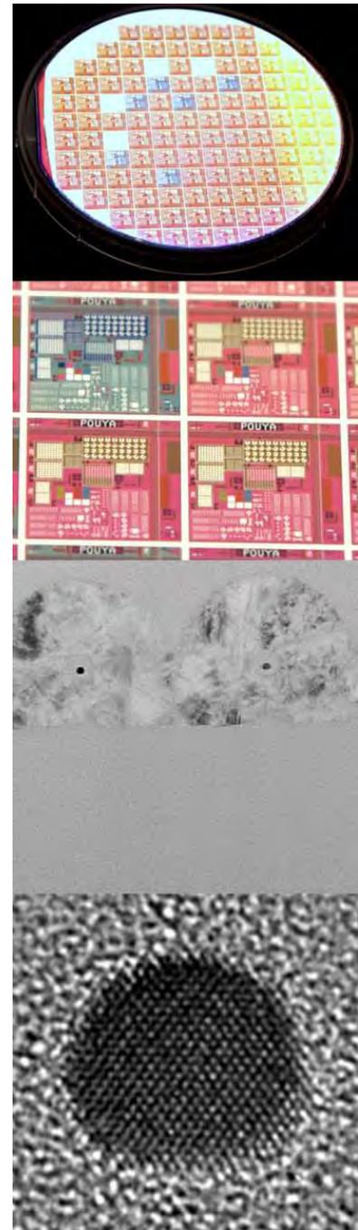
**FROM TOP TO BOTTOM**, four successive magnifications of a test chip with nanowire circuits. (1) A wafer with dozens of chips etched into it. (2) A close-up of four chips. (3) Cross sections of two nanowires in a transistor: at the centers are the nanowires; surrounding them are the transistor elements called “gates.” (4) A close-up of the wire with diameter of 8 nm.
