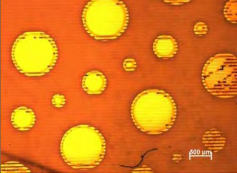
**ABOVE:** To test a new technique for creating micromachines, MIT researchers deposited films of gold on a sheet of plastic; grooves in the plastic are visible as a series of horizontal lines. Image: Corinne Packard and Apoorva Murarka
