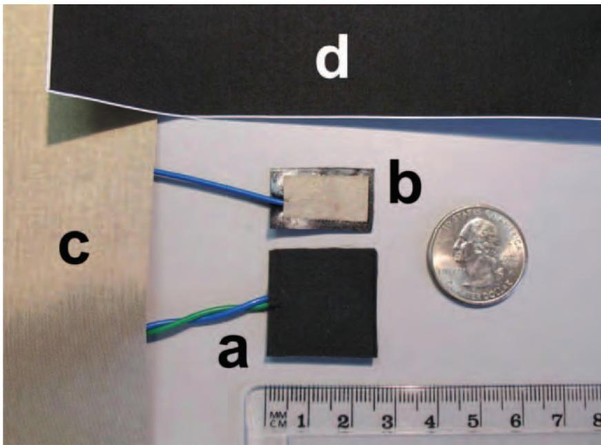
**FIGURE 2:** Photo of a) the capacitive sensing electrode (25mmX25mmX0.75mm), b) the dry CMFB electrode (15mmX25mmX0.35mm), c) the conductive fabric, and d) the nylon fabric.
