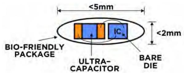
**FIGURE 3:** Illustration of the  $\mu$ Implant sensory monitor. By restricting the size to 2mm by 5mm, we retain the flexibility to either make the device a minimally invasive implant (it is small enough to be injected), or to make it discreetly wearable. The small size means it can be placed easily in body regions (distal arm or leg, for example) of interest, with minimal impact on the patient’s lifestyle.
