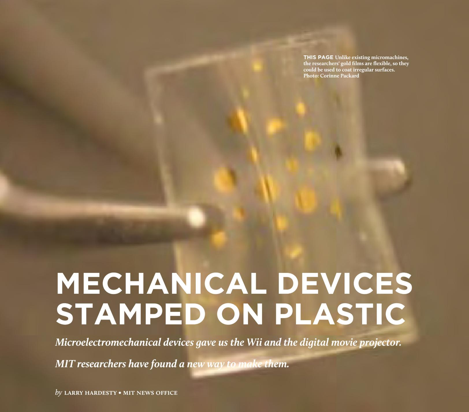
**THIS PAGE** Unlike existing micromachines, the researchers' gold films are flexible, so they could be used to coat irregular surfaces.
