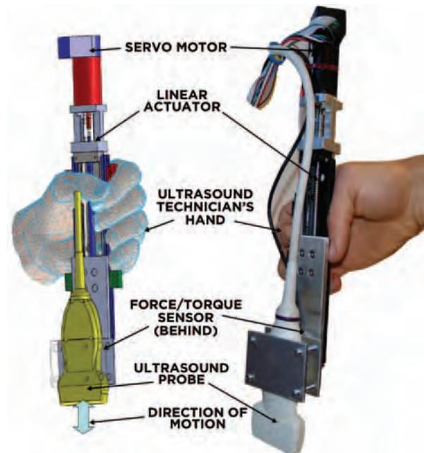
**FIGURE 5:** Force controlled probe.
