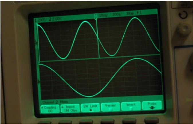
ABOVE: Oscilloscope traces showing the doubling in frequency of an electromagnetic signal processed through their experimental graphene microchip. (Photo / Donna Coveney)
