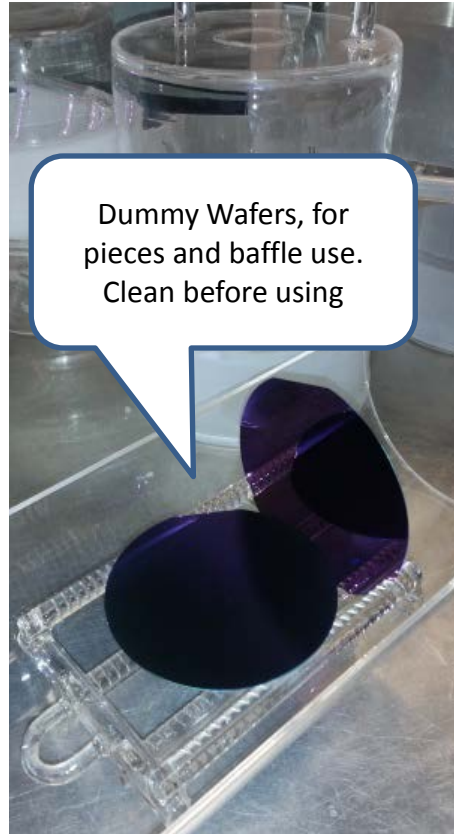
TRL dedicated quartz boat in storage, left, and Dummy wafers for holding pieces, baffling, right
