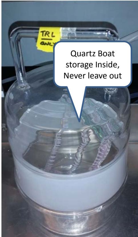
TRL dedicated quartz boat in storage, left, and Dummy wafers for holding pieces, baffling, right
