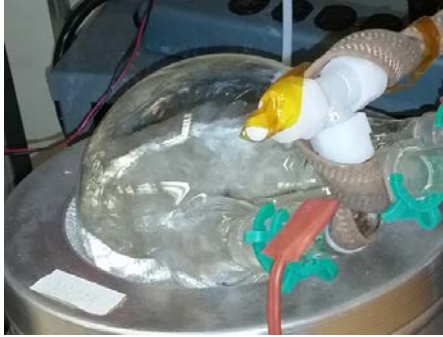
Bubbler with 2.5 SLM N2 Bubbling away, but Water not “climbing” tube, nor condensing
