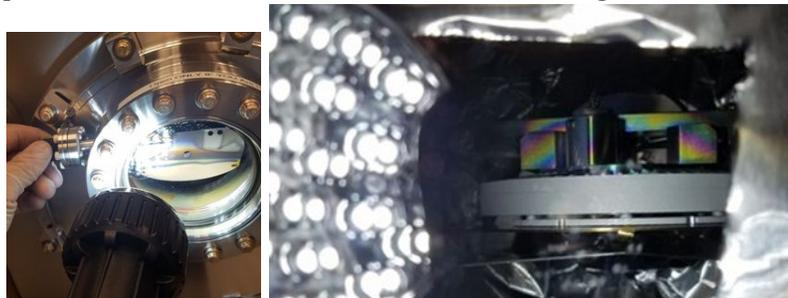
If using multiple deposition, the sample holder will be used to rotate, at slow speed (~20%) until the substrate plate indicator for sample #1 is positioned, then it's turned off. The sample is viewed with the light, thru the opened shutter.
