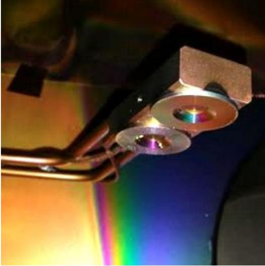
Verify the sensor 1 and 2 are operational, via the Inficon, From Main menu, press Next Menu, until you find the “Sensors Info”. These Quartz Crystals are 6 mHz, declining frequency, and are replaceable by pulling down on the sensor face, and they should be replaced when less than 80% life is displayed, or if they are reporting failure.
