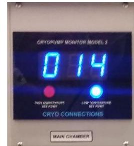
*Cryo Pump Temperature, Normal*
