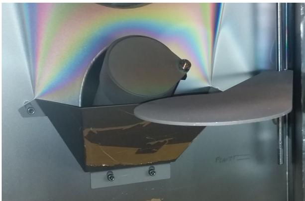
4. a) Verify the shutter for substrate (SHUT) on main menu), by going to Local mode, placing the primary shutter “SHUT” in Local, going back to main menu, and toggling the shutter. It should swing open, exposing the crucible, and closed, going between the crucible and substrate, at the height of the Kaufman. Now
