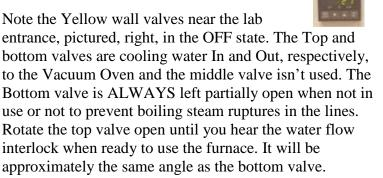
Always close the top valve when not in use, as the cooling water temperature is below the dew point, and the machine will get cold, then wet, and will rust. Wait until temp is below 200 before closing the top valve. Always return Temp Controller to below 20C before leaving.
