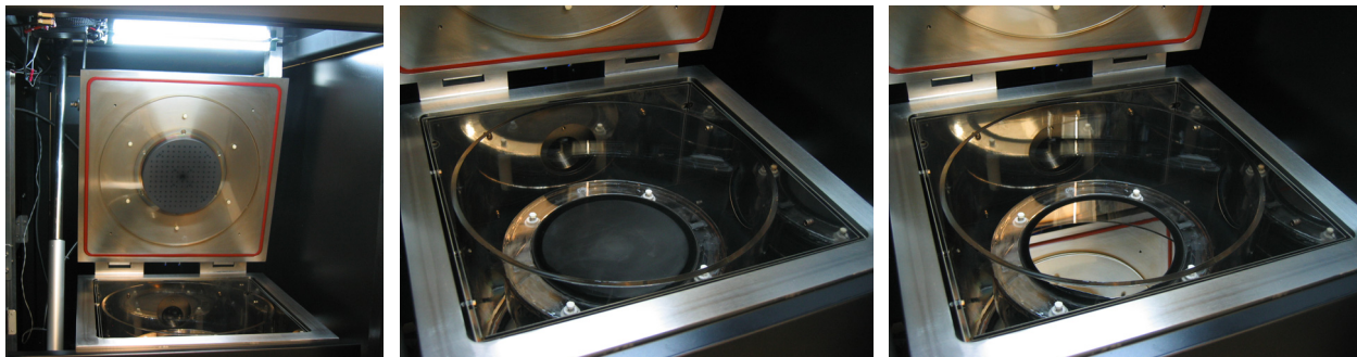
Figure 11. Reactor chamber is open (left), reactor chuck without substrate (center), and with substrate (right)
