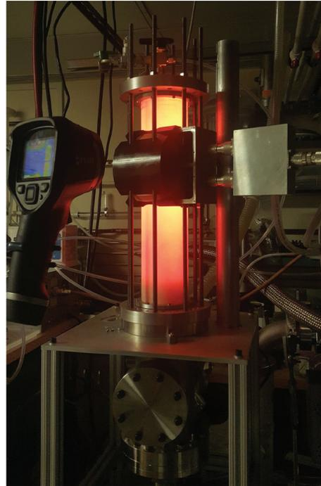
▲ Figure 1: The proposed plasma drive system with  $O_2$  being ionized during a plasma ashing process. The orthogonal coils on the plasma chamber can be seen in the center of the photograph, with the single-input two-output matching system in the sealed enclosure to its right.
