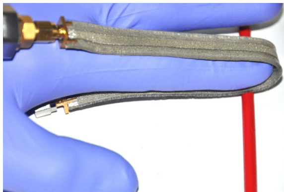
▲ Figure 1: Sensor, mounted on nitrile glove. The sensor is flexible, stretchable, and rugged and is fabricated from silver cloth and silicone rubber.
