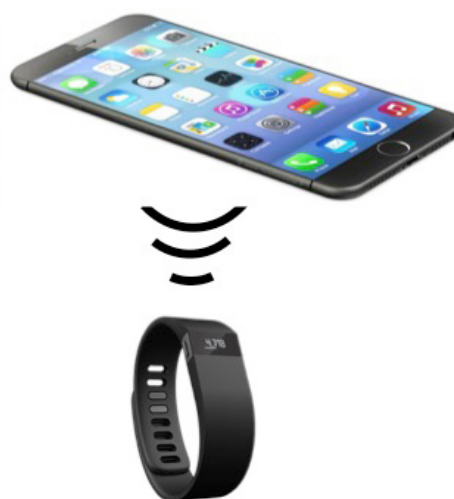
▲ Figure 2: Using a cellphone to provide a burst of energy to a wearable device such as a fitness tracker can typically charge it within a few minutes.
