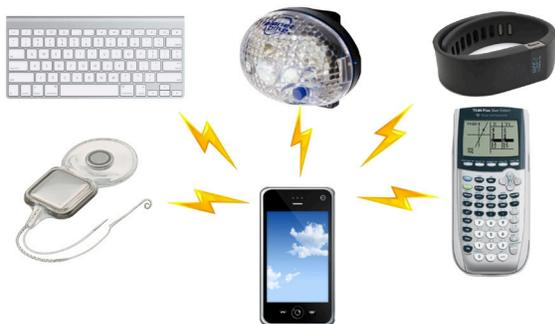
▲ Figure 1: Our wireless charging system uses a smartphone to recharge various lower-power portable devices, such as cochlear implants, wireless keyboards, bicycle lights, fitness trackers, and calculators. The smartphone charges most devices in 2 minutes for a typical day's use.
