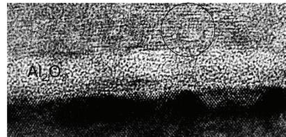
**FIGURE 1:** Example XTEM, a constructed device showing silicon nanoparticles (2.9 nm, circled) embedded in ALD-deposited  $\text{Al}_2\text{O}_3$ .
