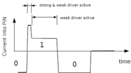
▲ Figure 1: Abstract modulator diagram and its corresponding pre-emphasized current profile for a 010- input bit pattern. The weak driver has a very strong NMOS and a weak PMOS.
