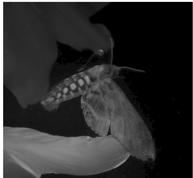
▲ Figure 2: A moth carrying a resonator during flight. The fine-tuned resonator will resonate with the moth's vibration frequency of 25 Hz, creating maximum swing amplitude to generate power. (Courtesy of Daniel Group at the University of Washington.)
