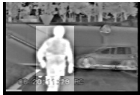
▲ Figure 2: Segmentation result for night driving environment.
