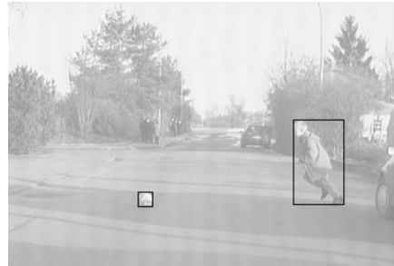
▲ Figure 1: Segmentation result for urban daytime driving environment.
