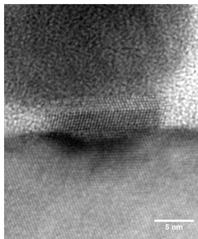
▲ Figure 2: GaP nanowire grown on Si <111> substrate using Ag catalyst.
