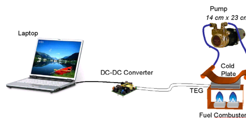
▲ Figure 2: Schematic for final demonstration system, set to include a module containing both thin-film and bulk TE materials.
