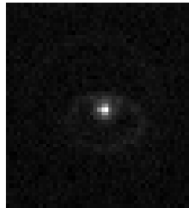
▲ Figure 2: A single strontium ion is trapped with the surface electrode NbN ion trap at 6K, sideband-cooled to its quantum ground state motion.
