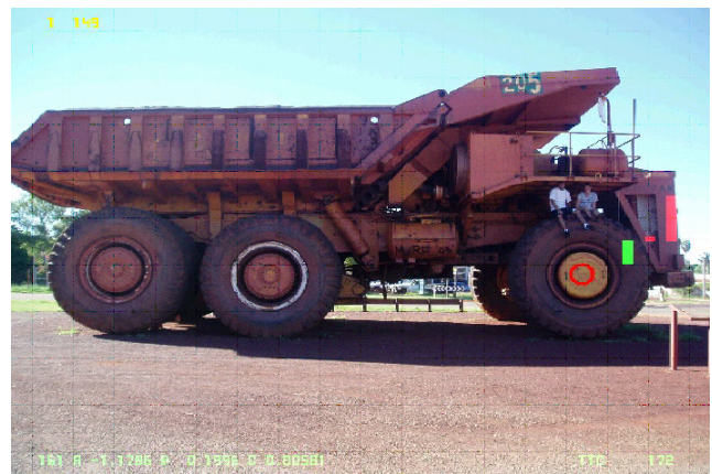
▲ Figure 2: The TTC calculation process for one video sequence. The circle represents the focus of expansion with coordinate at the bottom right corner. The three bars represent the relative speed between camera and object. The TTC value is at the upper left corner of each image.
