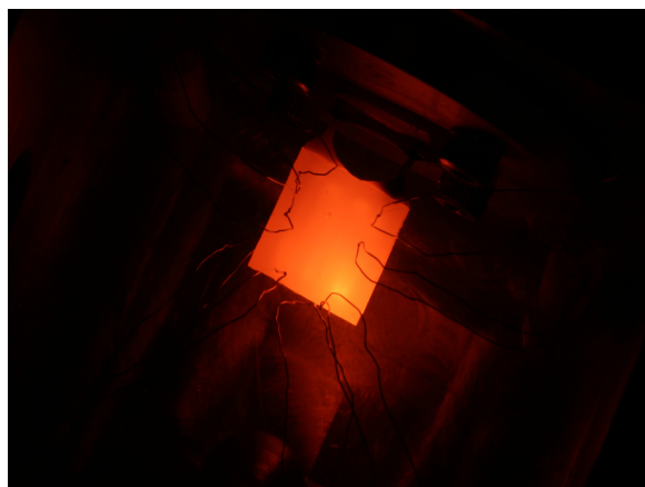
▲ Figure 2: Autothermal combustion of propane under 25-mTorr vacuum.
