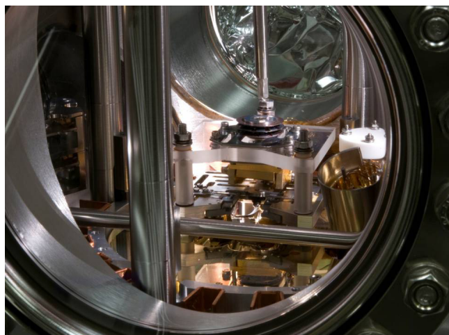
▲ Figure 1: Image of the VT-SPM (Omicron GmbH) inside the UHV chamber ( 3 \times 10^{-10} Torr). Surface potential measurements are recorded relative to a Pt-Ir coated Si tip. Measurement of the tail states requires equilibrium in the channel. However, the resistance of the channel is extremely large below the threshold. Further measurements are required to determine whether the measurement of the extreme tail states have indeed been made under equilibrium conditions.
