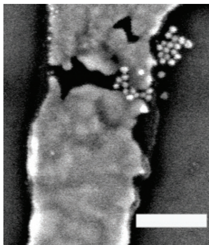
▲ Figure 1: An SEM image of assembly of citrate-stabilized 20-nm-diameter gold particles by the application of a 2V_{pp} , 1-MHz alternating field across a 23-nm gap for 120 seconds. A solution concentration of 7 \times 10^{10} particles/ml was used for this assembly. Scale bar=200 nm.
