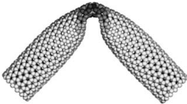
Figure 1: Simulated bending of single wall CNT [1].
