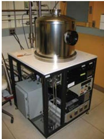
Figure 1: PECVD Machine for growing CNTs at MIT
