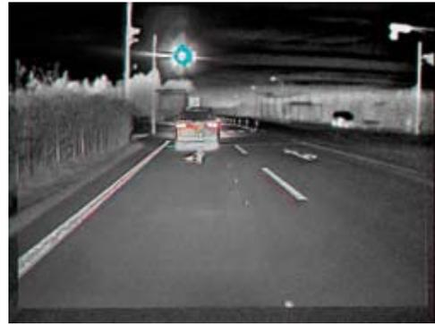
Figure 2: Fused image of a night driving scene combining the visible image (Figure 1) with a near infrared image and far infrared image (not shown). The fused image contains more information than any individual image.
