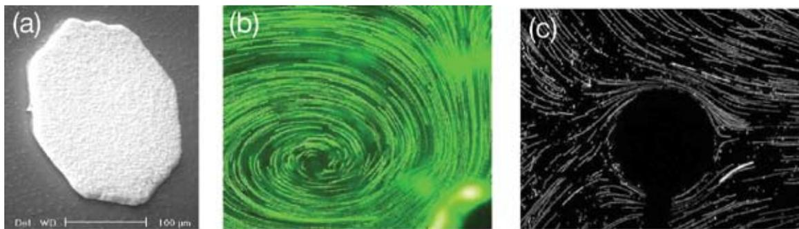
Figure 1: (a) SEM image of an electroplated gold post ( $12\mu\text{m} \times 150\mu\text{m}$ ). (b) ICEO convection around the post, visualized by streaks of fluorescent tracers used  $\mu$ PIV. (c) faster ICEO flow past a post held at fixed potential.
