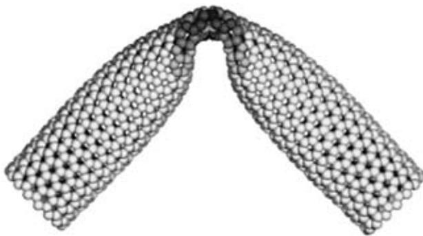
Figure 1: Simulated bending of single wall CNT [1].
