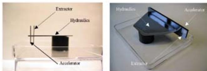
Figure 1: Field view of a finished device. The engine is composed of a hydraulic system and two electrodes, involving a total of four substrates. The electrodes are assembled to the hydraulic system using microprecision mesoscale silicon springs.
