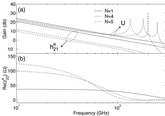
Fig. 27: (a) Unilateral power gain magnitude, current gain magnitude, and (b) output resistance for  $X_{\text{step}} = 500 \text{ \AA}$ ,  $\Delta = 1.2 h\omega_{LO}$ . As the number of steps increases ( $N = 1, 4, 5$ ),  $U$  extends in frequency by means of resonance.
