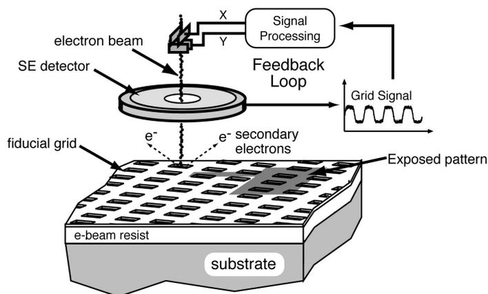
Fig. 4: Schematic of the global-fiducial-grid mode of spatial-phase-locked electron-beam lithography. The periodic signal detected from the fiducial grid is used to measure placement error, and feed a correction signal back to the beam deflection system.
