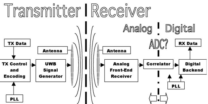
Fig. 13 : UWB Generic Transceiver Block Diagram
