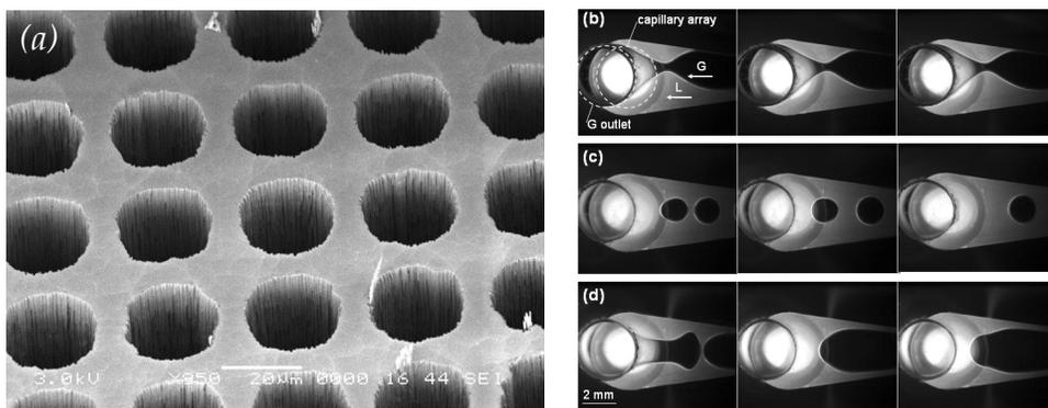
Fig. 19: (a) Microfabricated capillary array in silicon. Annular (b), bubbly (c) and slug flow (d) into the separator.
