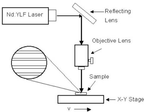
Fig. 5: An apparatus for scanned laser annealing (SLA) of Cu interconnects.
