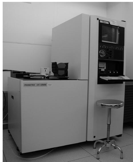
*KLA-Tencor UV1280 film thickness measurement system*
