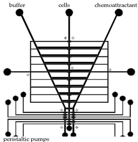
Fig. 7: Two layer mask for the chemotaxis chamber containing valves and peristaltic pumps.
