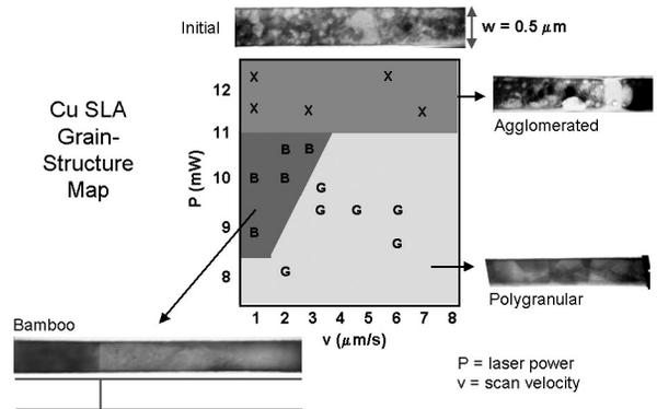
Fig. 6: The grain structures that result from SLA depend on the laser power and the scan velocity. Long-grained bamboo structures are obtained at intermediate powers and low velocities.
