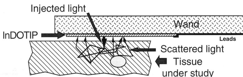
Fig. 39: An illustration of one way the DOT OEIC die might be mounted on the end of a wand and used for DOT subsurface imaging of soft body tissue. In use, each VCSEL is illuminated in turn (the figure shows one turned on) and the pattern of scattered light seen by the detector array is recorded. With this information, an image of the sub-surface structure can be constructed.
