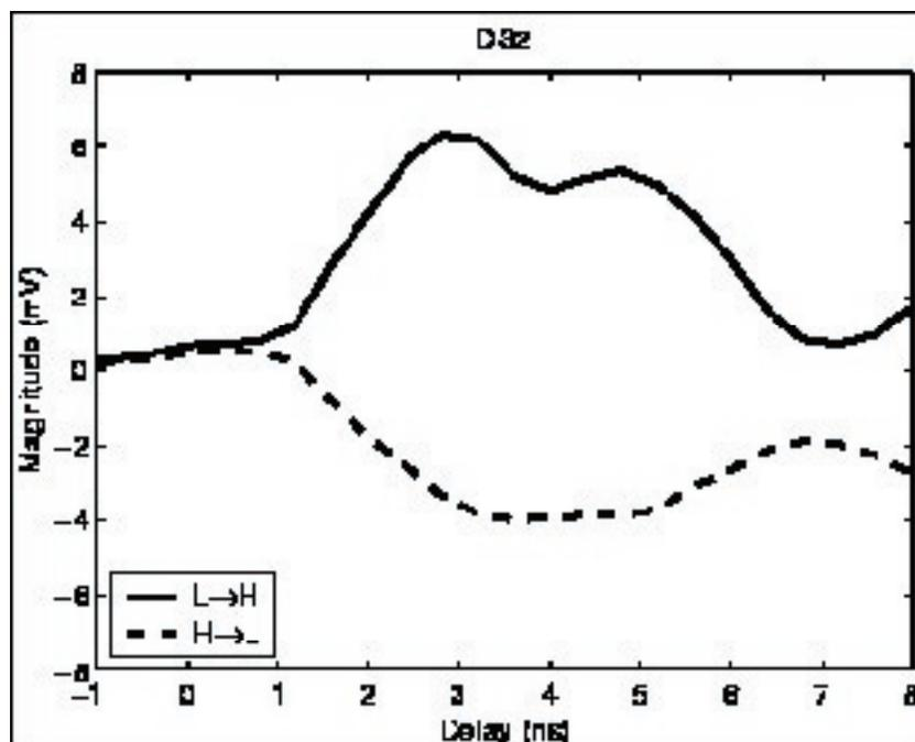
Fig. 29: Measured substrate noise with an on-chip sampling scope.
