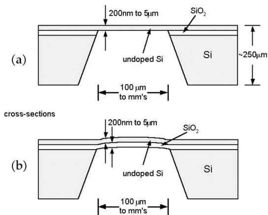
Fig. 49: (a) Micromachined single crystal Si membrane. (b) Pre-buckled composite Si-SiO<sub>2</sub> membrane
