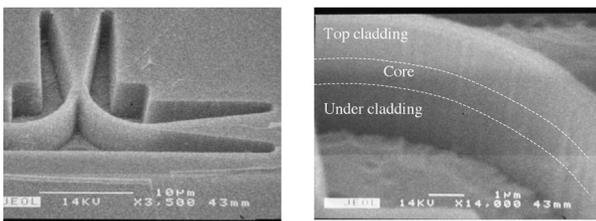
Fig.16: SEM images of an air trench T-splitter (x3,500) and an air trench waveguide (x14,000)
