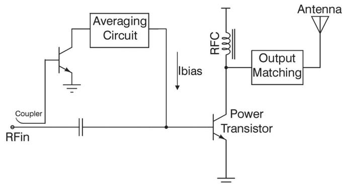
Fig 18: Adaptive Current Biasing Block Diagram
