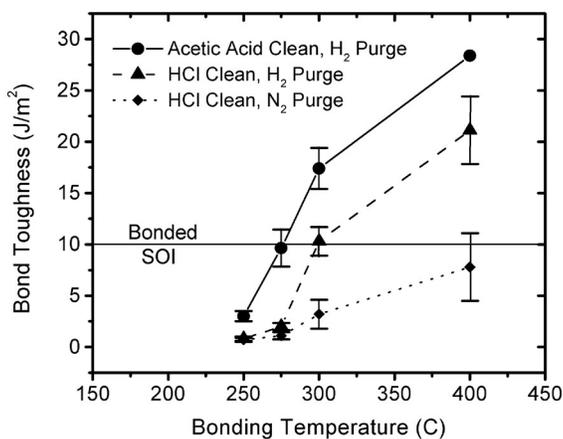
Fig. 1: Variation of bond toughness for wafers 0.4MPa thermo-compression bonded using 300nm-thick Cu films at different temperatures, after different surface preparations. Wafers bonded after an acetic acid pre-clean had higher bond toughness than bonded SOI wafers, even when bonded at temperatures below 300C. The point indicated by an "\*" is a lower bound.
