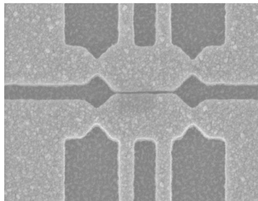
Fig. 20: Scanning electron micrographs of device pattern with feature size  $\sim 20$  nm achieved by X-ray nanolithography.
