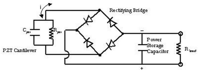
Fig. 31: Electrical equivalent circuit model of PMPG with full-wave rectifier
