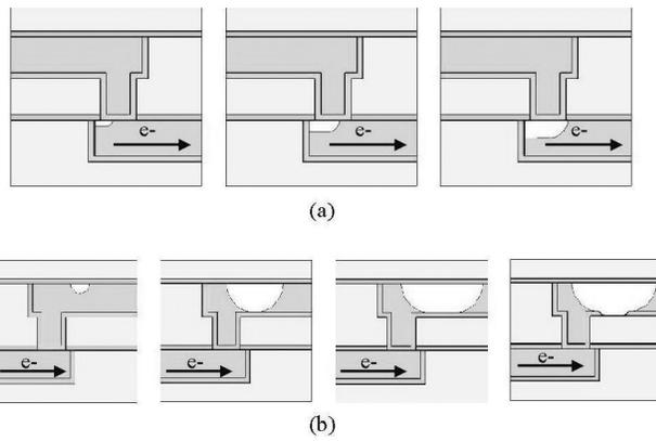
Figure 5: Schematic diagrams of M1-type test structures and in (b) M2-type structures.
