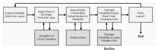
Fig. 39: A flowchart for a full hierarchical circuit-level reliability assessment, the basis for the prototype tool ERNI.
