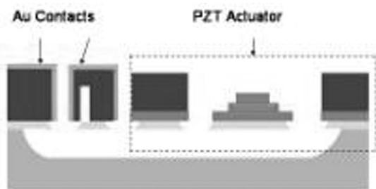
Fig. 37: A schematic view of the switch.
