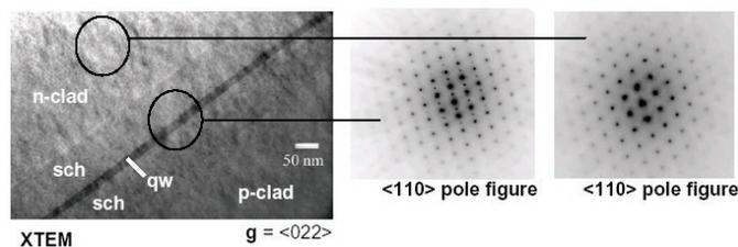
Fig. 7: X-TEM of device structure with an  $\text{In}_{0.32}\text{Ga}_{0.68}\text{P}$  quantum well. Electron diffraction of the quantum well (center) shows ordering superspots, while the clad (right) does not.
