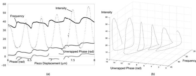
Fig. 23: (a) Plot of three measurable quantities in ISPI transverse chirp gapping fringes: frequency, phase, and average intensity as a function of gap. (b) Within the  $\pm 1$  range of fringe frequency resolution, a unique correspondence to gap is found from a combination of all three fringe quantities. (Note that in both plots frequency is upshifted by  $\sim 4x$  due to zero padding.)
