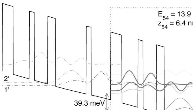
Fig. 40: Conduction band profile calculated using a self-consistent Schrödinger and Poisson solver (80% conduction band offset) biased at 64 mV/module. Beginning with the injector barrier, the layer thickness in Å are 54/78/24/64/38/148/24/94. The 148-Å well is doped with Si at  $1.9 \times 10^{16}/\text{cm}^3$ , yielding a sheet density of  $2.8 \times 10^{10}/\text{cm}^2$ .
