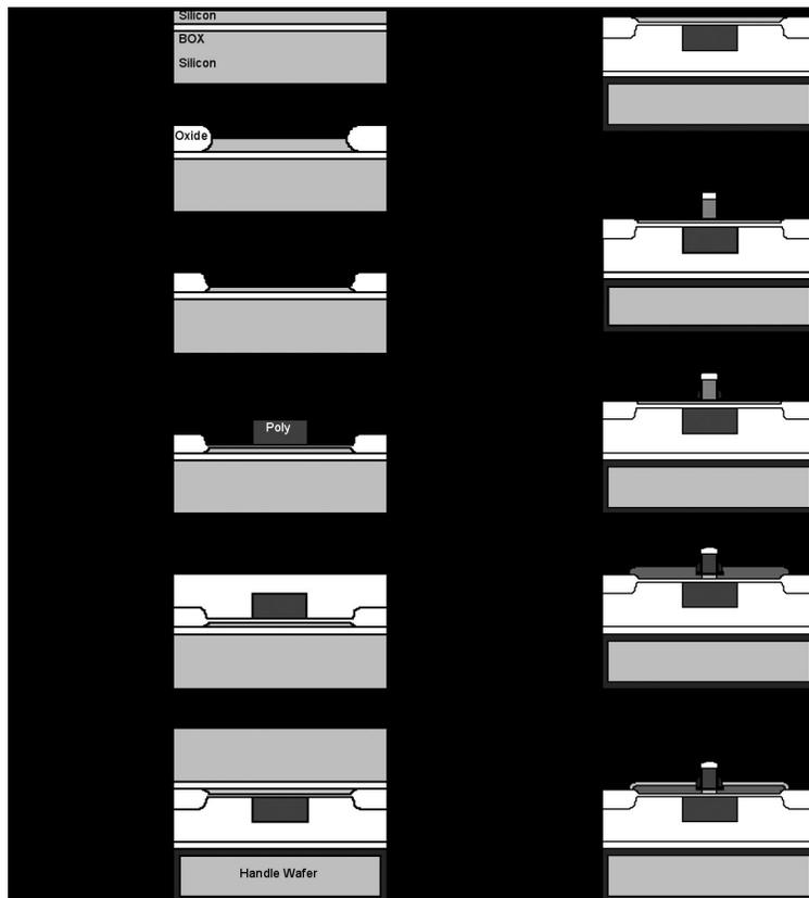
Fig. 1: Ultra-Thin Si DG MOSFET Fabrication
