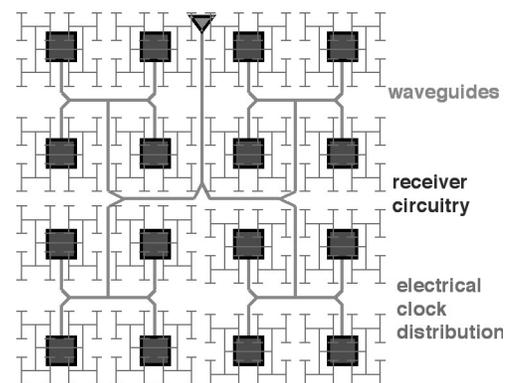
Fig. 36: Global optical clock with local electrical clock distribution.
