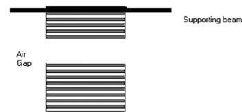
Fig. 5: The illustration of the one-dimensional photonic crystal with a large air defect.
