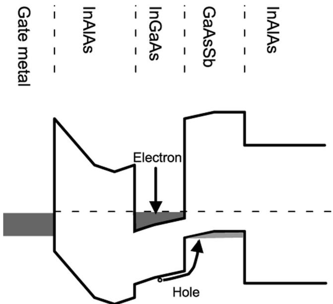
Fig. 19: Band profile of heterostructure under gate.
