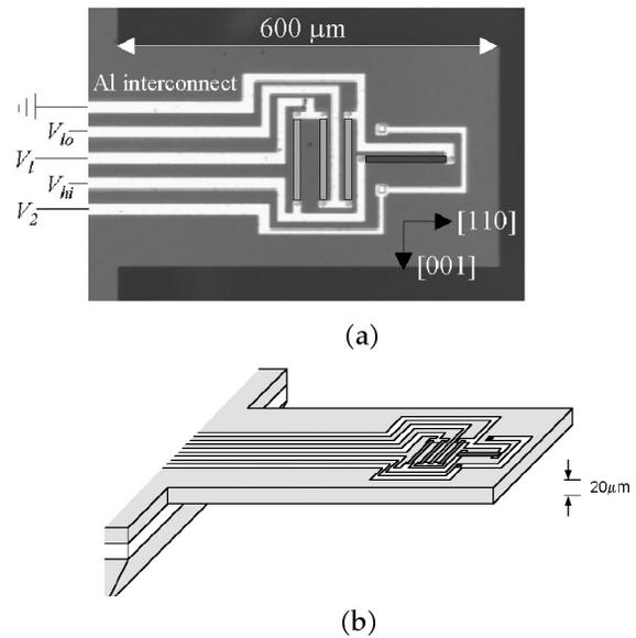
Fig. 51: (a) Top view and (b) Perspective view of a micromachined piezocantilever for *in-situ* stress measurements during film deposition
