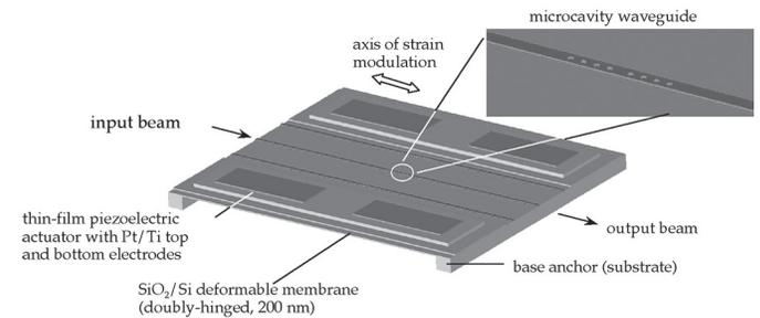
Fig. 17: Device schematic of the tunable photonic-bandgap micro cavity waveguide, with strain modulation via thin-film piezoelectric actuators on the deformable membrane.
