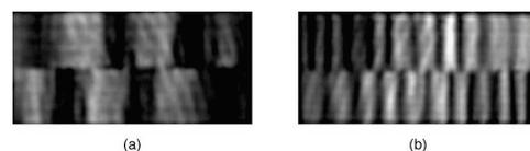
Fig. 22: Illustration of fringe variation with gap. Between (a) 4.3 mm and (b) 19.3 mm gaps the number of fringes increases by 0.51 fringe/mm.
