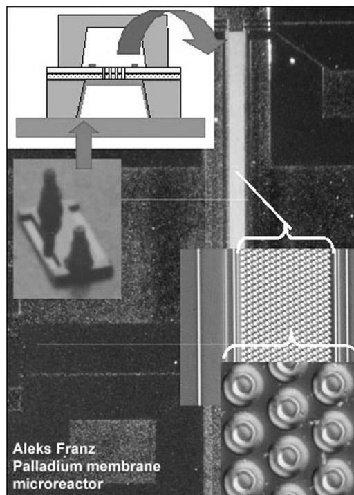
Fig. 25: Palladium micromembranes for hydrogen purification. Membrane device, 200 nm palladium film supported on silicon nitride and oxide membrane with 4 micron holes, image of membrane structure and integrated heater, actual device components.
