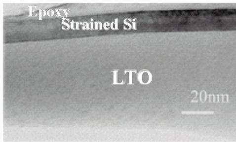
Fig. 3: XTEM of ultra-thin strained-Si on insulator. Strained Si thickness is 13-15 nm
