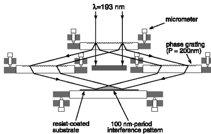
Fig. 30: Achromatic interferometric lithography (AIL) configuration employed to produce 100 nm-period gratings and grids.
