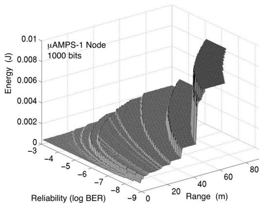
Fig 2: Energy-scalable communication on  $\mu$ AMPS-1 node.
