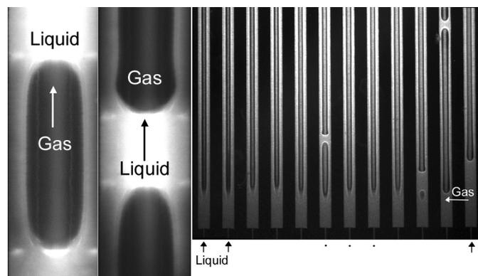
Fig. 24: Gas-liquid flow in a single microchannel with a field of view (FOV) of 435 μm x 1.3 mm (left) and multiple microchannels, FOV of 10 mm x 12 mm (right).
