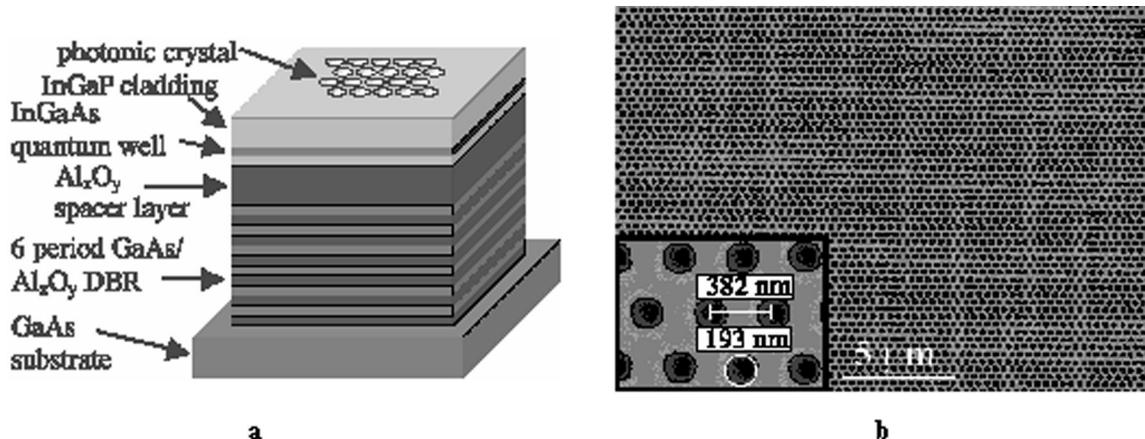
Fig. 19: a) The 2D PC structure. b) Scanning electron micrographs of PC structure.
