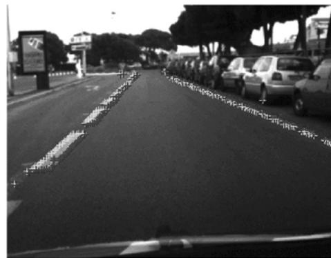
Fig. 32: Results from the lane marker detector
