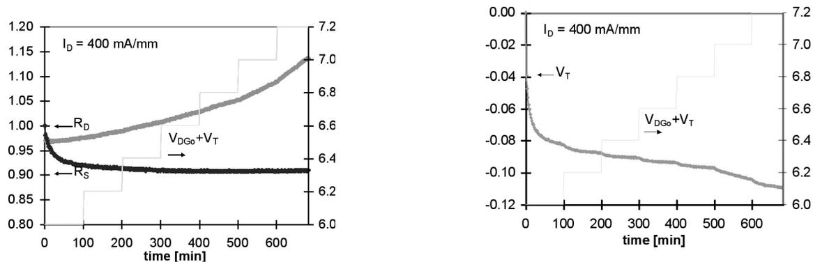
Fig. 21: Time evolution of the normalized drain resistance and source resistance (left) and change in threshold voltage (right), for a voltage step-stress experiment on a PHEMT at constant drain current of 400 mA/mm.
