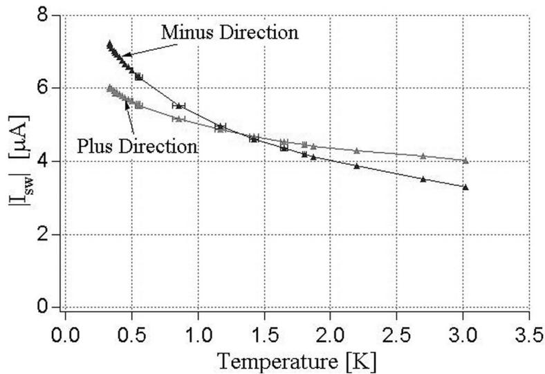
Fig. 16: Switching current for the plus and minus direction of a circular, 1-D Josephson array fabricated in the quantum regime. The switching current is a measure of the depinning rate in each direction. The crossover indicates that the preferred direction changes as a function of temperature. This is a possible signature of quantum effects.
