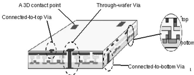
Fig. 40: Different types of via/contact for 3D ICs.
