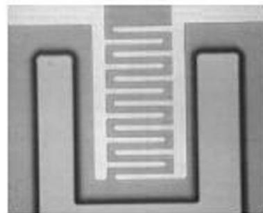
Fig. 33: Top View of interdigitated PMPG fabricated
