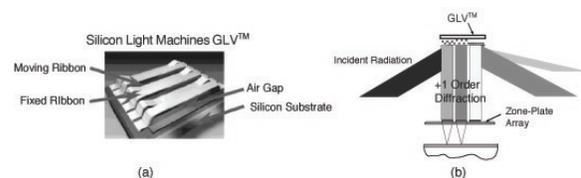
Fig. 10: Schematics of the Silicon Light Machines Grating Light Valve (GLV) device. (a): Fixed and electrostatically-deflected moving ribbons create a variable-height grating. (b): Incident light will be diffracted from the grating at a known angle, with varying intensity depending on the height of the grating. Each pixel, a small patch of the grating, diffracts onto a single zone plate, thus turning on and off (or grayscaleing) each pixel written onto the substrate in ZPAL.
