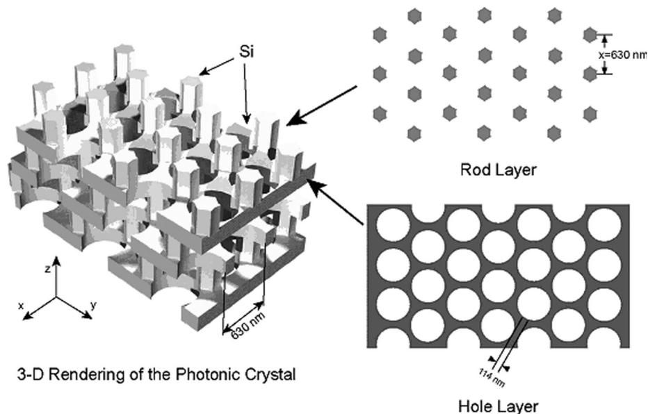
Fig. 22: A schematic of the MIT 3D photonic crystal.
