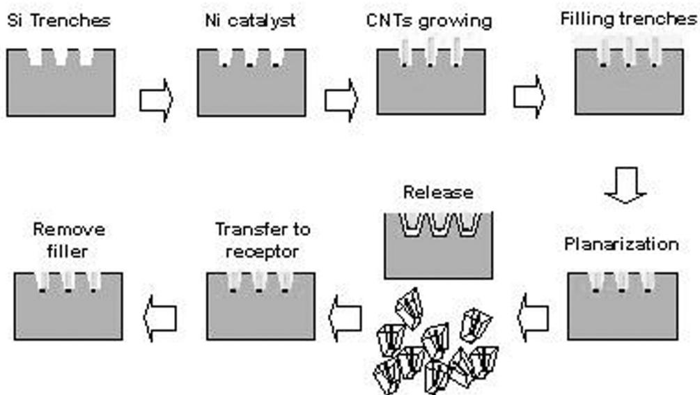
Fig 55: Nanopelleting of CNTs
