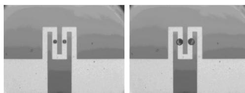
Fig. 12: A platinum heater with machined bubble nucleation sites, before and after bubble formation.
