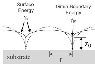
Fig. 11: When islands impinge, grain boundaries form as islands strain to close the gap between them, zipping a distance  $z_0$  to replace two surfaces of energy  $\gamma_s$  with a boundary of energy  $\gamma_{gb}$ .
