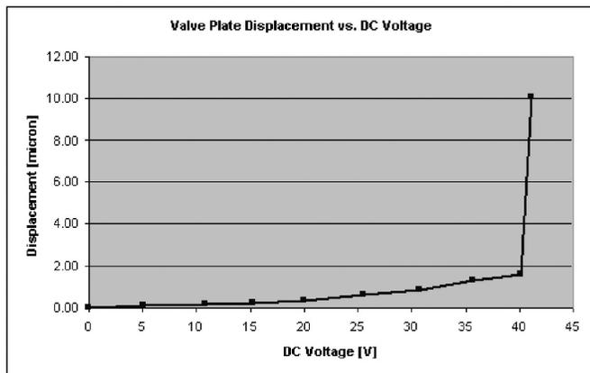
Fig. 27: Valve plate displacement vs. applied DC voltage
