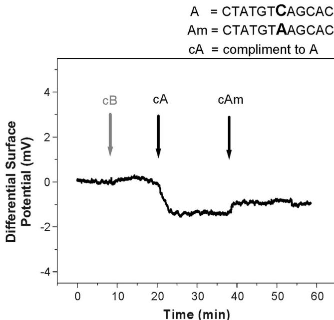
Fig. 6: Differential surface potential from two sensors which were functionalized with probe oligonucleotides A and Am which differ only in a single base. Control solutions with non-complementary target oligonucleotide cB show no differential signal, while injection of 80 nM of complementary sequences cA and cAm both show a distinctive hybridization signal.
