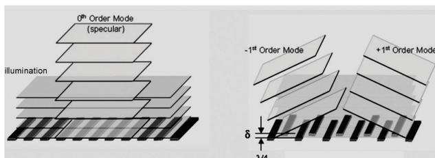
Fig. 16: Concept for measuring displacement with InterDigitated (ID) fingers. When the fingers are illuminated with a laser, the reflected light produces a diffraction pattern composed of several modes. The intensities of these modes depend on the relative out-of-plane distance between the ID finger sets.
