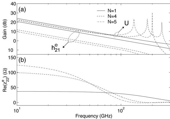
Fig. 27: (a) Unilateral power gain magnitude, current gain magnitude, and (b) output resistance for  $X_{step} = 500 \text{ \AA}$ ,  $\Delta = 1.2 h\omega_{LO}$ . As the number of steps increases ( $N = 1, 4, 5$ ),  $U$  extends in frequency by means of resonance.
