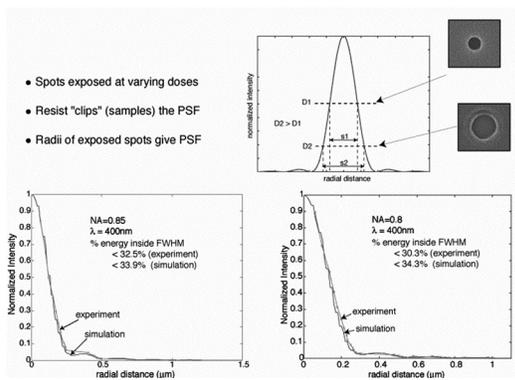
Fig. 9: Top: Experimental process for quantifying the PSF. Spots of several exposure times were patterned in photoresist, which acts as a sampler of the PSF. The radii of the exposed spots can be assembled to form the PSF. Bottom: PSFs for zone plates of NA=0.85 (left) and NA=0.8(right) were determined experimentally using the simulation tools. The results show excellent agreement.
