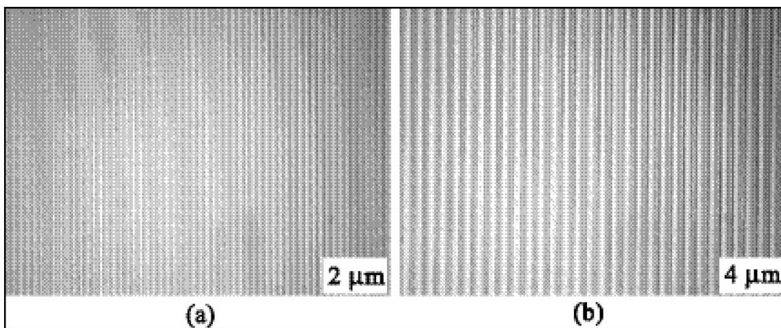
Fig. 13: Grating images written by VP-SBIL with period (a) 2.0  $\mu\text{m}$  and (b) 4.0  $\mu\text{m}$ .
