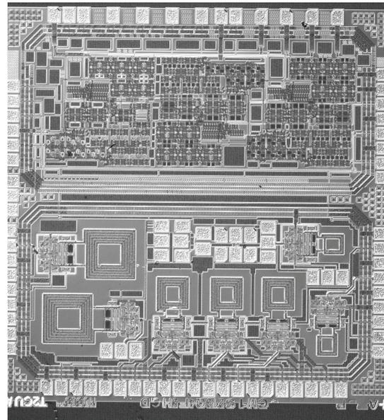
Fig. 9 Die photo of the VCO chip and digital circuits
