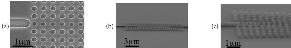
Fig. 54: a) Top view SEM of coupling design from Figure 51(a) after e-beam lithography in PMMA. The bulk photonic crystal has hole diameter of 307nm, while the defect has diameter of 244nm. b) Top view SEM of coupling designs from Figure 51(b) after  $\text{SiO}_2$  etch. c) Top view SEM of coupling design from Figure 51(c) after  $\text{SiO}_2$  etch.
