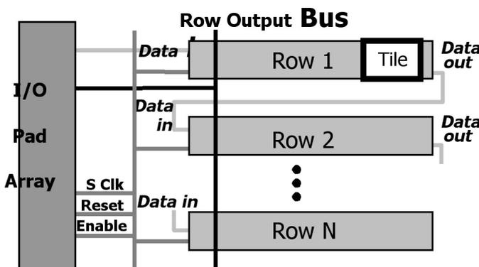
Fig. 1: Variation test chip architecture.
