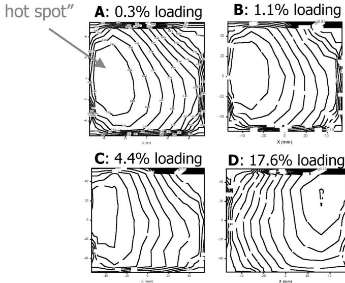
Fig. 2: Normalized wafer-scale DRIE etch rates. Uniform grid of circles etched with diameter  $\Phi$  and separation distance (mm/mm): A (0.6/16); B (2/16); C (2/8); D (2/4).
