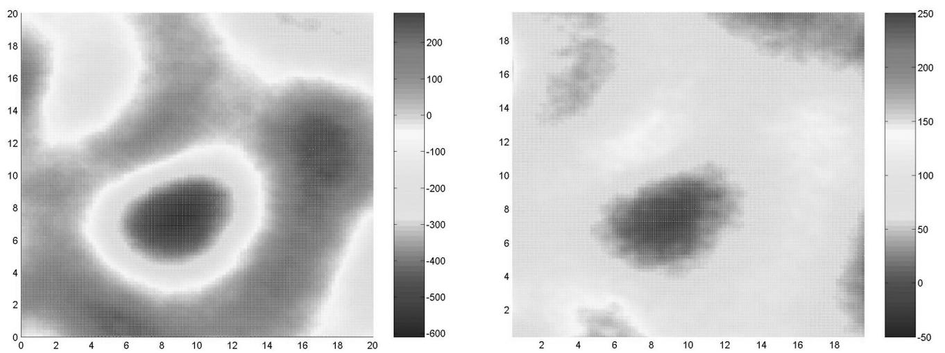
Fig. 5: (a) Nanotopography map measured on a chip size region on bare wafer; (b) Additional nitride erosion caused by the nanotopography shown in (a); height variation is shown in color bar and is in angstroms
