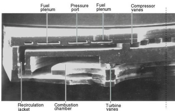
Fig. 35: SEM cross-section of six-wafer combustion system.
