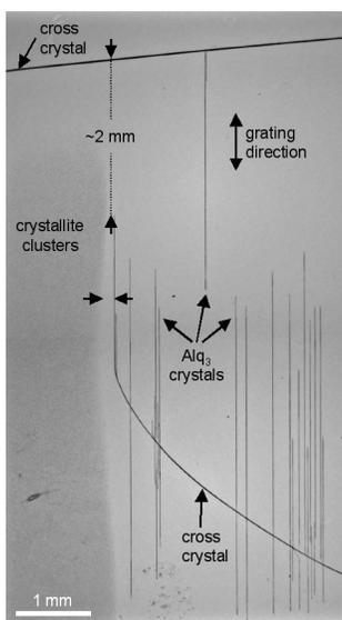
Fig. 47: Macroscopic  $Alq_3$  crystals on a nanopatterned substrate.
