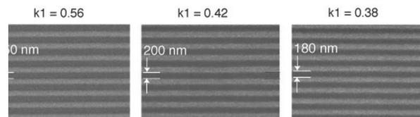
Fig. 17: Exploring the limits of  $k_1$  with ZPAL. High-numerical-aperture zone plates (0.85 and 0.9) can operate at low  $k_1$  factors (below 0.4). Sub-70 nm patterning should be possible, by operating at the demonstrated  $k_1=0.39$ , with 0.9NA zone plates and  $\lambda = 157\text{nm}$ .
