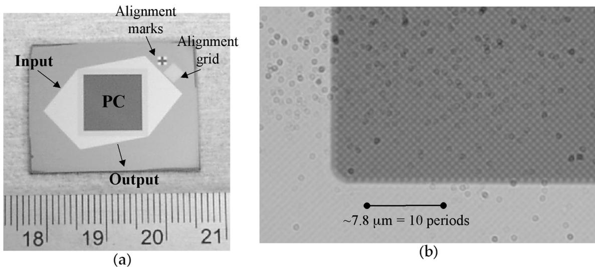
Fig. 50: (a) Photograph showing a top view of the superprism hard mask layers on a silicon substrate. (b) Microscope image of the corner area of the photonic crystal region shown in Fig 48(a). The defects in the photograph are due to dust particles in the microscope optics that could not be readily removed.
