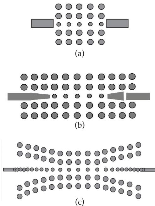
Fig. 52: a) Schematic of coupling from untapered dielectric waveguide. b) Schematic of coupling from a tapered dielectric waveguide. c) Schematic of adiabatic transition from a dielectric waveguide into strongly coupled cavities and tapered cladding.
