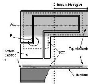
Fig. 45: Device schematic of water-immersible piezoelectric actuator.
