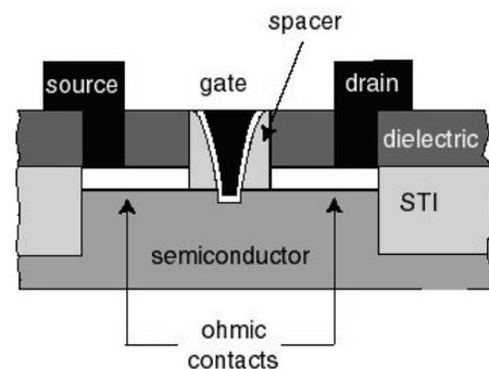
Fig. 23: Cross-sectional view of a tentative device design for an InP-HEMT fabricated using a CMOS-like process.
