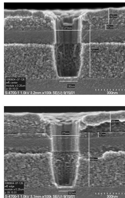
Fig. 4: 0.25  $\mu\text{m}$  via cross sections for the best IPS hexafluoro-1,3-butadiene process for LKD film. BARC BT: 800 W Outer, 400 W Inner, 300 W Bias, 4 mT, 5 sccm  $\text{C}_4\text{F}_6$ , 10 sccm  $\text{O}_2$ , 100 sccm Ar, 15s; SiCN BT: 1000W Outer, 200 W Inner, 300 W Bias, 10 sccm  $\text{C}_4\text{F}_6$ , 5 sccm  $\text{O}_2$ , 100 sccm Ar, 25s; Main Etch: 1540 W Outer, 260 W Inner, 1800 W Bias, 7 mT, 12 sccm  $\text{C}_4\text{F}_6$ , 100 sccm Ar, 60s. (IPS-LK4-XLK)
