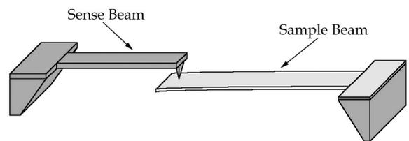
Fig. 50: Micromachined 'sample' cantilever being actuated by AFM 'sense' cantilever
