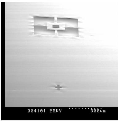
Fig. 6. SEM picture of the one-dimensional photonic crystal with a large air defect.
