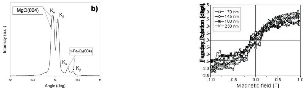
Fig. 17: Left: XRD spectra of a 420nm maghemite ( $\text{Fe}_2\text{O}_3$ ) film deposited on a MgO (001) substrate, showing the cube-on-cube film-substrate epitaxial relationship. Right: Faraday rotation measurements of maghemite with different thickness at a wavelength of 645nm showing an average saturation rotation of about 1.9deg/ $\mu\text{m}$ .
