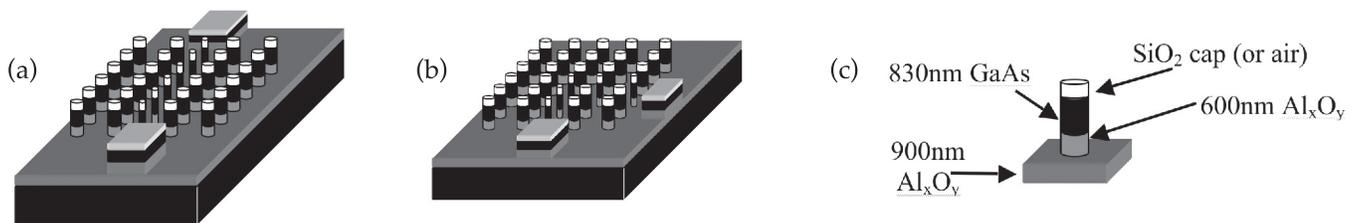
Fig. 51: (a) Schematic of a linear PC waveguide. (b) Schematic of a 90° bend PC waveguide. (c) Schematic of a cylindrical pillar structure. For the bulk photonic crystal, the pillar diameter is 300nm; for the defects, the diameter is 250nm.
