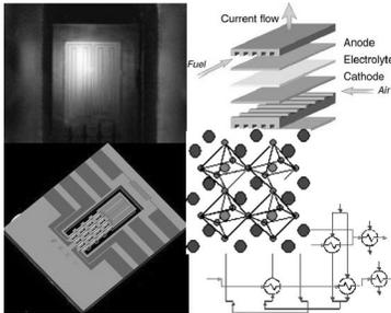
Fig. 29: Different elements of the fuel processing program; fuel processor, microcombustor, solid oxide fuel cell schematic, crystal structure of catalysts, energy integration diagram.
