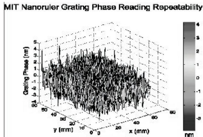
Fig. 36: Wafer phase mapping repeatability (nm), for a 400 nm-period grating that was written and then read by the Nanoruler.
