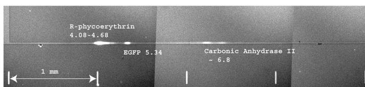
Fig. 8: Isoelectric focusing in 4mm channel. Electric field was 35.7 V/cm. Carbonic anhydrase II was labeled by cysteine-specific labeling (rhodamine-maleimide), while R-phycoerythrin and EGFP are naturally fluorescent. The focusing was achieved within 30 s after applying the electric field. Wider channel regions at both ends are filled with catholyte and anolyte, respectively, and pH gradient was established within 4mm channel.
