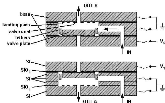
Fig. 26: Switch valve cross section
