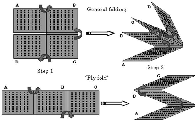
Fig. 64: Examples of how 3D structures can be obtained by folding pre-fabricated thin 2D membranes in a two step process. Black dots
