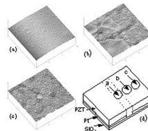
Fig. 46: AFM images of the PZT film surface and intersection diagram of the PZT film on the separated Pt bottom electrode region; (a) PZT surface exact on the separated Pt; (b) PZT surface near on the separated Pt; (c) PZT surface on Pt bottom electrode; (d) Schematic diagram of the region "P" in Figure 1(a) which was observed by AFM.
