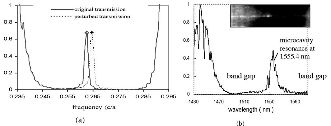
Fig. 18: (a) Computed transmission shift through perturbation theory in the photonic band gap; (b) Measured static microcavity resonance with Q of 159. Inset; top view of microcavity waveguide in transmission.
