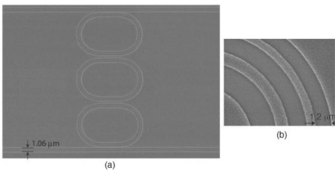
Fig. 15: Scanning electron micrographs of patterns exposed with our continuous-scan 0.9 NA UV-ZPAL system operating at  $\lambda = 400\text{nm}$ . Sub-pixel stepping enables patterning of curved structures with smooth edges. (a) waveguides with ring resonators, (b) one quadrant of a zone plate.
