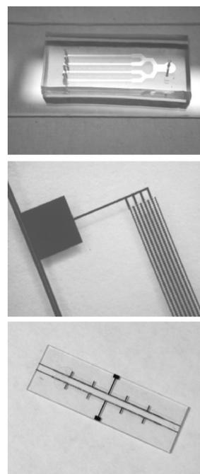
Fig. 11: (Top) Microfluidic cell-adhesion assay device that is fabricated using rapid prototyping techniques; (Middle) Cell electroporation lysis device that contains arrays of electrodes; (Bottom) Organelle sorting device that uses miniaturized isoelectric focusing field flow fractionation technique.
