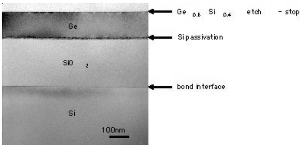
Fig. 22: Ge on Insulator (GOI) structure fabricated by wafer bonding and epitaxial layer transfer from a Ge/SiGe/Si virtual substrate.
