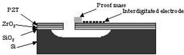
Fig. 30: Surface micromachined PMPG device
