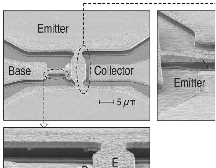
Fig. 28: Schematic and SEM pictures of a HBT device using airbridges for electrode isolation.
