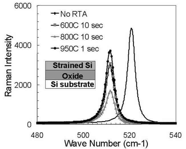
Fig. 4: Raman analysis of SSOI using 325 nm excitation shows shift of 9 wavenumbers between silicon and strained-silicon peak corresponding to a strain of 1.2%, in excellent agreement with the strain in the as-grown film prior to layer transfer. In addition, no shift in the strained-Si peak is observed after RTA. Raman data courtesy N. Klymko, IBM Microelectronics.
