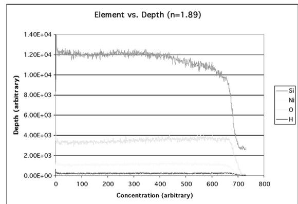
Fig. 14: SIMS profile of silicon, oxygen and nitrogen through the depth of a  $n=1.89$  silicon oxynitride film.
