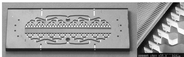
Fig. 22: Photograph of cross-flow microreactor for catalyst testing (Felice Frankel) and electron micrograph of catalyst channel detail.
