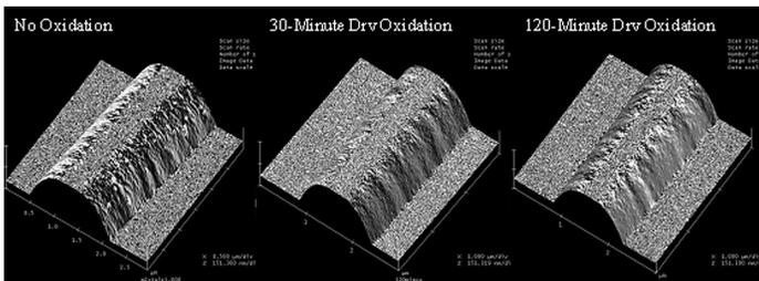
Fig. 10.: AFM images of silicon waveguides, the left image is as-fabricated whereas the center and right waveguides have undergone 30 and 120 minutes of dry oxidation and subsequent oxide etch respectively.
