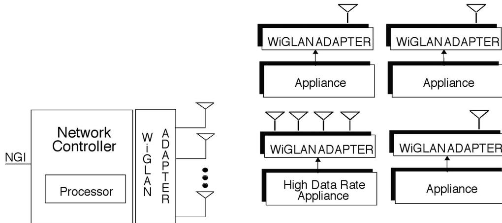
Fig. 14: Wireless Gigabit Local Area Network
