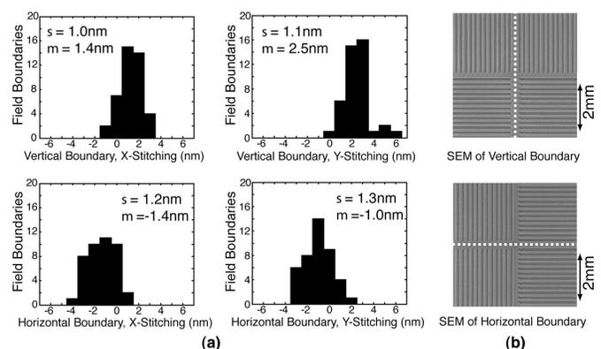
Fig. 5: (a) Histograms showing x- and y-stitching measurements at all 84 field boundaries of 49 stitched fields. Spatial-phase locking has reduced the standard deviation of the stitching errors to below 1.3 nm. (b) Sample 200-nm period stitched grating patterns. The dashed line indicates the field boundary.
