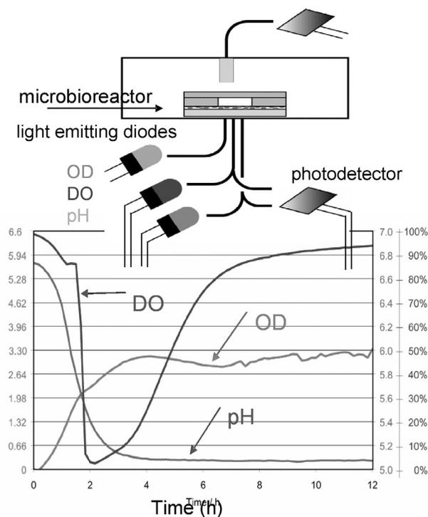
Fig. 10: (Top) Schematic of microbioreactor with optical, on-line monitoring of optical density (cell concentration), Dissolved Oxygen (DO), and pH. (Bottom) Example of data obtained with on-line sensors.
