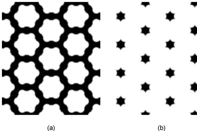
Fig. 24: Schematics of the improved 3D PBG design. (a) The "hole" layer. (b) The "rod" layer.
