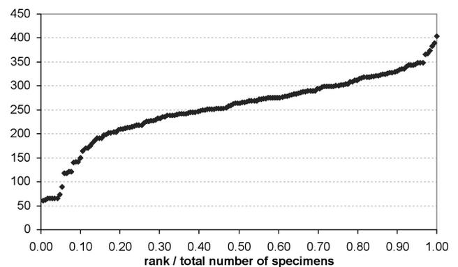
Fig. 48: Bond toughness data for specimens bonded at 300°C and 73 MPa (on gold).
