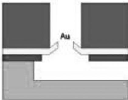
Fig. 38: Folding Au layers into sidewall
