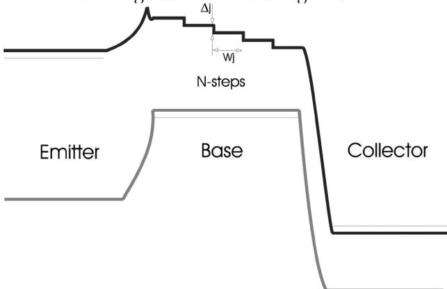
Fig. 26: Energy band diagram of an HBT with stepwise base. The energy drop  $\Delta$  at each step is slightly greater than the LO-phonon energy (36 meV) in GaAs. Thus, electrons encounter very fast LO-phonon emission scattering (with a time  $\sim 0.1$  ps) when they go over the edge of a step. Consequently, backward diffusion is significantly reduced and forward diffusion is enhanced.
