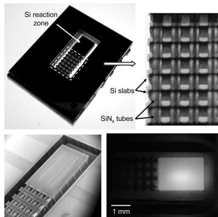
Fig. 28: Micro fuel processor. Photograph of device (top) with close-up of suspended tube/slab structure. Electron micrograph of reactor/heat exchanger section (lower left). Glowing reactor during autothermal combustion and ammonia cracking (Note, that the tubes and surroundings remain at low temperatures).
