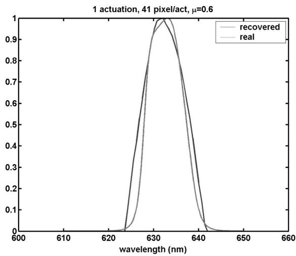
Fig. 3: Spectrum recovered using deconvolution VS real spectrum of an interference filter.
