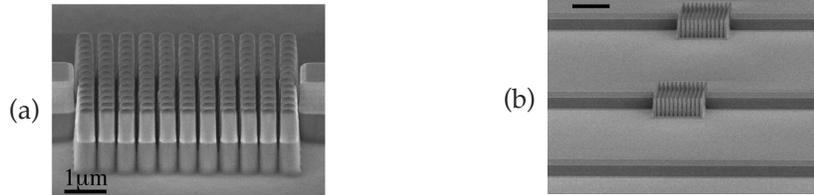
Fig. 53: a) Side view SEM of a bulk photonic crystal etched in GaAs/AlGaAs using  $\text{BCl}_3/\text{He}$  plasma. The AlGaAs is oxidized into  $\text{Al}_x\text{O}_y$ . The period is 500nm and the diameter of the pillars is 300nm. The input and output waveguides are 1.5 $\mu\text{m}$  wide. b) Photonic crystal devices on a single chip. The design contains a straight waveguide for normalization purposes.
