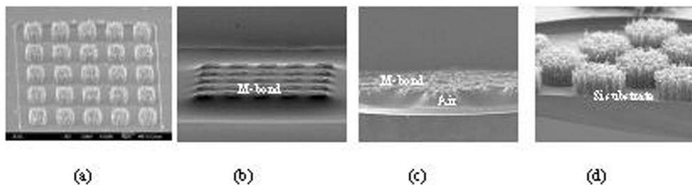
Fig. 56: SEM images of the CNTs (a) Grown CNTs, (b) Filled with M-bond, (c) Released M-bond pellet by XeF<sub>2</sub> (not planarized) and (d) CNTs after filler removal by O<sub>2</sub> plasma (not planarized)
