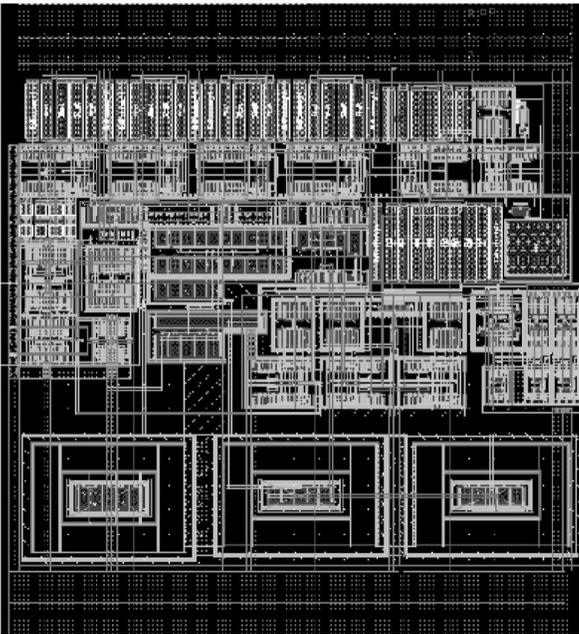
Fig. 37: Third generation clock receiver circuit.
