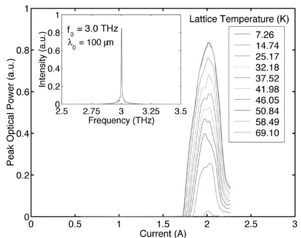
Fig. 45: Power-current relations of a laser device using metal waveguide for mode confinement, measured at heat sink temperatures up to 70 K. Inset: Emission spectrum taken at a bias voltage 11.4 V and current 1.8A. The spectrum is single-mode, and the wavelength is among the longest achieved in QCLs.
