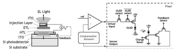
Fig. 19 (left) An OLED pixel integrated with a “smart” si active matrix driver. The si photodetector monitors the intensity of the OLED pixel during the on state and provides feedback to the driving circuit to keep the light output intensity constant as the device efficiency changes with operation. (Right) pixel design in integrated circuit implementation
