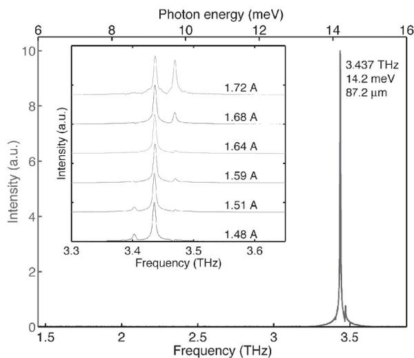
Fig. 42: Emission spectrum above threshold biased at 1.64 A at 5K heat sink temperature. The inset shows an expanded view of spectra at various bias points, offset for clarity.
