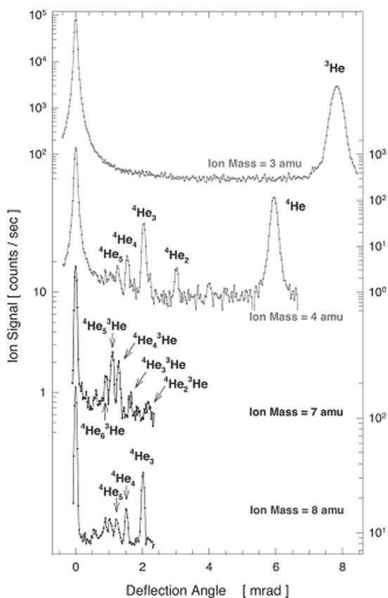
Fig. 62: Non-destructive mass separation of small mixed-isotope helium clusters. These results were obtained by Peter Toennies, et al, at the Max-Planck Institute in Goettingen, Germany, using free-standing, 100 nm-period gratings made in the NSL at MIT.
