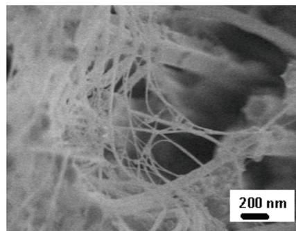
Fig. 15: Gold nano-wires (~20nm) grown by halide reduction in nano-porous alumina template. Template chemically etched to expose nano-wires.
