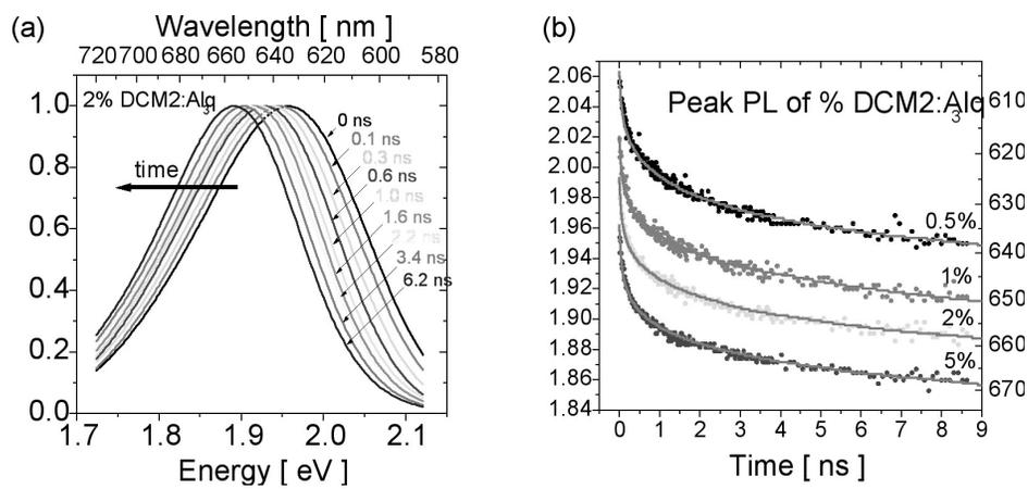
Fig. 30: (a) Normalized DCM2 PL spectra, following ultrafast excitation; (b) Evolution of peak PL of DCM2 doped in films of Alq<sub>3</sub>. Grey lines denote simulation results optimized for each data set.
