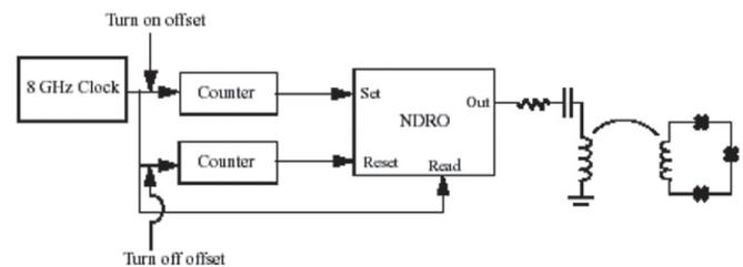
Fig. 24: An RSFQ Variable Duty Cycle Oscillator.
