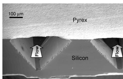
Fig. 23: Cross-sectional scanning electron micrograph of the reaction microchannels.
