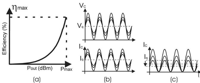
Fig. 17: (a) Typical Efficiency Curve (b) Fixed-Bias Waveforms (c) Adaptive Current Biasing
