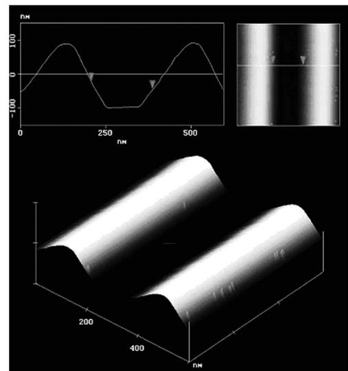
Fig. 58: AFM image of nano-imprinted grating. Profile is far from ideal at this stage.
