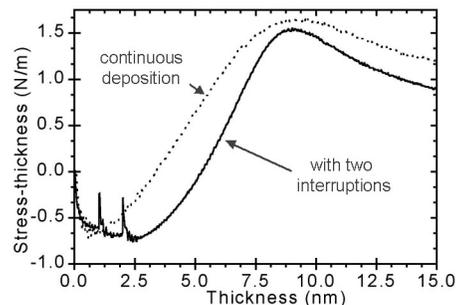
Fig. 23: The onset of coalescence occurs at a higher film thicknesses when growth is interrupted, presumably due to island coarsening during the interruptions.
