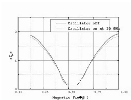
Fig. 3: This graph shows the switching current of the DC SQUID while the oscillator is off and while it is on. The current is clearly suppressed by turning the oscillator on. This oscillator has been fabricated and testing has begun. Although it is too early to comment on its effect on the qubit, it is clear that the oscillator is producing sufficient signal to suppress the current of the dc SQUID magnetometer used to measure the qubit's state, as shown in Figure 3.
