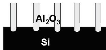
Fig. 37: To make a film of anodized alumina containing a regular arrangement of pores, we start by patterning a silicon substrate with a square array of inverted pyramids, using interference lithography. The substrate is then coated with Al, which conforms to the surface topography. The aluminum film is then anodized (at 80V in this case), and the indentations in the aluminum act as nucleation sites for pores. A film of porous alumina grows containing a square array of pores.
