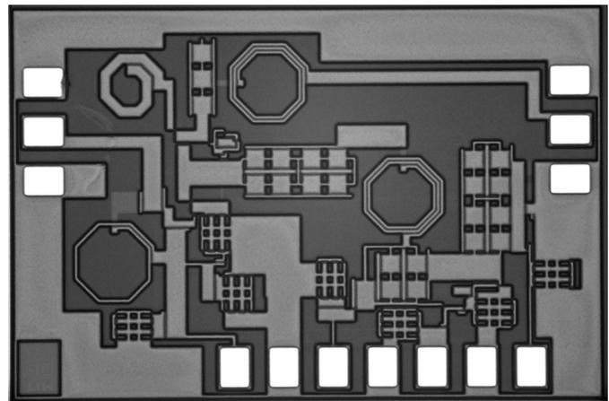
Fig. 15: Die photo of an LNA with notch filter for image rejection on IBM BiCMOS 7HP process.
