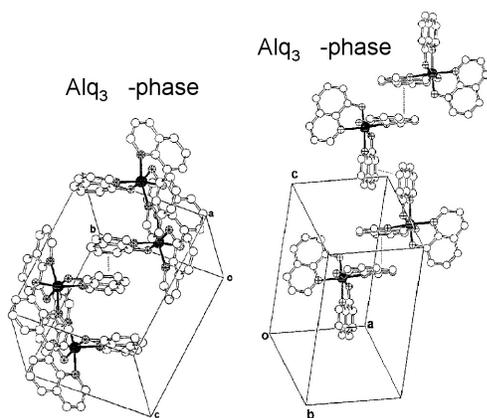
Fig. 46:  $\alpha$  and  $\beta$  crystal forms of  $\text{Alq}_3$ . (from Brinkmann, et al., *J. Am. Chem. Soc.*, **122**, 5147 (2000)).
