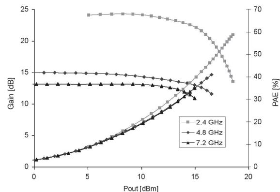
Fig. 15: Gain and Power-Added Efficiency (PAE) as a function of output power for a  $300\ \mu\text{m}$  wide NMOS in a  $0.25\ \mu\text{m}$  technology at three different frequencies.
