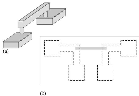
Fig. 3: A second structure for characterization of interfacial electromigration of Cu. A via-to via metal 2 test line connected to larger metal 1 lines, connected to bond pads. (a) Conventional dual-damascene processing through CMP of metal 2 is carried out at Sematech. Metal 2 surface treatment and passivation, and the rest of the test structure processing, are carried out at MIT.
