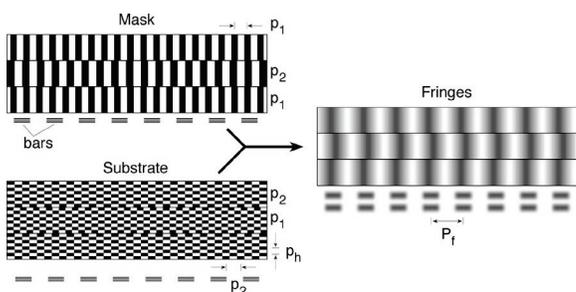
Fig. 21: Schematic of ISPI aligning marks. Fine alignment is detected using the spatial phase relation of middle to outer fringe sets. Errors from camera-mark rotation are removed by phase comparison of outer fringe sets. Spatial-phase ambiguity is eliminated by comparing the phase between bar arrays on the mask and wafer, as well as between bars and fringes.
