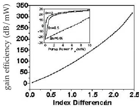
Fig. 3: Device gain efficiency versus index difference  $\Delta n$  for a 1 m long waveguide amplifier with  $10^{20}$   $\text{Er}/\text{cm}^3$  optically active. Inset: plot of device gain  $\gamma_d$  vs. optical pump power  $P_p$  shows an increasing slope with higher  $\Delta n$ . The slope of this plot gives the device gain efficiency.
