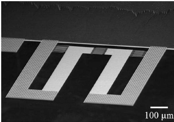
Fig. 17: Scanning electron micrograph of a differential microcantilever stress sensor.
