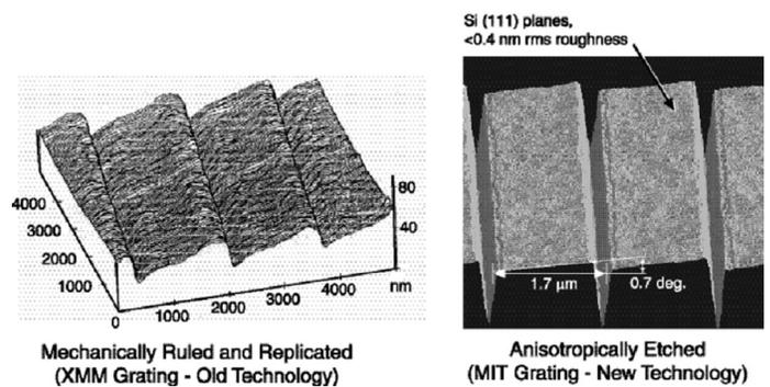
Fig. 57: (a) An AFM image of a traditional mechanically-ruled and replicated X-ray reflection grating (Bixler et al., Proc. SPIE 1549, 420-428 [1991]). Note the rough, wavy grating surfaces that lead to poor diffraction performance. (b) An AFM image of a blazed X-ray reflection grating fabricated by anisotropic etching of special off-cut (111) silicon wafers. Note the improvement of grating surface flatness and smoothness, leading to significantly improved performance.
