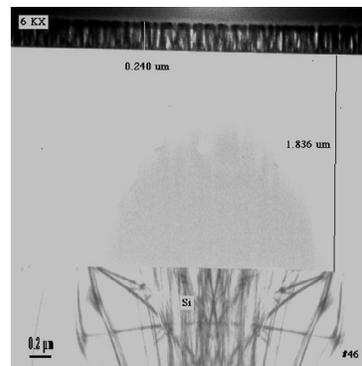
Fig. 15: TEM micrograph of  $n=1.89$  silicon oxynitride film.
