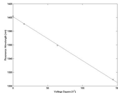
Fig. 8: The resonance wavelength shift with voltage square at 1.402 $\mu\text{m}$ .
