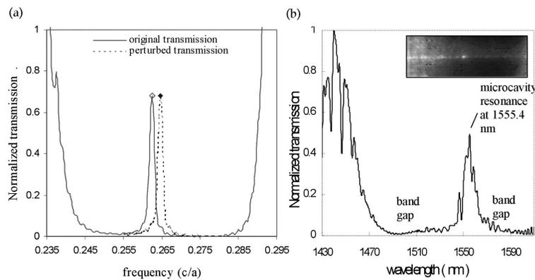
Fig. 54: (a) Computed transmission shift through perturbation theory in the photonic band gap, (b) Measured static microcavity resonance with  $Q$  of 159. Inset: top view of microcavity waveguide in transmission.
