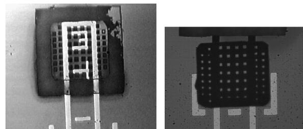
Fig. 53: Membrane flap before folding (left) and after folding to 180 degrees (right). Note the alignment tolerance achieved in folding (alignment fiducials are 50µm wide).
