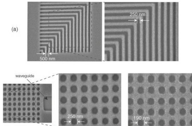
Fig. 14: Scanning electron micrographs of patterns exposed with our continuous-scan 0.9 NA UV-ZPAL system operating at  $\lambda = 400\text{nm}$ . (a) Dense nested Ls, (b) 2D photonic bandgap structures with 500 nm period, (c) 2D photonic bandgap structures with 360 nm period.
