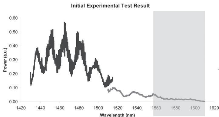
Fig. 55: Initial experimental data of a bulk photonic crystal with 7 columns and 13 rows of dielectric pillars. The darker grey data is for a tunable laser source of 1410nm-1510nm. The lighter grey data is for source wavelength of 1510-1610nm. The shaded region indicates the band gap covered by the tunable range. The band gap extends to 1725nm.
