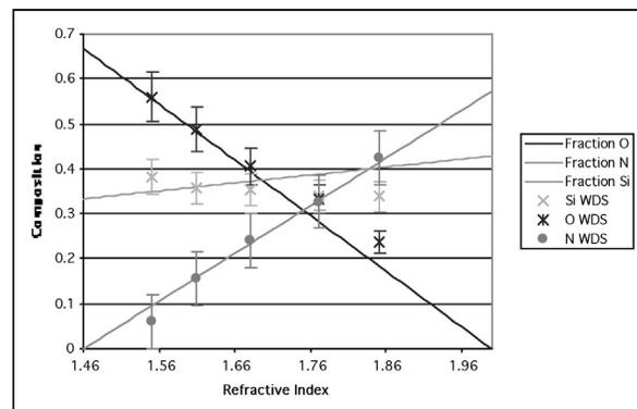
Fig. 13: Data points show atomic fraction as determined by WDS. Solid lines are predictions based on a silica/silicon nitride alloy.
