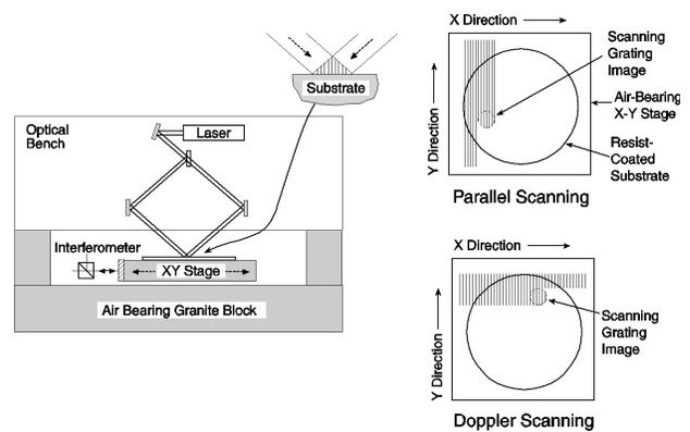
Fig. 33: Schematic of the Scanning-Beam-Interference-Lithography (SBIL) system under development in the SNL. A pair of narrow, low-distortion beams overlap and interfere at the substrate, producing a small grating “image.” The substrate is moved under the beams, writing a large area grating. Tightly overlapped scans ensure a uniform dose.
