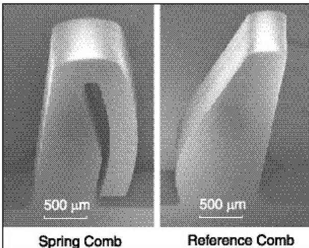
Fig. 63: Electron micrographs of silicon micro-combs. Teeth are  $\sim 500 \mu\text{m}$  wide. a) Spring comb. b) Reference comb.
