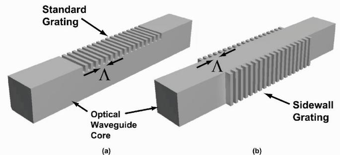
Fig. 40: Two possible configurations for physically patterned Bragg gratings in optical waveguides. (a) Bragg grating patterned in the top of the high-index core. (b) Bragg grating patterned in the sides
