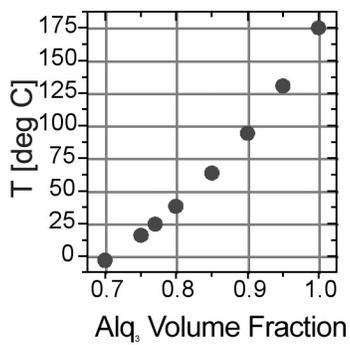
Fig. 52: Change in the glass transition temperature of Alq<sub>3</sub> upon incorporation of chloroform.
