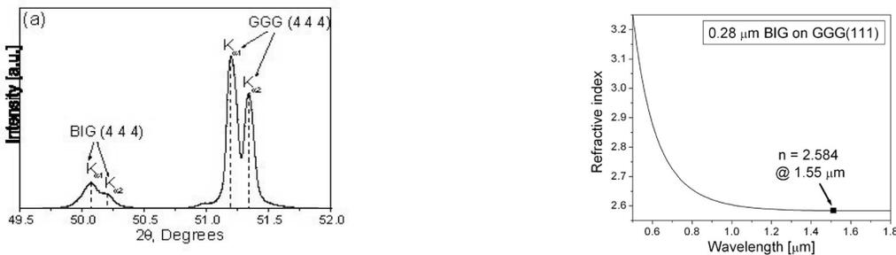
Fig. 16: Left: X-ray diffraction spectra from 300 nm thick BIG film deposited on (111) GGG (gallium gadolinium garnet) single crystal substrate, illustrating epitaxial growth. Right: Refractive index vs wavelength, measured from ellipsometry data, assuming zero absorption, for a 280 nm thick BIG film on (111)GGG.
