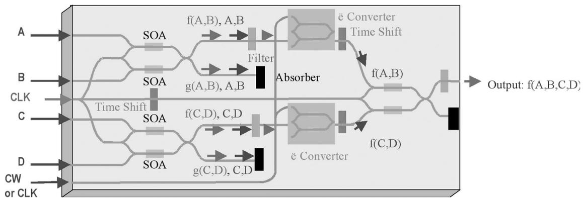
Fig. 35: Three unit cells cascaded on a chip with additional components that enable proper signal processing.
