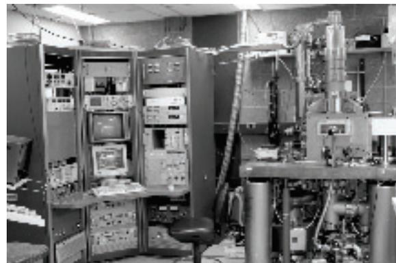
Fig. 1: Photograph of the VS-26 scanning-electron-beam lithography system.
