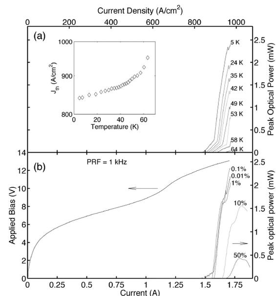
Fig. 43: (a) Emitted light versus current at various temperatures. The inset is a semi-log plot of the threshold current density  $J_{th}$  as a function of temperature. (b) Applied bias voltage and peak optical power versus current, collected at various duty cycles.
