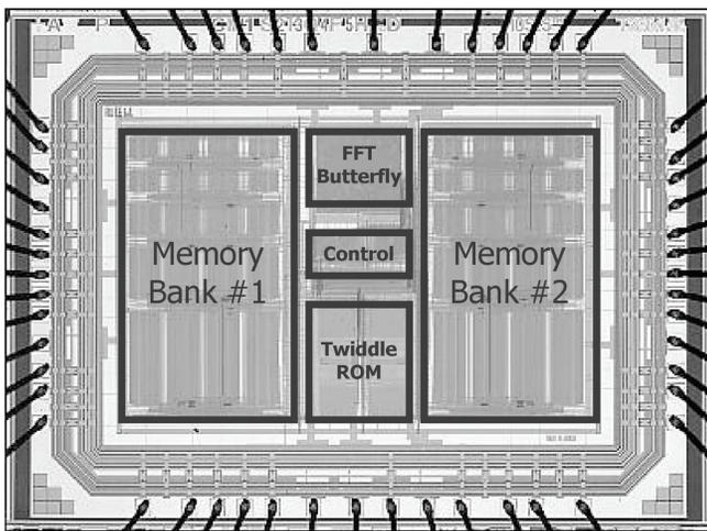
Fig. 4: Die photograph of the Energy-Scalable RVFFT.
