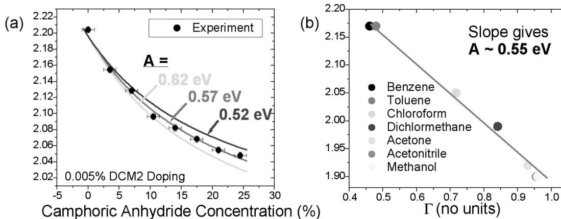
Fig. 29: (a) Fits of OLM theory to observed evolution of DCM2 peak PL energy; (b) OLM fit to DCM2 PL data in solution.
