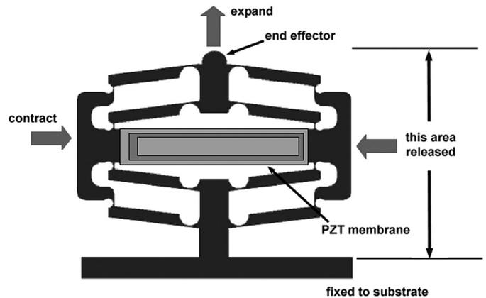
Fig. 44: A Bow Actuator Design for Strain Amplification
