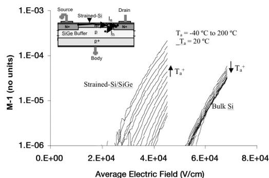
Fig. 7: Impact ionization as a function of average field and temperature for bulk and strained-Si/SiGe samples.  $M = (I_s + I_b)/I_b$ .  $M-1$  increases with temperature in the strained-Si samples, but decreases with increasing temperature in the bulk samples. Inset shows test structure.
