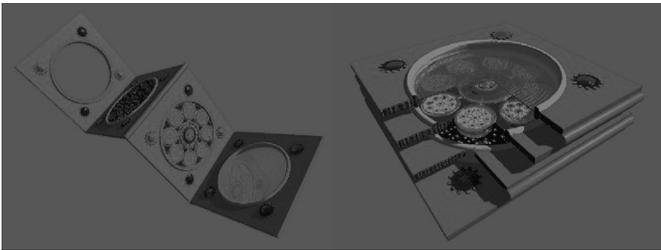
Fig. 55: An example of a heterogeneous system created through folding. Optics, microfluidics, nanopatterning, and circuitry are fabricated within the plane and then folded into one complete functional system.
