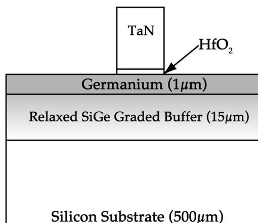
Fig. 5: Layer structure of epitaxial germanium-on-silicon. The 1 µm germanium device layer was grown on a relaxed SiGe graded buffer using UHV-CVD.
