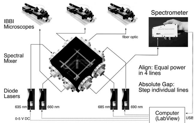
Fig. 24: A Closed-Loop Variable Bandwidth (CLVB) light source provides optimum illumination for both aligning and gapping. A single laser line is used for gapping, but a broad spectrum using multiple lasers is ideal for aligning. The spectrometer monitors wavelength when gapping, and relative intensities when aligning.
