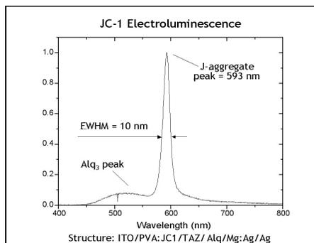
Fig. 36: Electroluminescence spectrum of a JC-1 OLED.
