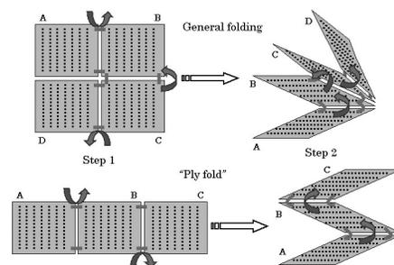
Fig. 52: Examples pre-fabricated thin 2D membranes folded into 3D structures in a two-step process. Black dots denote surface features nanofabricated on the membrane surface, and grey lines denote "hinges."
