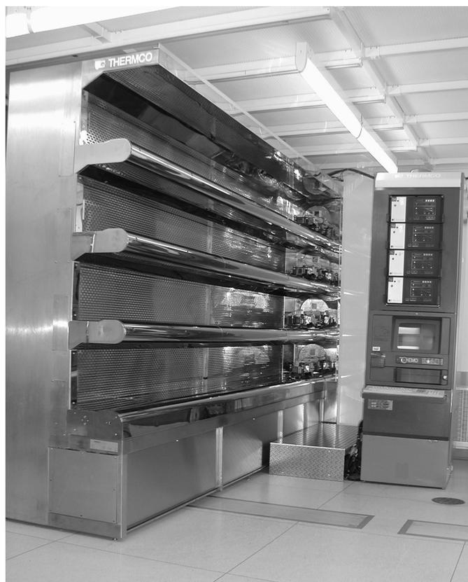
*Thermco Furnaces - cleanroom view, ICL*
