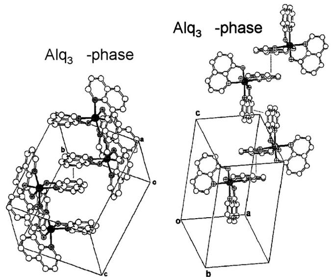
Fig. 22.  $\alpha$  and  $\beta$  crystal forms of Alq<sub>3</sub>. (from Brinkmann, et al., *J. Am. Chem. Soc.*, 122, 5147 (2000)).
