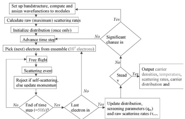
Fig. 46: Flow chart of our ensemble Monte Carlo simulation scheme.
