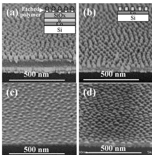
Fig. 38: Cross-section SEM micrographs of (a) Block copolymer lithographic template on the multilayer film. (b) W hard mask (dots) on continuous Co film. (c) Co dots after Ar ion milling. (d) Co dots after Ne ion milling.
