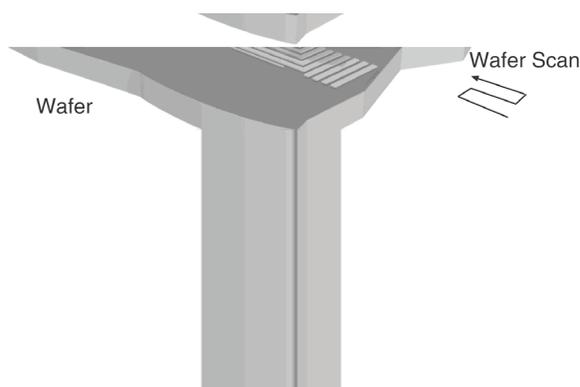
Fig. 6: Schematic of Zone-Plate-Array Lithography (ZPAL). An array of Fresnel zone plates focuses radiation beamlets onto a substrate. The individual beamlets are turned on and off by upstream micromechanics as the substrate is scanned under the array. In this way, patterns of arbitrary geometry can be created in a dot-matrix fashion. The minimum linewidth is equal to the minimum width of the outermost zone of the zone plates.
