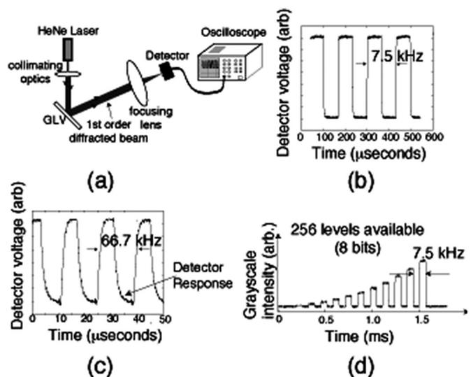
Fig. 11(a): Schematic of the experimental setup for testing the data delivery system for ZPAL. (b) The GLV operating at 7.5 kHz, the required speed for our prototype system. (c) The GLV operating at 66.67 kHz, corresponding to a 1Gbit/sec data rate. (d) Grayscale at 7.5 kHz
