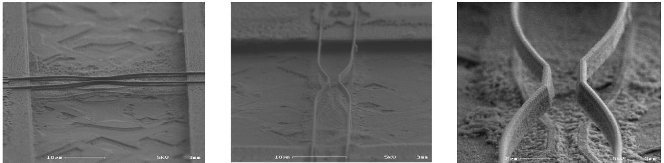
*Fig. 38: SEM images of a fabricated ONEMS device in a gallium arsenide-based material system with an exponentially tapered geometry.*
