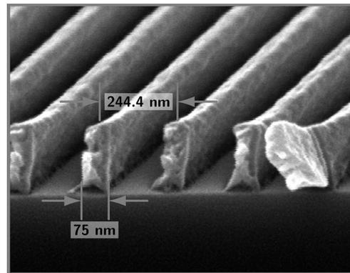
Fig. 19: Example of X-ray lithography done with the JMAR laser plasma X-ray source.
