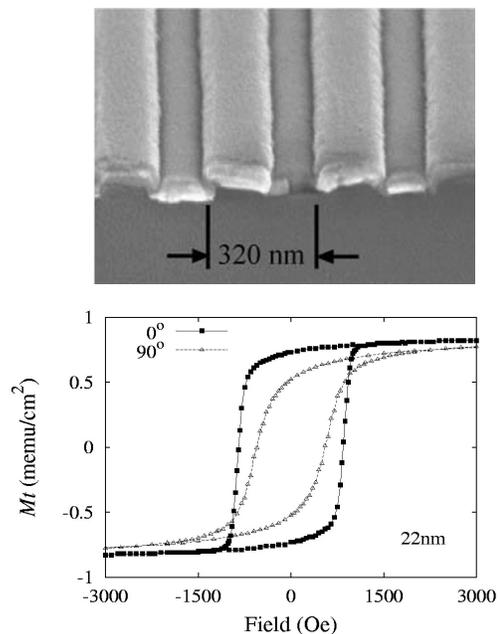
Fig. 18: Top: Example of a film sputtered over a substrate with 320 nm period grooves. Bottom: Magnetic hysteresis loops from a sample of Cr/CoCrPt sputtered onto a substrate with 200 nm period, 22 nm deep grooves. Coercivity, remanence and squareness are higher parallel to the grooves (filled symbols) compared to perpendicular to the grooves (open symbols).
