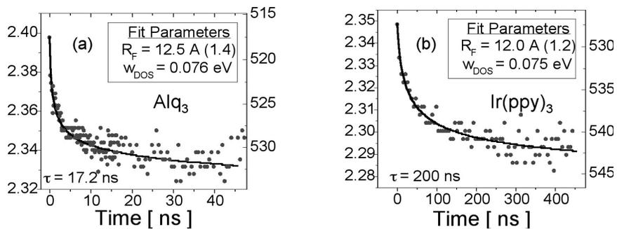
Fig. 31: (a) Evolution peak PL of Alq<sub>3</sub> with simulation fit; (b) evolution of peak PL of Ir(ppy)<sub>3</sub> with simulation fit.
