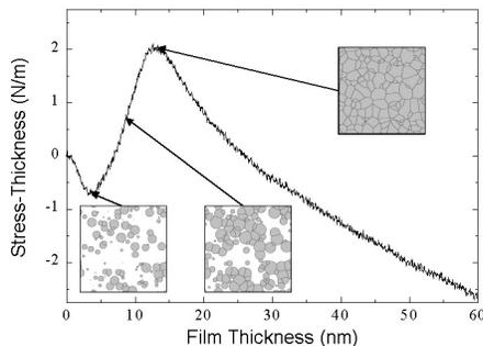
Fig. 20: Stress-thickness product measured during deposition of a Cu film. The stress is compressive as islands nucleate and grow, becomes tensile as islands coalesce, reaching a maximum when the film is continuous, and becomes compressive at higher thicknesses.
