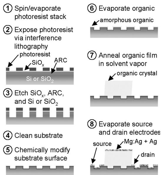
Fig. 48: Fabrication steps, beginning with the nano-lithography, necessary to form oriented crystals of  $Alq_3$ .
