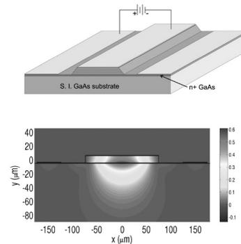
Fig. 41: Schematic of the THz laser ridge structure, calculated two-dimensional mode profile using FEMLAB (on the left), and one-dimensional mode profile, confinement factor, and waveguide loss (on the right).
