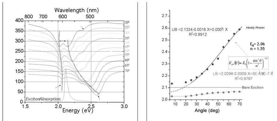
Fig. 35: Angle dependent reflectivity and dispersion curve of a silver mirror metal microcavity containing J-aggregates of JC-1 in polyvinyl alcohol.
