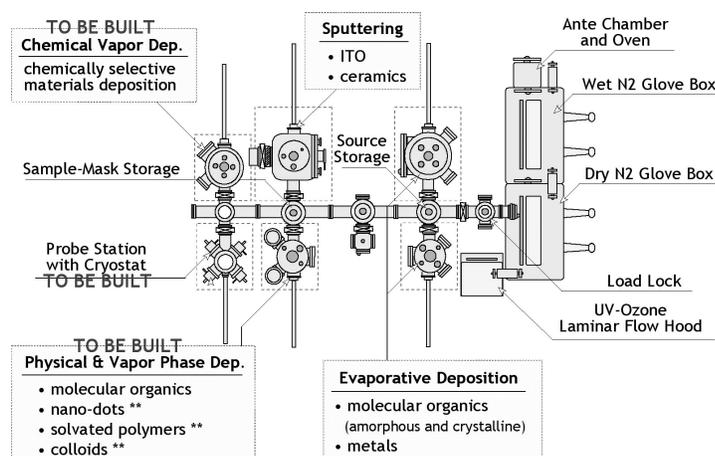
Fig. 10: Integrated Materials Growth System. Both present and projected chambers are indicated. Projected chambers and chambers in construction are labeled as "TO BE BUILT".
