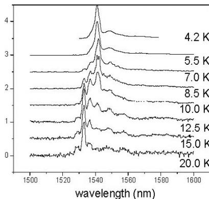
Fig. 4: Low temperature photoluminescence study of  $\text{Er}_2\text{O}_3$ . Observations indicate the presence of three optical light-emitting centers, correlated by X-ray diffraction with the formation of three crystal phases.
