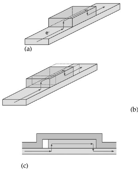
Fig. 4: Void growth causes a gradual resistance increase during elec-
