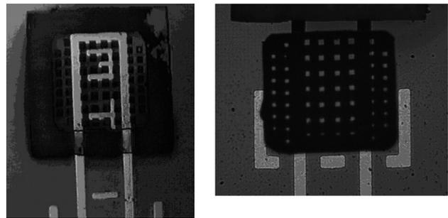
denote surface features nanofabricated on the membrane surface. Fig. 65: Membrane flap before folding (left) and after folding to 180 degrees (right). Note the alignment tolerance achieved in folding. (Alignment fiducials are 50mm wide).
