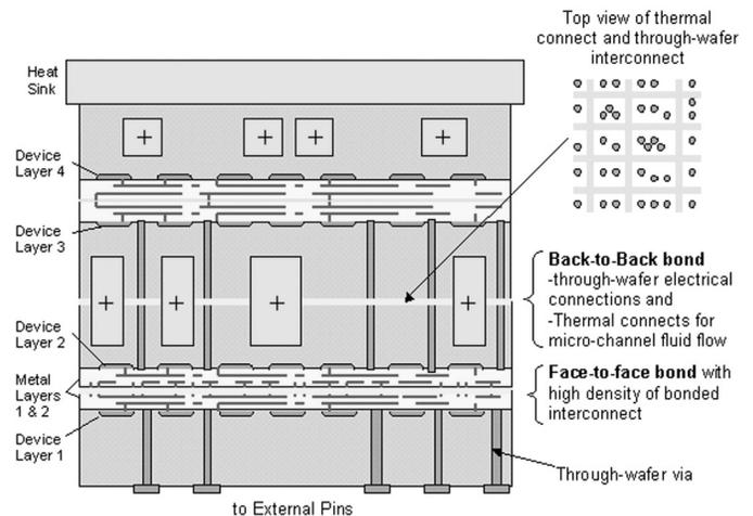
Fig. 41: Thermal management in a 3D IC. Here the 3D IC is a 4-wafer bonded stack.
