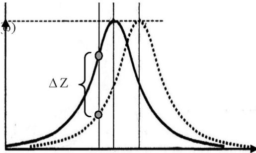
Fig. 41: Illustration of the shift in resonant frequency  $\Delta\omega_0$  upon a change in the qubit state. During the measurement, one biases the operating frequency at  $\omega_{sb}$  and senses a change in impedance  $\Delta Z$ , which in turn can be retrieved as a voltage signal.
