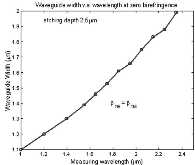
Fig. 56: Calculation of zero birefringence for different waveguide widths and measuring wavelengths (2.5  $\mu\text{m}$  etch depth for all waveguides)
