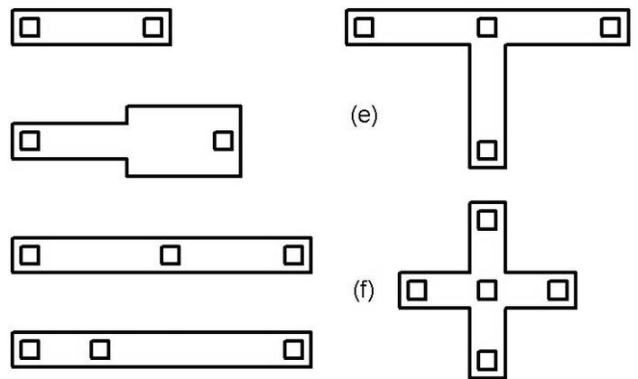
Fig. 24: Test structures used for development of circuit-level reliability assessment methodologies for Cu based interconnects: (a) 'i' structure with 2 terminals, (b) 'i' structure with a width transition, (c) symmetric 'dotted-i' structure with 3 terminals, (d) asymmetric 'dotted-i' structure, (e) 'T' structure with 4 terminals, and (e) '+' structure with 5 terminals.
