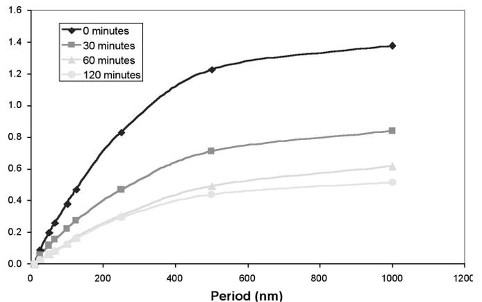
Fig. 11: Plot of waveguide roughness amplitude versus roughness period for different oxidation times.
