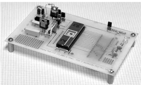
Fig. 23: Circuit board including IC in  $0.18\mu\text{m}$  CMOS process.
