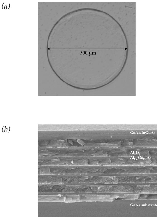
Fig. 34: (a) Nomarski image of fully-oxidized SBR. (b) SEM image of SBR cross-section showing 67 nm GaAs, 40nm InGaAs, 67 nm GaAs absorber with a 7 pair Al<sub>x</sub>O<sub>y</sub>/Al<sub>0.3</sub>Ga<sub>0.7</sub>As mirror stack (~180nm/92nm).
