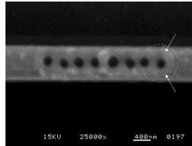
Fig. 56: SEM image of holes drilled into a Si line on oxidized Si. A femtosecond laser was used.
