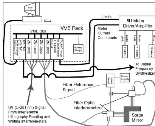
Fig. 35: Schematic of SBIL system control architecture. The system utilizes a frequency stabilized HeNe laser ( $\lambda=632.8\text{ nm}$ ) and heterodyne interferometry to measure substrate position, and argon ion laser ( $\lambda=351.1$ ) heterodyne interferometry to measure image fringe phase. Phase error signals are processed by an IXTHOS 4x167 MHz DSP board which then drives the stage DC motors and the RF digital frequency synthesizer controlling the fringe-locking AO modulators.
