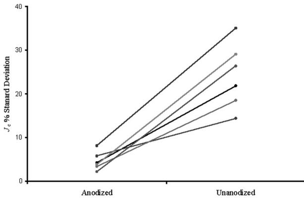
Fig. 12: Comparison of cross-wafer critical-current-density standard deviation of anodized/unanodized wafer pairs. The wafers shown have  $I_c$  values ranging between  $102\text{A}/\text{cm}^2$  and  $103\text{A}/\text{cm}^2$ . Lines connect data points on wafers whose trilayers were deposited together.
