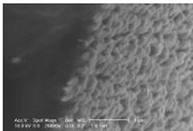
Fig. 39: SEM picture of side wall Au
