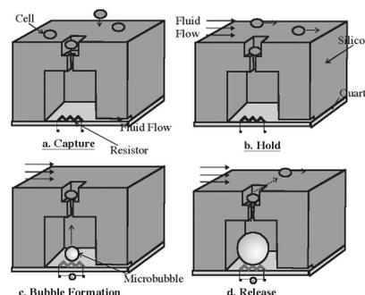
Fig. 13: Schematic of microbubble bioparticle actuator. (a) A small backflow draws particle into capture well. (b) A bulk flow sweeps uncaptured particles away. (c) The platinum heater is turned on, and a vapor bubble begins to form in the bubble chamber. (d) The volume expansion of the bubble creates a jet of fluid that releases the particle from the capture chamber and is entrained in the bulk flow.
