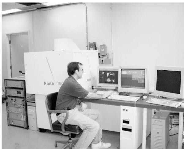
Fig. 2: The Raith-150 electron-beam lithography system. This tool provides sub-20-nm patterning resolution, and pattern-placement accuracy  $\sim 1\text{nm}$  via spatial phase locking. The operator is graduate student J. Todd Hastings.
