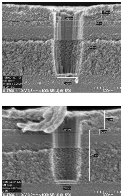
Fig. 3: 0.25  $\mu\text{m}$  via cross sections for IPS  $c\text{-C}_4\text{F}_8$  process of comparison for LKD film. BARC BT: 800 W Outer, 400 W Inner, 300 W Bias, 4 mT, 5 sccm  $c\text{-C}_4\text{F}_8$ , 10 sccm  $\text{O}_2$ , 100 sccm Ar, 15s; SiCN BT: 1000W Outer, 200 W Inner, 300 W Bias, 15 sccm  $c\text{-C}_4\text{F}_8$ , 5 sccm  $\text{O}_2$ , 100 sccm Ar, 25s; Main Etch: 1540 W Outer, 260 W Inner, 1800 W Bias, 7 mT, 8 sccm  $c\text{-C}_4\text{F}_8$ , 100 sccm Ar, 60s. (IPS-LK3-XLK)
