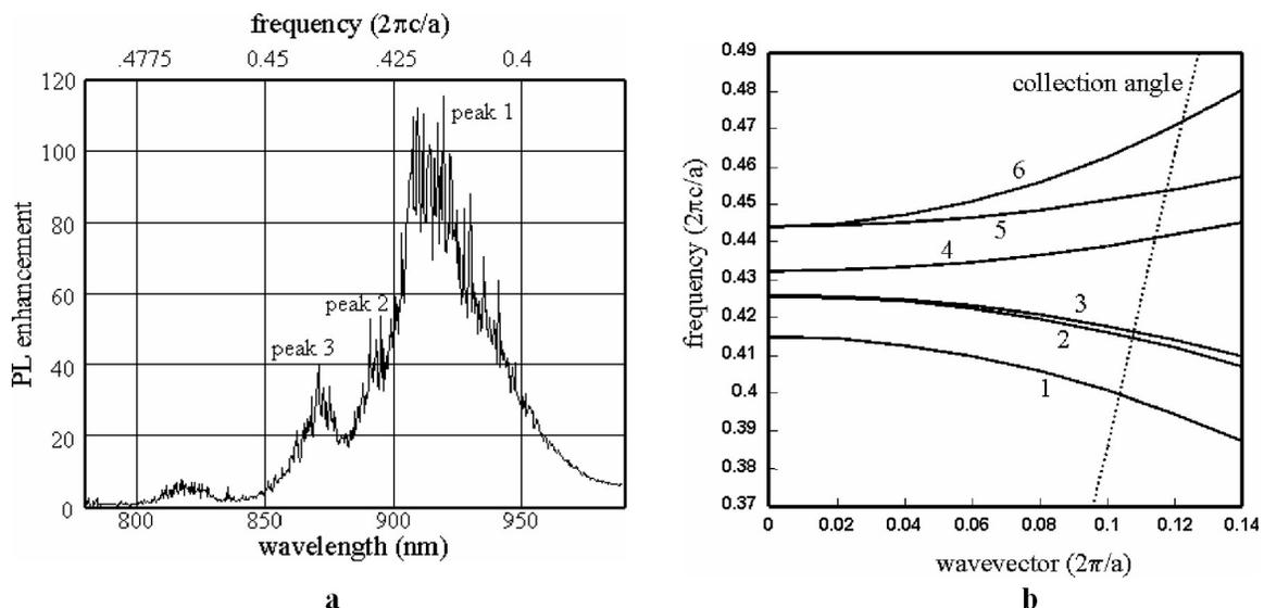
Fig. 20: a) PL enhancement spectrum from PC structure. b) Calculated photonic band structure near G point.
