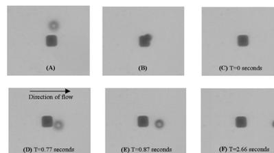
Fig. 14: Microbubble bioparticle actuator in operation. In (A) and (B), a  $10\mu\text{m}$  polystyrene bead is drawn into the capture well where it is held against a bulk flow in (C). In (D), the bead is released by a jet created by a bubble in the chamber below. In (E) and (F), the bead is entrained in the bulk flow.
