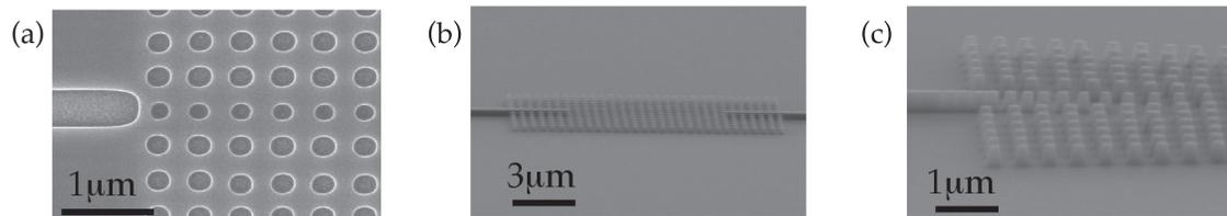
Fig. 27: Top view SEM image of (a) the first coupling design after electron-beam lithography, (b) the second coupling design after a hard mask etch, and (c) the third coupling design after a hard mask etch.
