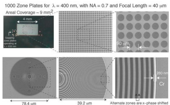
Fig. 8: Large zone plate arrays can be readily fabricated with our novel process that requires a single lithography exposure and no etching, even for the case of phase zone plates. Top-left: Optical micrograph showing an array containing over 1,000 zone plates with an areal coverage of 9 mm<sup>2</sup>. Bottom-right: Detail of the outermost zones. The duty-cycle is very close to 50%, and the phase shift between alternate zones was controlled to about 1%.
