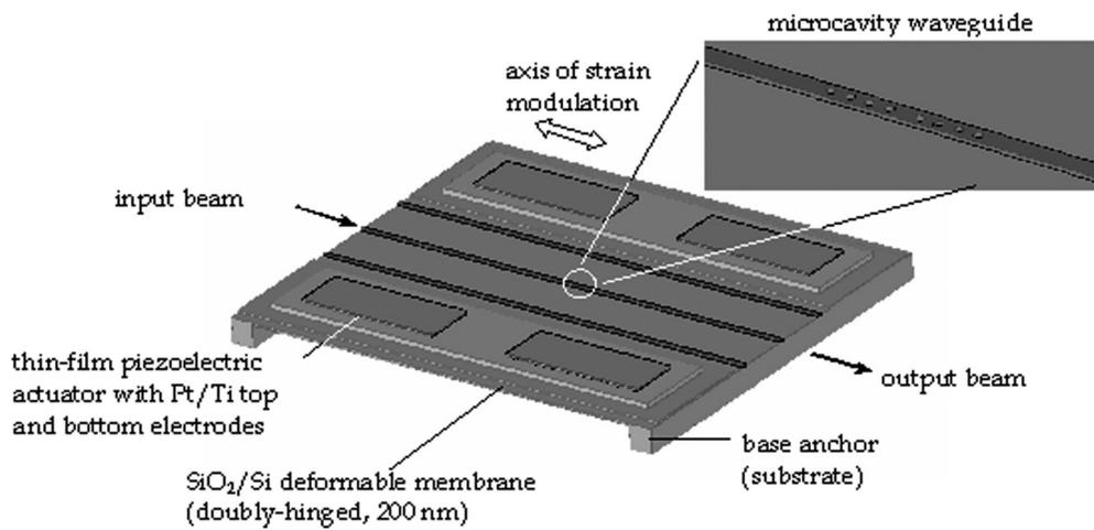
Fig. 53: Device schematic of the tunable photonic-bandgap microcavity waveguide, with strain modulation via thin-film piezoelectric actuators on the deformable membrane.
