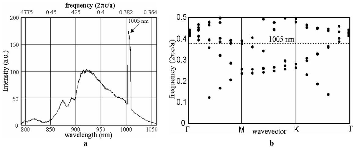
Fig. 21: a) Lasing spectrum. b) Calculated band structure showing band folding near M point.
