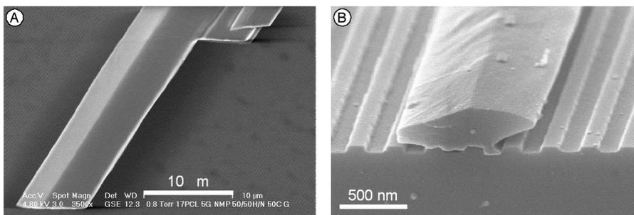
Fig. 49: SEM micrograph of two  $Alq_3$  crystals. (A) is a top view of one end of a several micron wide needle, and (B) shows the cross section of a smaller needle (the substrate was cleaved in the middle of the needle).
