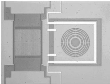
Fig. 54: Top view of tunable grating (left) and static Fresnel zone plate (right) before folding.
