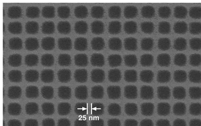
Fig. 60: Scanning electron micrograph of a free-standing 100 nm period grid in a silicon nitride membrane of area 500 micron by 5 mm. Such grids are used in experiments to separate out Helium trimers from other clusters.
