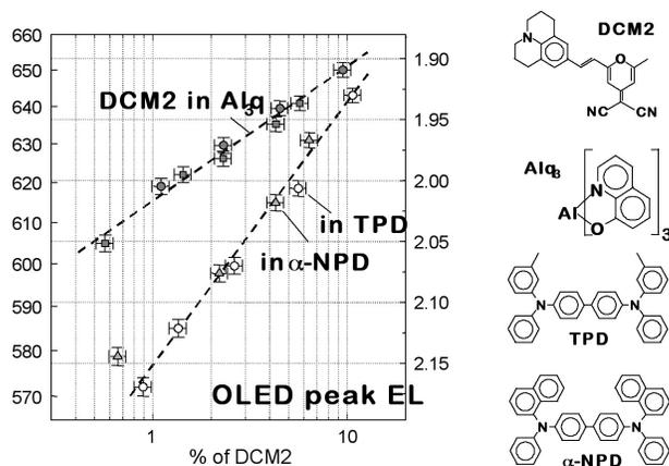
Fig. 26: (a) Evolution of peak PL spectra of DCM2 in films of Alq<sub>3</sub>, TPD and α-NPD.; (b) chemical structures of molecules used in this work.”.
