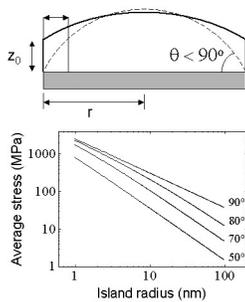
Fig. 12: Effects of the equilibrium island-substrate contact angle on the coalescence stress, as indicated by finite element analyses.
