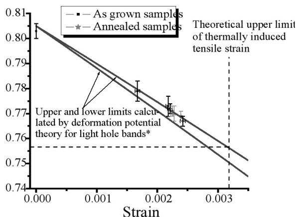
Fig. 8: Direct Ge bandgap vs. strain for several different as grown and annealed samples.
