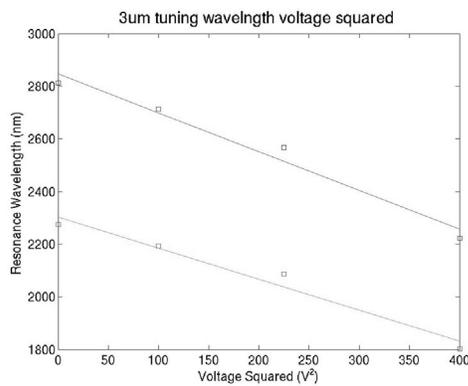
Fig. 9: First demonstration of an optical filter with a continuous tuning wavelength range of  $2 \mu\text{m}$ .
