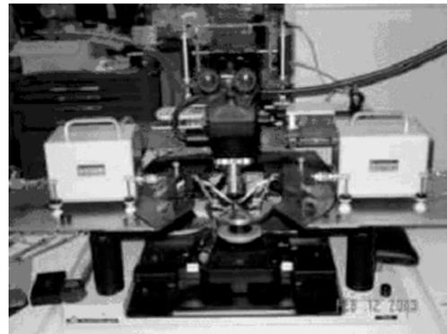
Fig. 14: Probe station and tuners of a new load-pull system assembled at MTL to carry out on-wafer RF power characterization.
