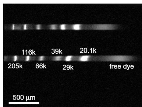
Fig. 9: SDS-PAGE separation of six proteins in 12% gel (acrylamide : bis-acrylamide = 37.5:1), also containing 0.1% SDS and 0.2% photoinitiator. The gel buffer was 0.375M Tris-Cl (pH=8.6). The rightmost peak in the channel is due to the Bromophenol blue dye added to the sample. The width of dye band is much larger than other protein bands, suggesting no stacking effect for small dye molecules.
