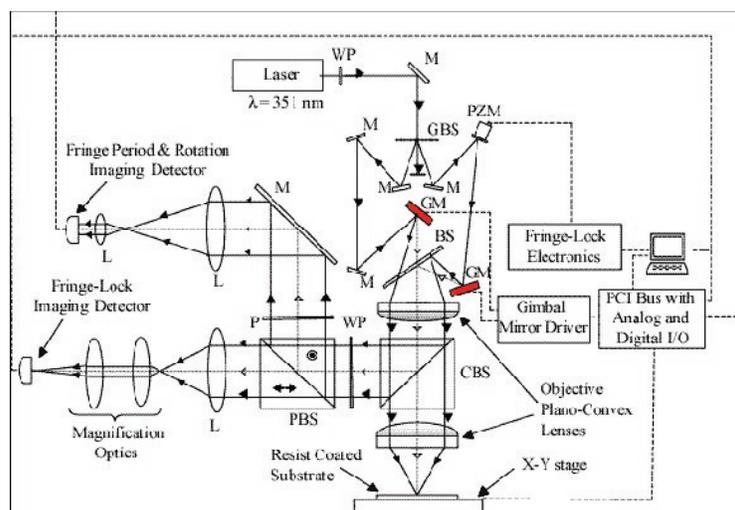
Fig. 12: Experimental diagram of variable-period scanning-beam interference-lithography system. M: mirror, L: lens, P: polarizer, GM: gimbal mirror, WP: wave plate, BS: beam splitter, PZM piezo-actuated mirror, GBS: grating BS, CBS: cubic BS, PBS: polarizing BS.
