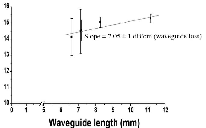
Fig. 2: Waveguide loss for  $1.5\mu\text{m}$   $1.5\mu\text{m}$  PECVD-deposited SiON waveguide ( $\Delta n=0.05$ , unannealed)
