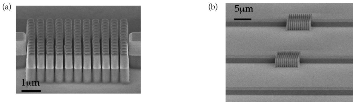
Fig. 28: (a) Side view SEM image of a bulk photonic crystal. The period is 500nm and the diameter of the pillars is 300nm. The input and output waveguides are 1.5μm wide. (b) Photonic crystal devices on a single chip. The design contains a straight waveguide for normalization purposes.
