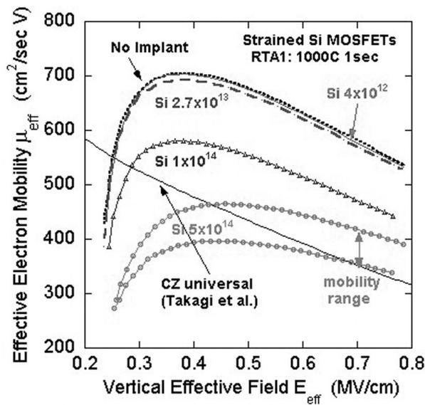
Fig. 8: The effective mobility  $\mu_{eff}$  vs  $E_{eff}$  for the strained Si devices with RTA1 (1000 C for 1 sec) and different implantation conditions.
