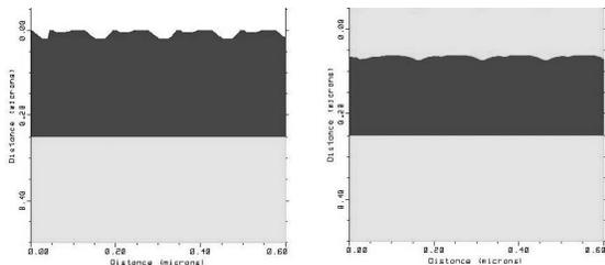
Fig. 12: Simulation images of a surface roughness profile, with a bimodal roughness distribution, before and after oxidation.
