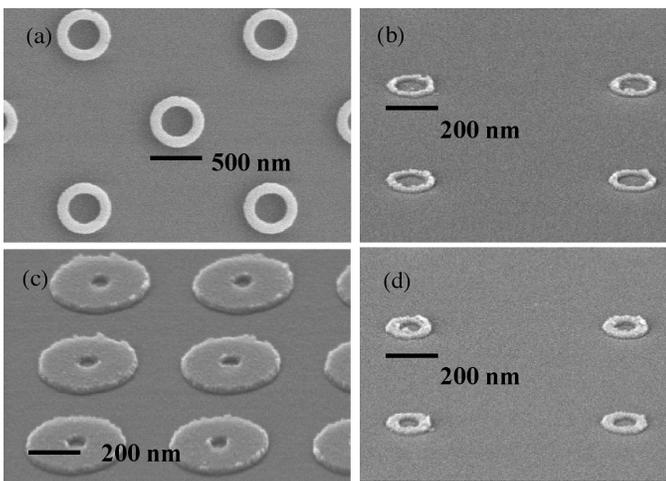
Fig. 24: Plan-view and tilted scanning-electron micrographs of four arrays of Co rings with diameters and linewidths of (a) 520 nm and 120 nm, (b) 190 nm and 30 nm, (c) 360 nm and 160 nm, (d) 180 nm and 50 nm.
