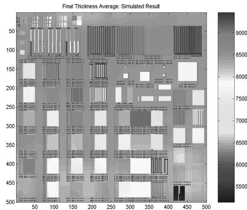
Fig. 4: Final Thickness Average: Simulation Result
