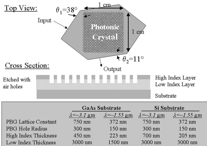
Fig. 49: Superprism device design showing top and side views of the device.
