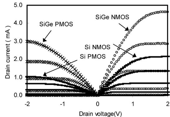
Fig.13: Drain current versus drain voltage as a function of gate drive of SiGe NMOS and PMOS transistors along with Si control device (Gate length =20μm, gate width= 213μm, and 3.8 nm-thick gate oxide). Gate overdrive starts from  $V_g - V_t = 0V$ , to  $|V_g - V_t| = 2V$ , with 0.5V step. SiGe PMOS and NMOS shows about 2.5 and 2.0 times current enhancement respectively owing to increased mobility.
