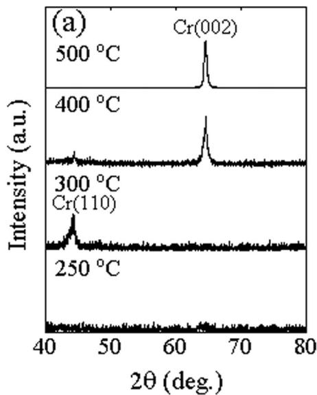
Fig. 19: Cr grown on Si by PLD. As the substrate temperature increases, the texture of the Cr changes from (110) to (200). A similar effect is seen in sputtered Cr films used in hard disks.
