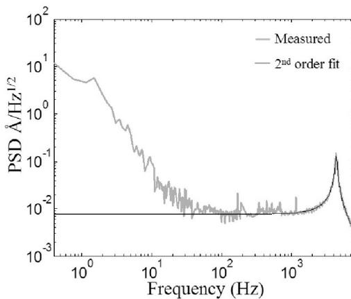
Fig. 18: Power Spectrum Density (PSD) of the differential cantilever deflection.
