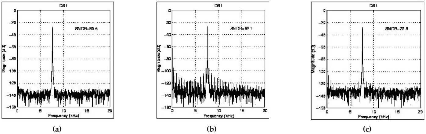
Fig. 30: Delta-sigma converter outputs with a 7.6kHz input signal. (a) Substrate noise generator off, substrate noise shaping loop off. (b) Substrate noise generator on, substrate noise shaping loop off. (c) Substrate noise generator on, substrate noise shaping loop on.
