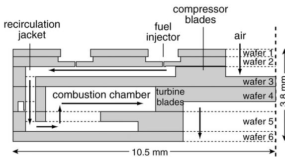
Fig. 34: Schematic of six-wafer combustion system.
