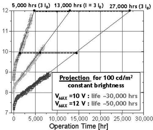
Fig. 21: Driving circuit voltage increase the proposed display driving scheme that compensates for the aging of an OLED.
