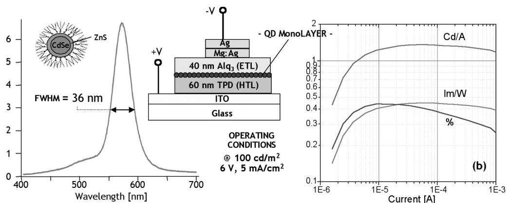
Fig. 32: Hybrid organic/inorganic light emitting device contain inorganic QDs. (Inset) QD-LED cross section. (left) Electroluminescence spectrum at  $\sim 100$  cd/m<sup>2</sup>, with inset device cross section. (right) QD-LED quantum efficiency in percent units, and luminescence efficiency in units of Cd/A and lm/W.
