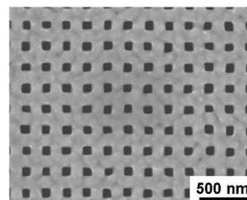
Fig. 14: Anodized alumina template on a Si wafer containing ordered nano-pores. (Pore spacing = 200nm, Pore diameter = 80nm)
