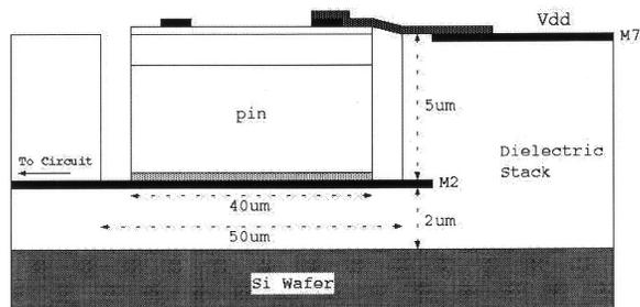
Fig. 30: Cross-sectional drawing illustrating a InP-InGaAs PiN photodiode ABP integrated on a CMOS integrated circuit chip for use in optical clock distribution studies.
