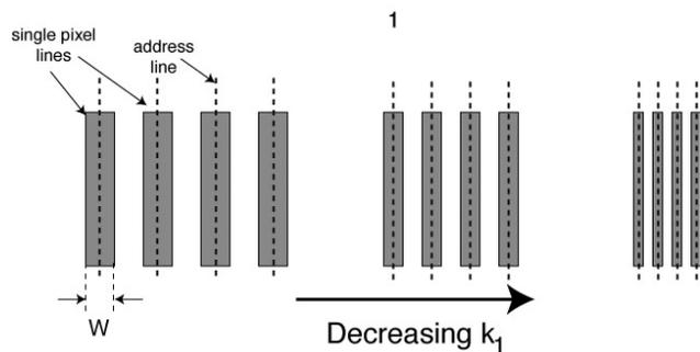
Fig. 16:  $k_1$  in ZPAL. Decreasing  $k_1$  decreases the minimum feature size. This is done by decreasing the address grid of the system, i.e., the scan lines of the focused spot are brought closer together as shown. At some point, the final image will not have sufficient contrast to be resolved by the photoresist. That point determines the limiting  $k_1$  factor.
