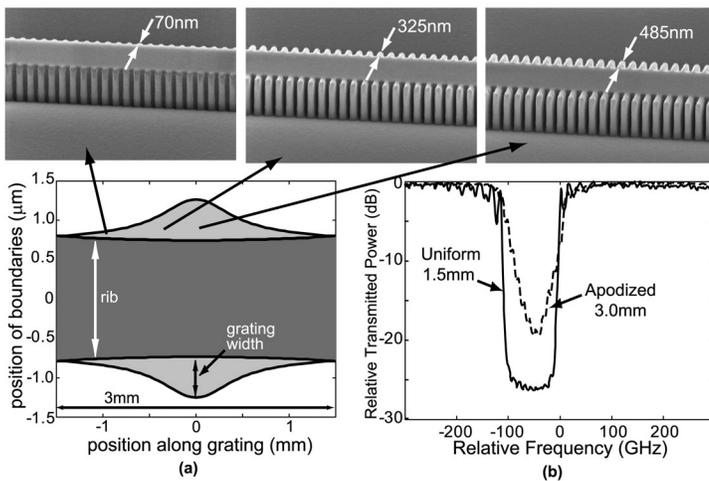
Fig. 43: (a) Apodized Bragg gratings fabricated in the side-walls of a SOI ridge waveguide. (b) Transmission spectra for the TE- mode of uniform and apodized waveguide-grating devices. The reduction of side-lobe levels for the apodized devices is readily apparent.
