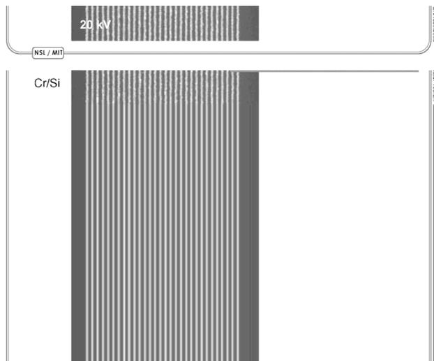
Fig. 3: Scanning electron micrograph illustrating the resolution of the Raith 150 SEBL system.
