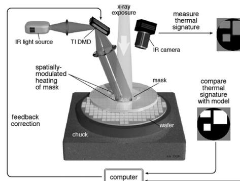
Fig. 26: Proposed implementation of Adaptive-Membrane-Mask Distortion Correction
