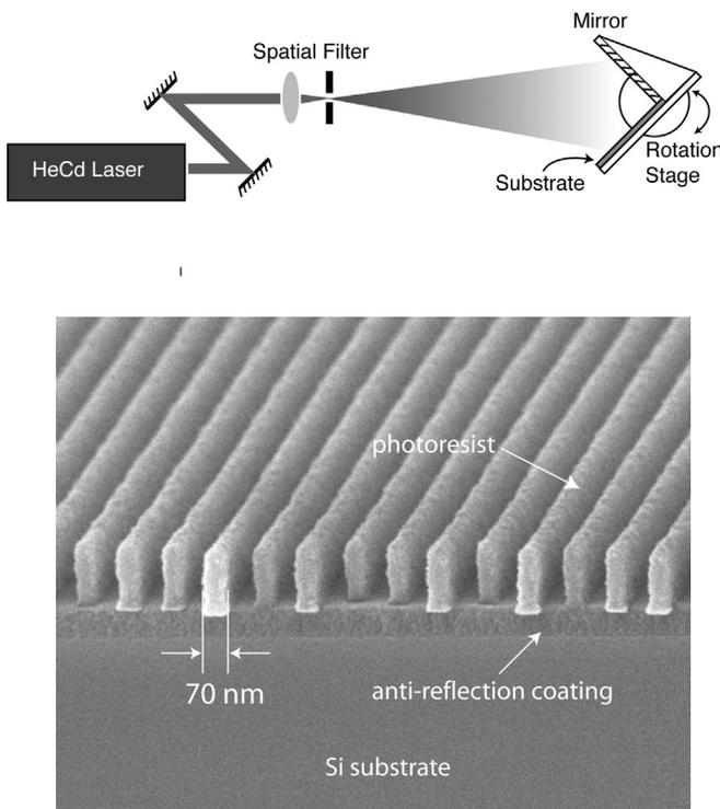
Fig. 29: Schematic of a Lloyds-mirror interferometer. The substrate and mirror are fixed at a  $90^\circ$  angle to one another, and centered in a single incident beam. Rotating the substrate/mirror assembly about its center point varies the spatial-period of the exposed grating. The micrograph shows a grating with 70 nm lines on a 170 nm pitch exposed using the Lloyds-mirror.
