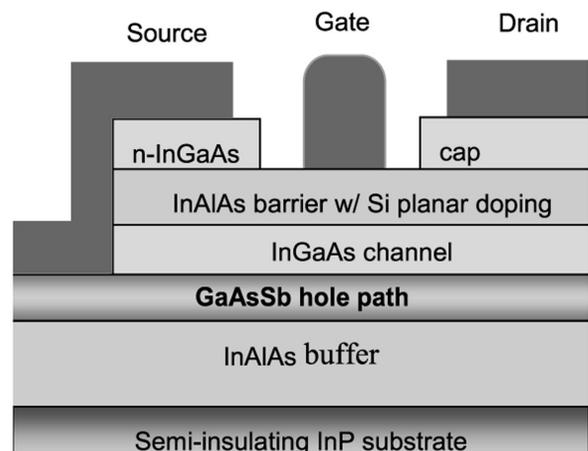
Fig. 18: Cross sectional view of InP-HEMT with hole collector.
