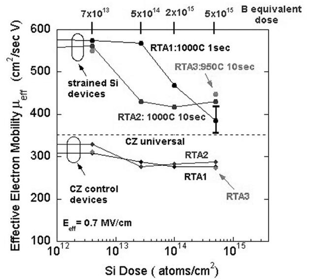
Fig. 9: The effective mobility  $\mu_{eff}$  at  $E_{eff} = 0.7$  MV/cm for strained Si and CZ control devices vs. Si implant dose with different RTAs. The equivalent B doses (in terms of damage profiles) are shown above in blue.
