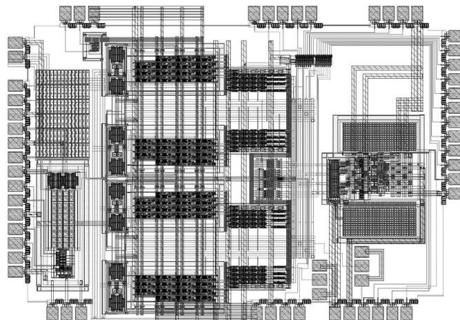
Fig. 12 : Layout of Analog front-end for base-band UWB
