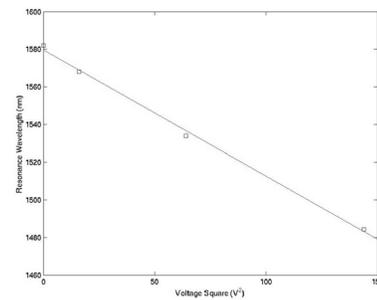
Fig. 7 The resonance wavelength shift with voltage square at 1.582 $\mu\text{m}$ .
