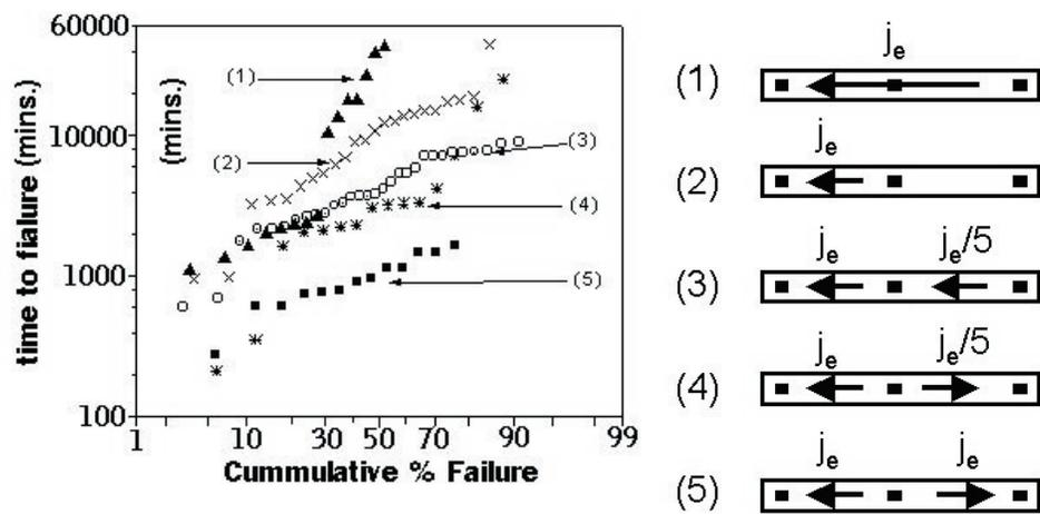
Fig. 25: Failure times (right) for 3-terminal Cu interconnects tested under different current configurations (left).
