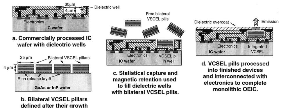
Fig. 32: The MASA process: (a) the processed IC wafer with the recesses prepared, and (b) the p-side down VCSEL wafer with pillars etched in a close-packed array; (c) statistical assembly of the freed nanopills in the recesses on the IC wafer; and (d) after completing device processing and integration.
