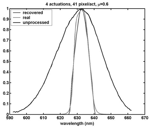
Fig. 4: Spectrum recovered using ICIOD VS real spectrum of an interference filter.
