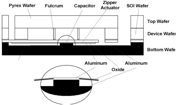
Fig. 40: 2-D schematic of the design of a tunable capacitor.
