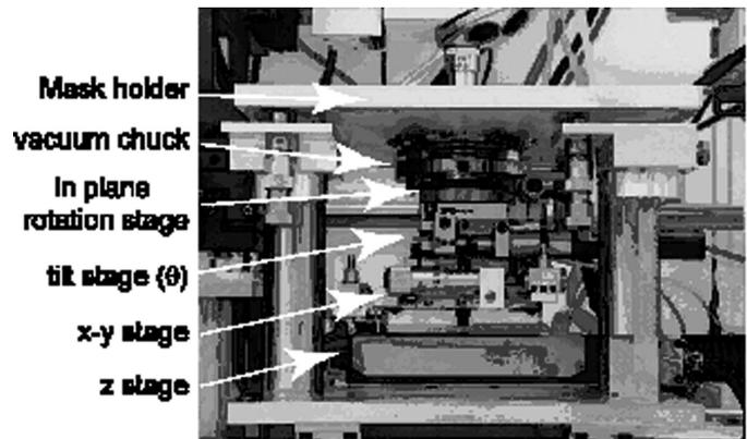
Fig. 26: Photograph of the stage for tilted X-ray exposure. The X-ray source, which is not shown, is above the mask holder.
