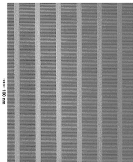
Fig. 59: Scanning electron micrograph of a free-standing 100 nm-period grating (50 nm-wide bars) in a silicon nitride membrane of area 500 microns by 5 mm.
