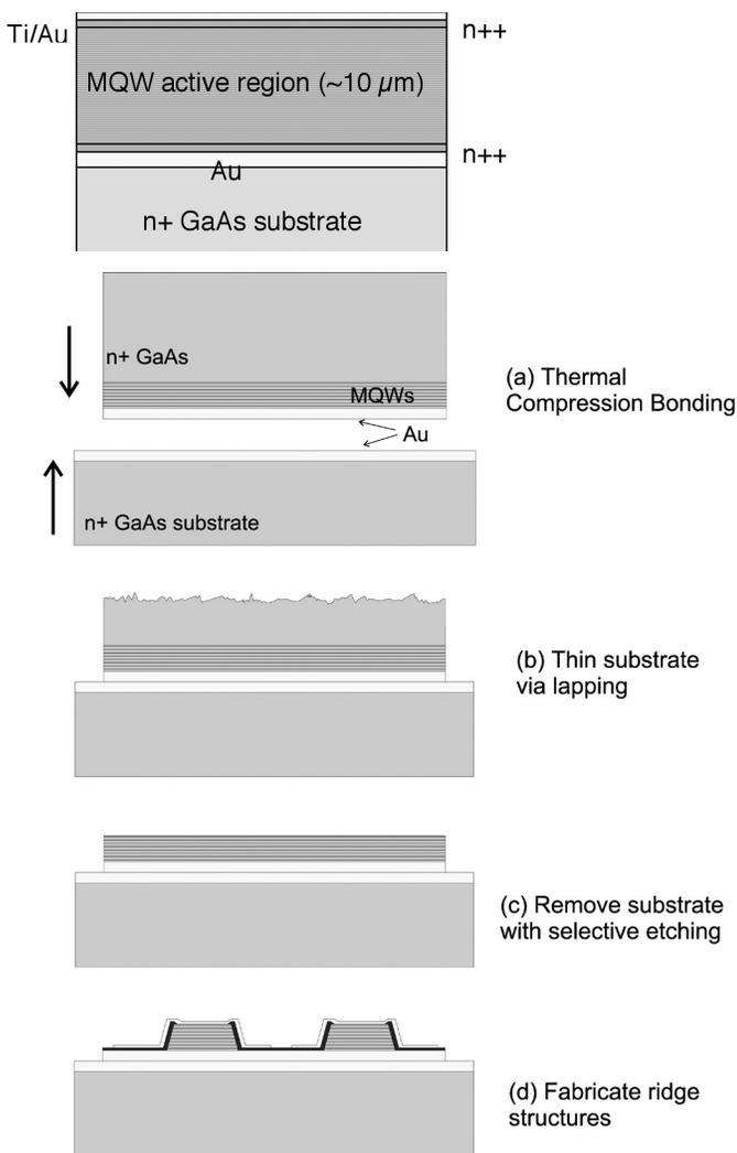
Fig. 44: Top: Side view of a metal waveguide structure for THz mode confinement. Right: Fabrication process of the metal waveguide structures.
