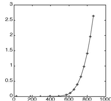
Fig. 36: Photocell power output and system efficiency, as a function of temperature, during electrical heating of the SμRE.
