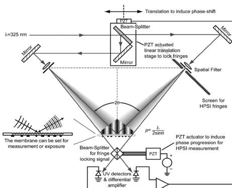
Fig. 25: Schematic of the Holographic-Phase-Shifting Interferometer (HPSI). This setup can be used as an interference lithography system to write reference grids as well as a holographic interferometer to measure grid distortion.
