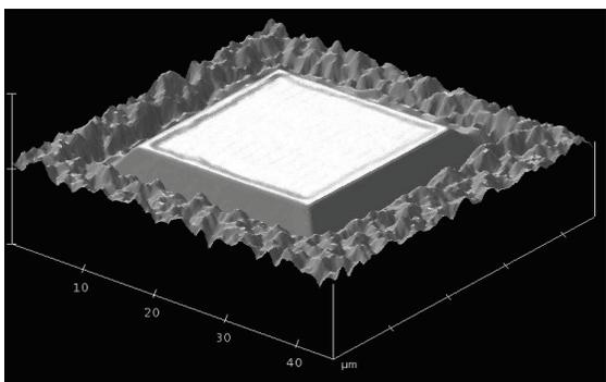
Fig. 9: AFM image of a selectively grown Ge mesa.
