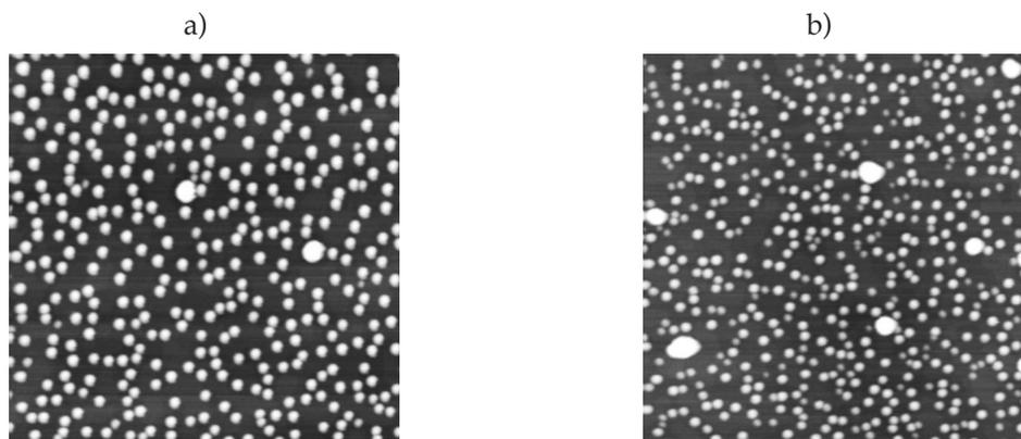
Fig. 48: Atomic force micrographs of  $1 \mu\text{m} \times 1 \mu\text{m}$  square areas. a) With the arsine flow = 0.1 sccm, the density of InAs quantum dots is  $4 \times 10^{10} \text{ cm}^{-2}$  and the average diameter is 23 nm. b) With the arsine flow = 1.0 sccm, the density of InAs quantum dots is  $6 \times 10^{10} \text{ cm}^{-2}$  and the average diameter is 21 nm.
