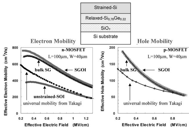
Fig. 17: Partially depleted surface strained-Si *n*- and *p*-type MOSFETs on relaxed SGOI substrates show enhanced electron and hole mobilities comparable to those measured on bulk SiGe virtual substrates (bulk SG).
