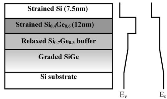
Fig. 12: Schematic CMOS layer structure and band alignment for this proposal. The buried compressively strained-Si<sub>0.4</sub>Ge<sub>0.6</sub> channel is channel for holes while the surface strained-Si is channel for electrons.
