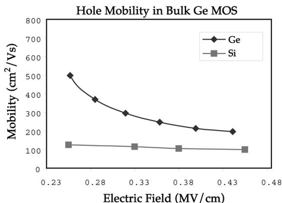
Fig. 6: Comparison of hole mobility in Ge and Si PMOSFETs. The germanium devices show a factor of two enhancement in mobility.
