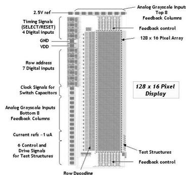
Fig. 20: 28 x 16 pixel integrated circuit layout.
