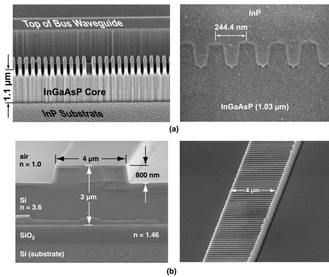
Fig. 42: Examples of the dual-hardmask process applied to two different materials systems. (a) Scanning-electron micrograph depicting a quarter-wave-shifted, 244.4 nm period Bragg grating etched into the top surface of an InGaAsP waveguide, and the subsequent InP overgrowth. (b) Silicon-on-insulator (SOI) ridge waveguide cross-section and SOI waveguide with Bragg grating in the top.
