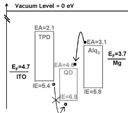
Fig. 19: Proposed energy level diagram of device in Fig. 18. Values for ionization energy (IE) of all materials except QDs are taken from photoemission spectroscopy measurements<sup>1</sup>. Electron affinity levels (EA) were then calculated using optical absorption data. QD levels shown are from calculated values
