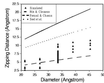
Fig. 13: Comparison of zipping height versus island size based on MD simulations, finite element simulations, and models of Nix and Clemens and Freund and Chason.
