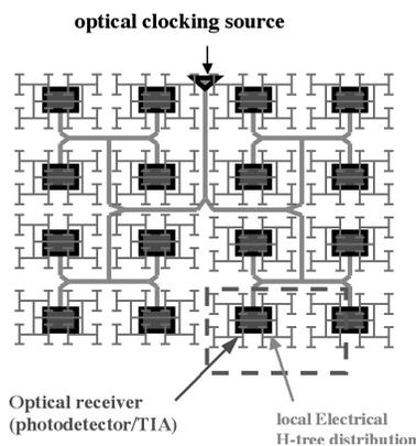
Fig. 1: Schematic of optical clocking and H-tree waveguide structure
