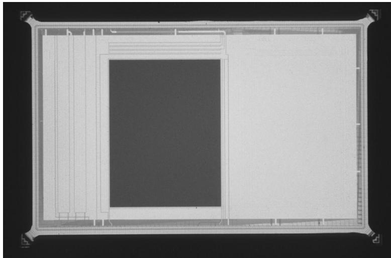
Fig. 26: Die photo of programmable wide dynamic range CMOS image.
