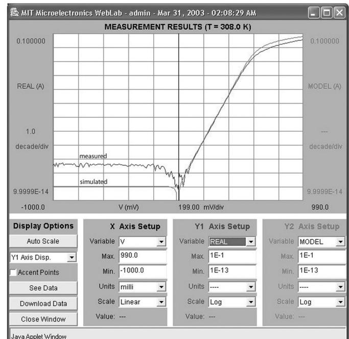
Fig. 1: Measured and simulated response of a pn junction to an applied voltage, plotted in the WebLab client applet.
