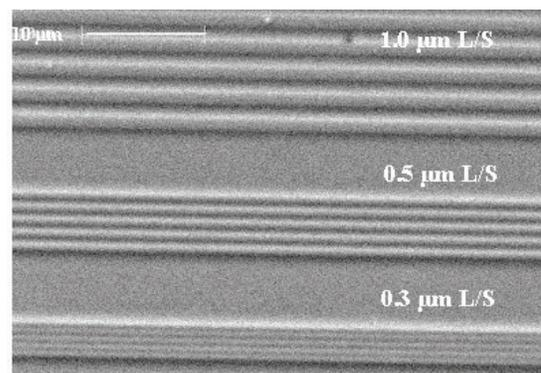
Fig. 6: Solventless lithography using a dry resist developed by supercritical  $\text{CO}_2$  after e-beam exposure, demonstrating 0.5  $\mu\text{m}$  and 0.3  $\mu\text{m}$  line/spaces pattern in the vapor deposited copolymer of GMA and FAA.
