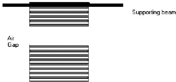
Fig. 29: The illustration of the one dimensional photonic crystal with large air defect.
