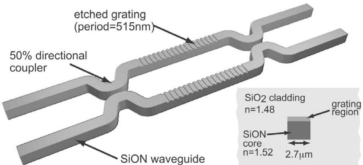
Fig. 16: Wavelength-Division-Multiplexing (WDM) channel add/drop filter currently being fabricated in silicon-oxynitride, and a cross-section of the waveguide/grating region (lower right). A number of WDM channels enter the device on the input port, a single channel is routed to the drop port while the remaining channels pass to the through port. The dropped channel can be replaced with an input on the add port.
