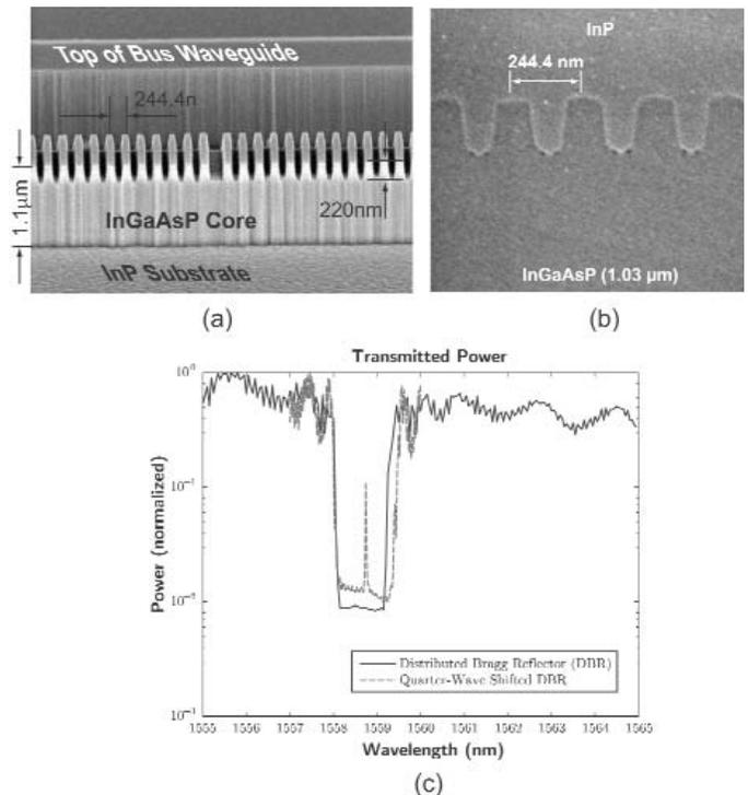
Fig. 15: (a) Scanning electron micrograph depicting a quarter wave shifted 244.4 nm period Bragg grating etched into the top surface of an InGaAsP waveguide. (b) Device grating after InP epitaxial overgrowth at Lucent Technologies. (c) Transmission spectra for uniform and quarter-wave-shifted distributed-Bragg-reflectors.
