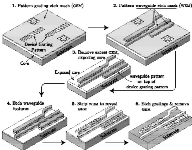
Fig. 14: Dual-layer hardmask process used to pattern fine-period Bragg gratings atop relatively tall waveguide structures. The process is designed such that all lithography steps are performed over essentially planar topography.
