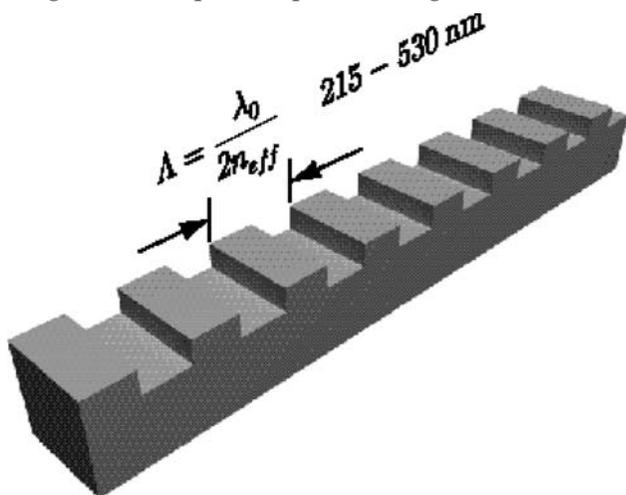
Fig. 13: Schematic of an integrated Bragg grating. A shallow corrugation is etched into the top surface of a waveguide. The Bragg grating period,  $L$ , ranges from 215 nm to 540 nm, depending on the material and waveguide design.
